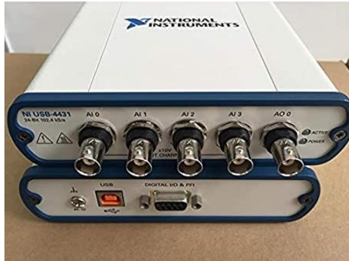
Figure 22 data acquisition system used in the experiments
