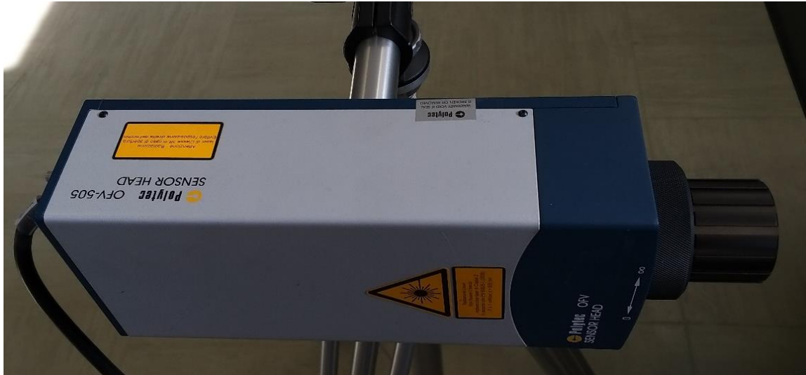
Figure 18 Laser vibration sensor used in the experiments
