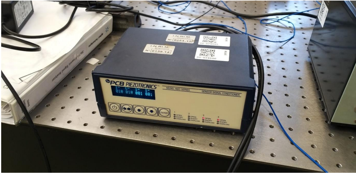
Figure 21 signal conditioner used in the experiments
