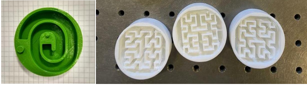
Figure 4 Acoustic metamaterials analysed in the thesis paper of Tomosso Pandolfi conducted in the INRiM research centre [5]
