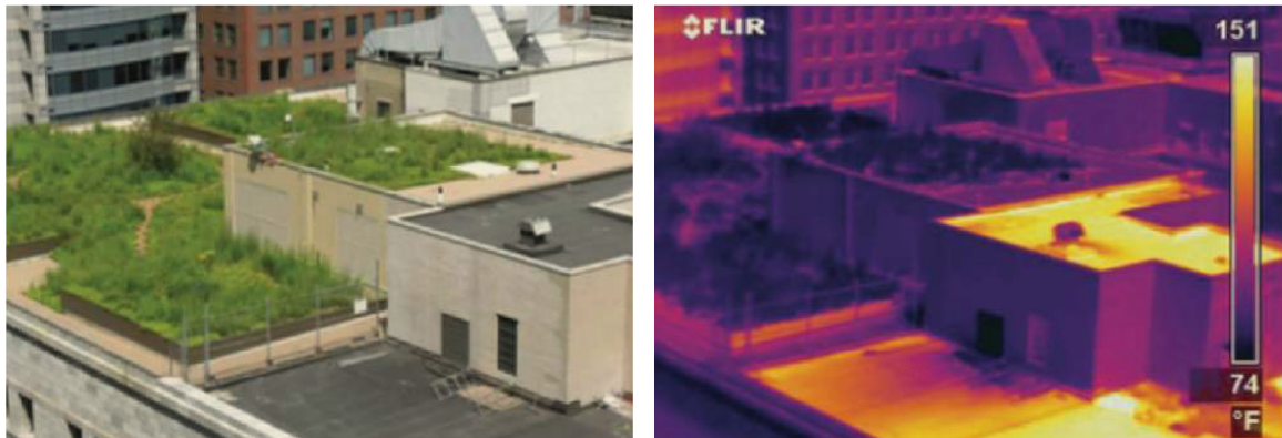
Figure 38 Temperature Differences Between A Green And Conventional Roof [21]
