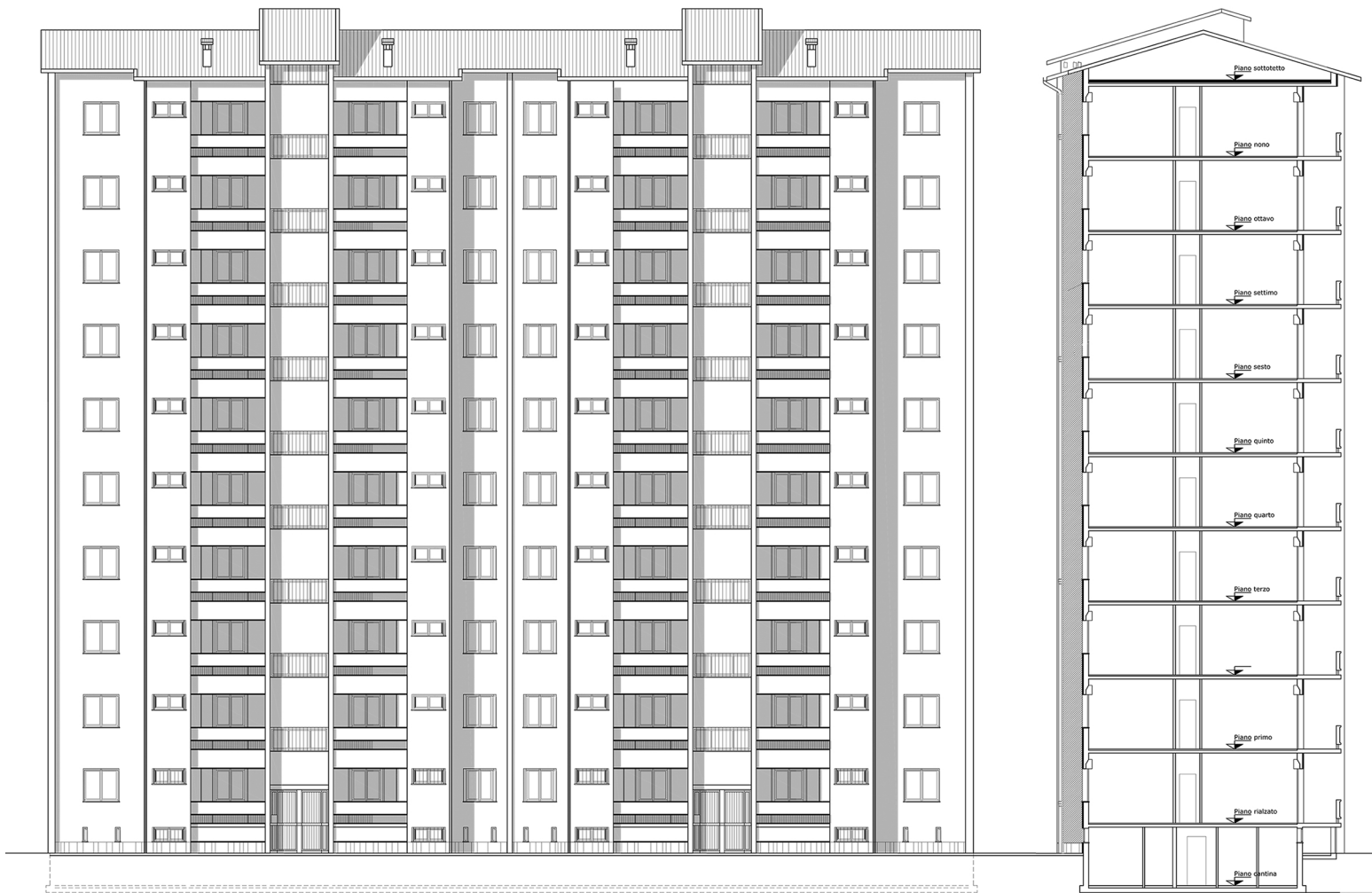
Figure 125 Front View and Section A-A of Building Type B (Reference Building)
