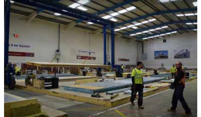
fig 5.2.20 Timber frame slabs assembled and lifted
