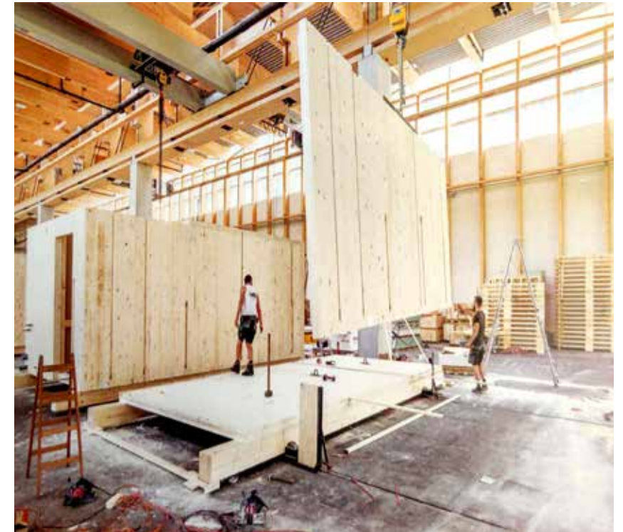
fig 3.5.4 Manufacturing Hall at Kaufmann Zimmerei und Tischlerei in Dornbirn(AT), Architect Johannes Kaufmann Architektur, Room module shell structures made of CLT.
