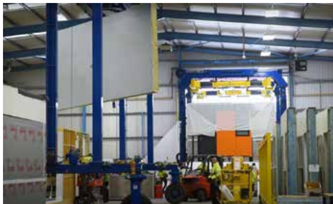
fig 5.2.25 Module lifted with crane
