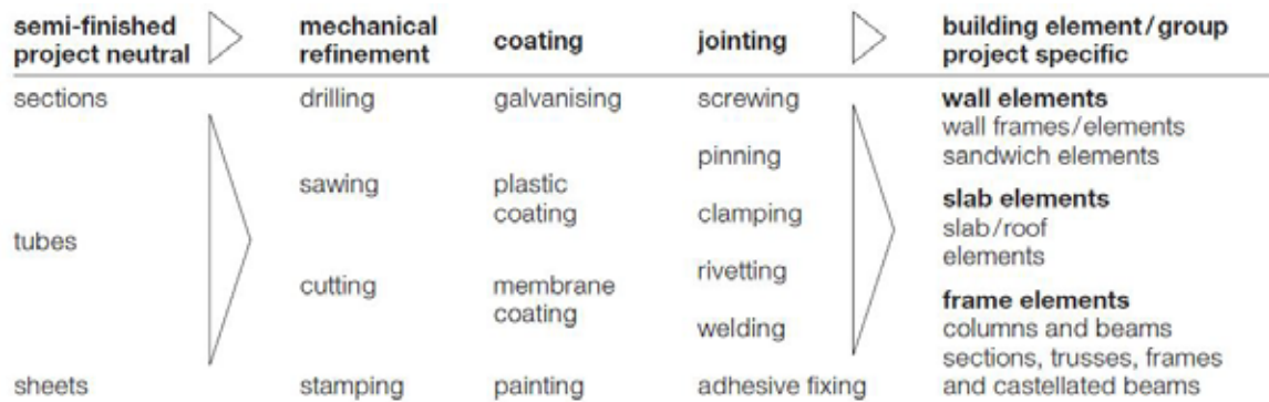
fig 4.2.1 Manufacturing process of elements at factory
