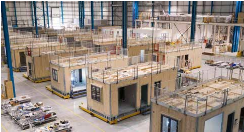
fig 3.1.2 Offsite module construction and assembly with interior fittings. Source - APRAO - Modular Construction
