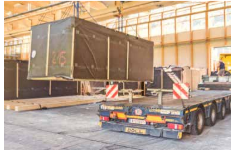
fig 3.5.14 Hotel Nordlingen 2018 Ar. Johannes Kaufmann Loading of room modules onto the articulated truck in manufacturing hall.
