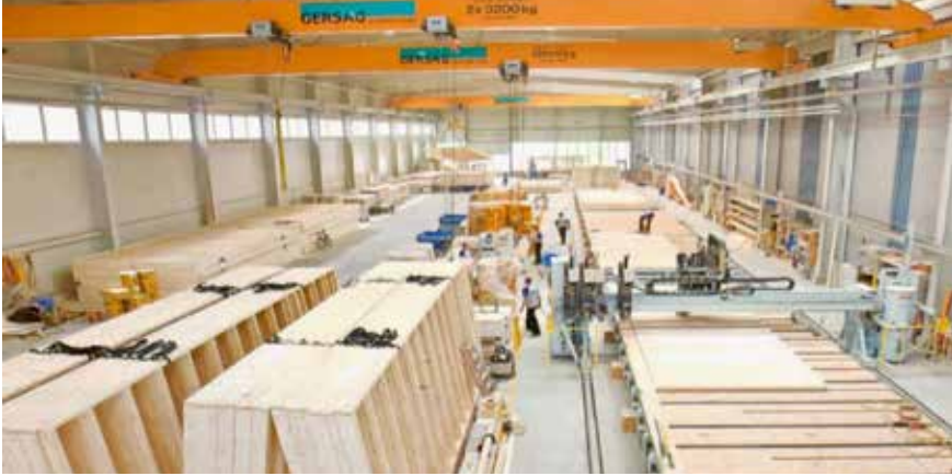
fig 3.5.1 Timber construction and manufacturing hall at Erne. - Manufacture of timber frame elements as shell structure by means of a rail system and indoor crane.
