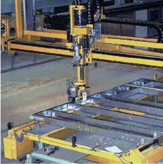
fig 4.5.1 Manufacture of a steel frame in a factory
