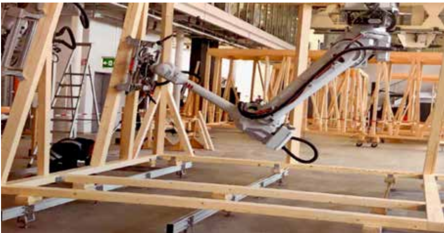
fig 3.5.3 Manufacture of complex room modules as timber frame structures using a gantry robot. Research project by Erne in collaboration with ETH Zurich.
