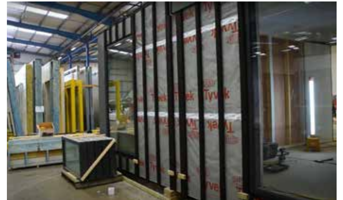
fig 5.2.23 Modules packed with waterproof membrane
