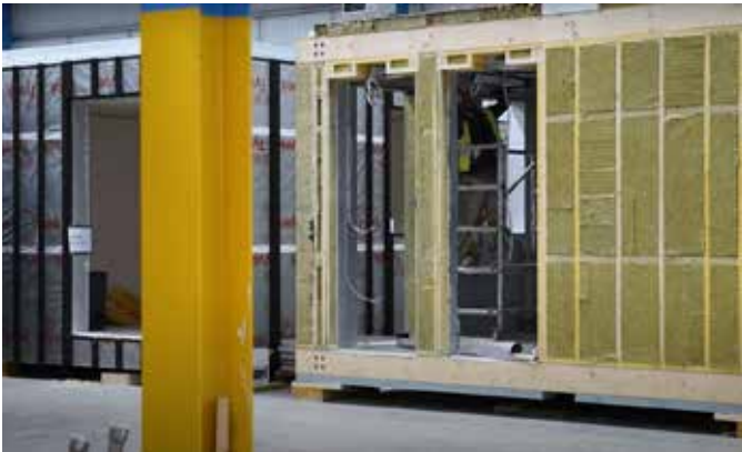
fig 5.2.21 Adding insulation and fittings to the module
