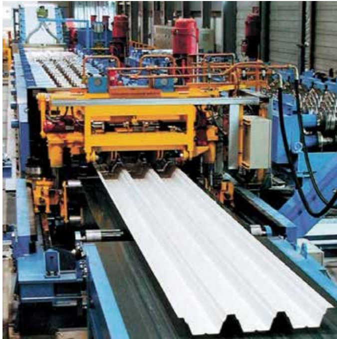
fig 4.5.7 Manufacture of trapezoidal steel sheeting
