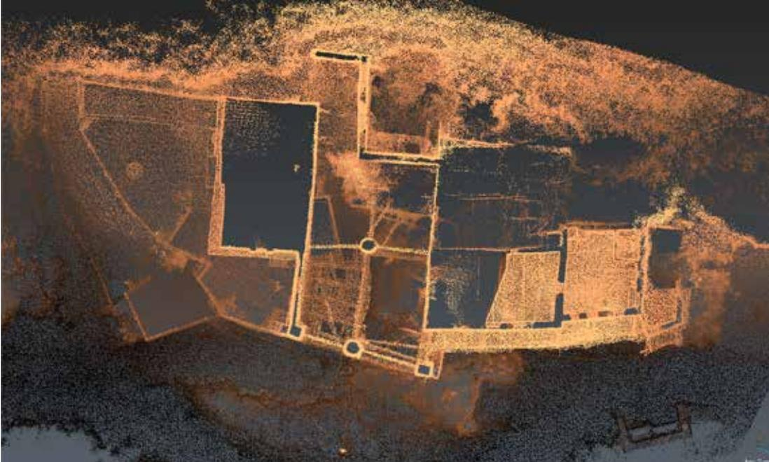
Fig.3.85 - View of the cloud from Zeb Revo RT showing interior profiles and wall thickness.
