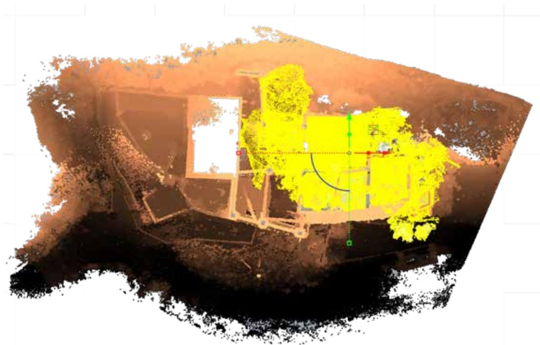
Fig.3.53- Image of top view, alignment of the Zeb cloud and the 3D scanner application cloud
