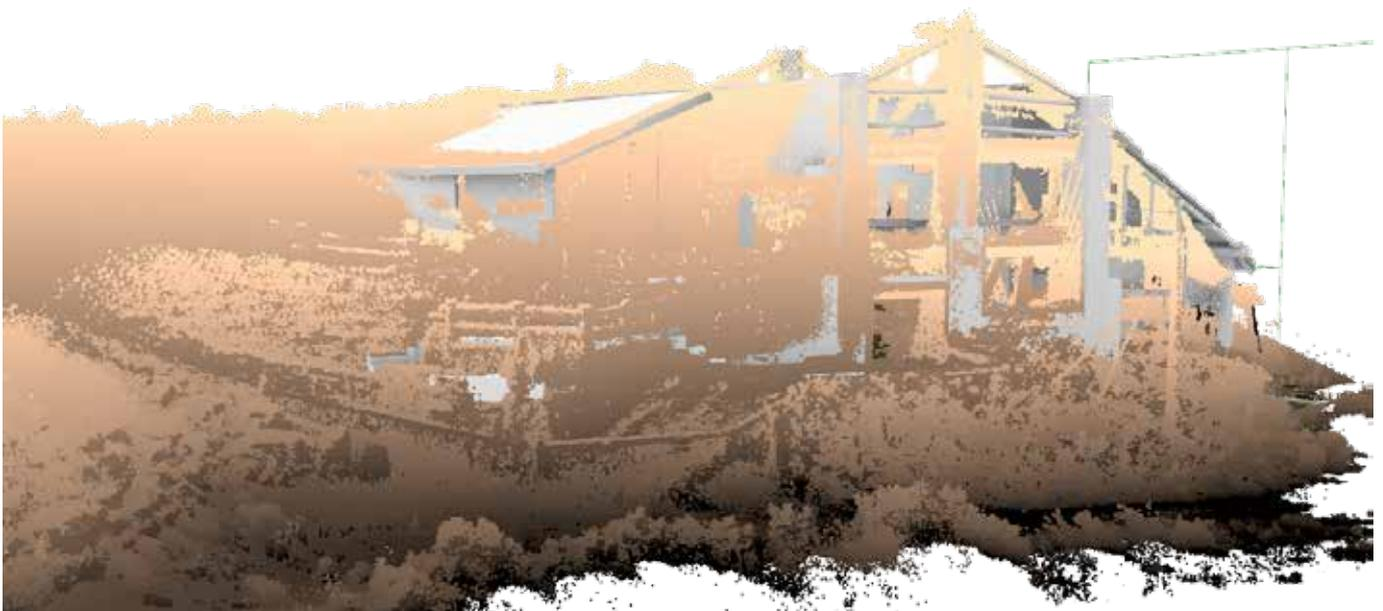
Fig.3.58- Image showing the overlap of the Rhinoceros 3D model and the Zeb cloud.
