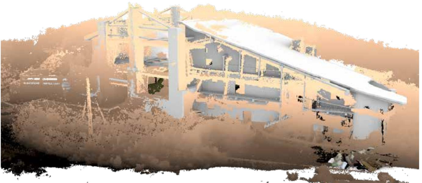
Fig.3.57- Image showing the overlap of the Rhinoceros 3D model and the Zeb cloud.
