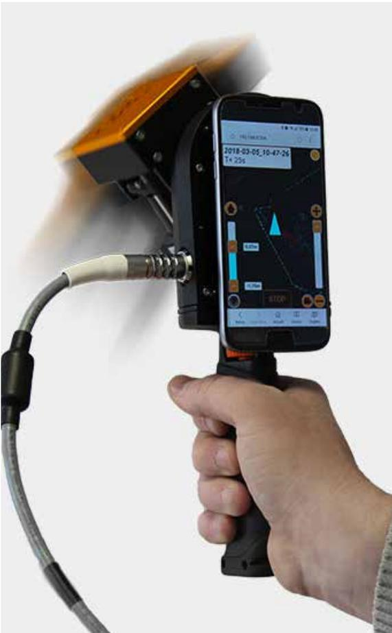
Fig.1.19- Image of Zeb Revo RT instrument, when being used.
