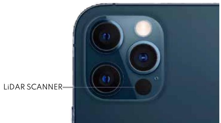
Fig.3.37- Image of the LiDAR scanner inbuilt inside the I-phone device
