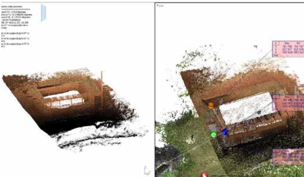
Fig.3.78 - Alignment through points, using 6 points keeping the LiDAR cloud as a fixed reference.
