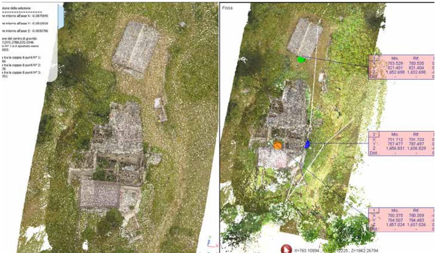
Fig.3.61- Alignment through points, using 3 points keeping the Flight cloud as a fixed reference.
