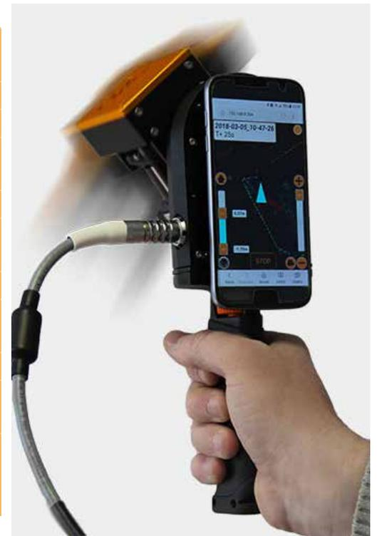
Fig.3.24- Image showing Functioning of the instrument Zeb Revo Rt.
