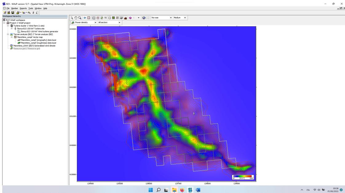
**Figure 2.6:** User interface of the software WAsP, for wind turbine site sizing
