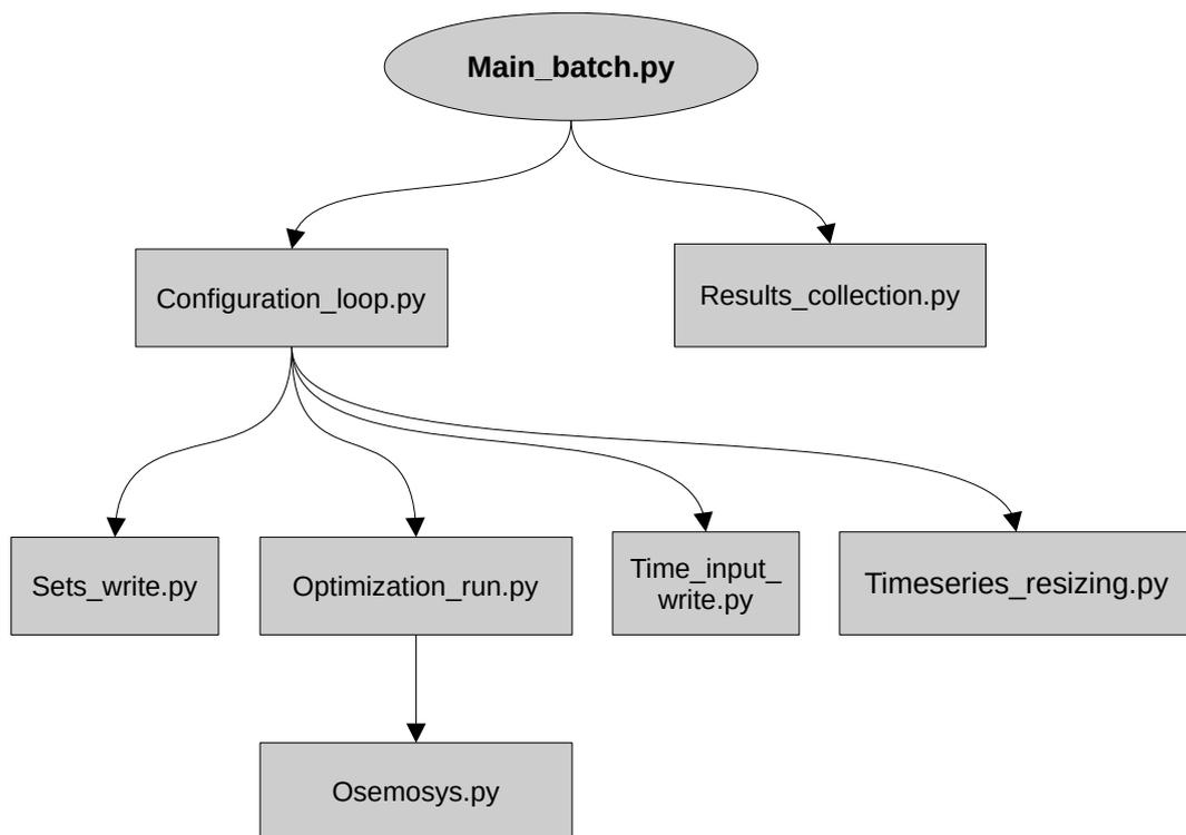
**Figure 4.4:** Structure of the developed code.
