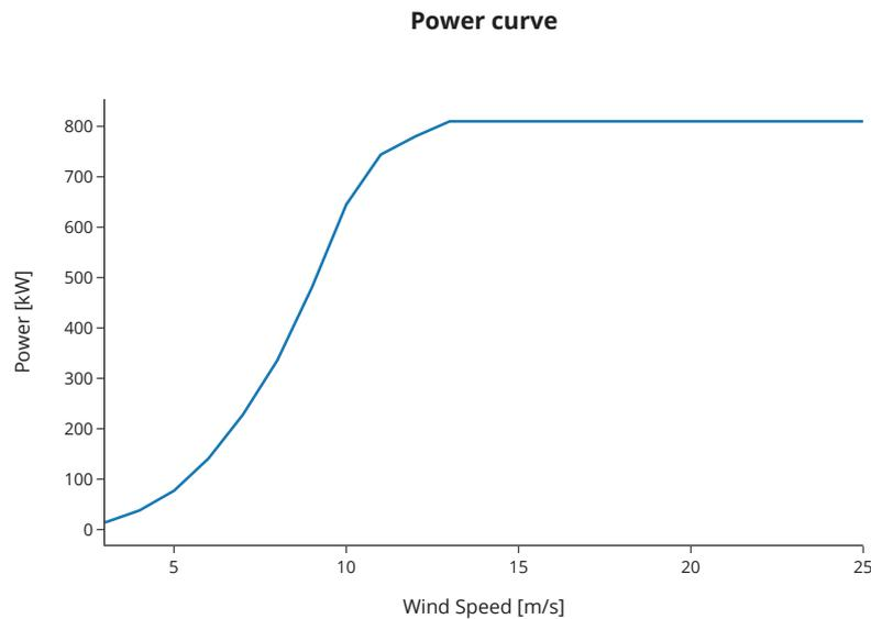
**Figure 3.5:** Enercon E53 power curve [23]
