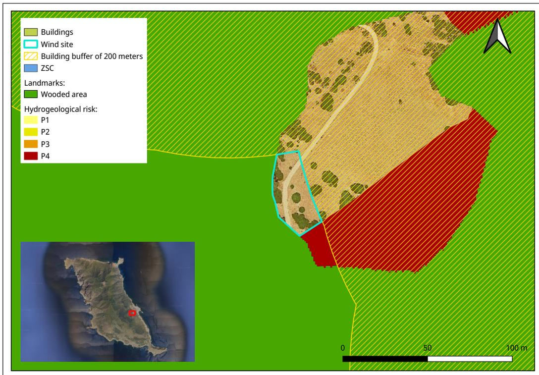
**Figure 2.28:** Suitable site for the installation of wind turbines on the island of Marettimo
