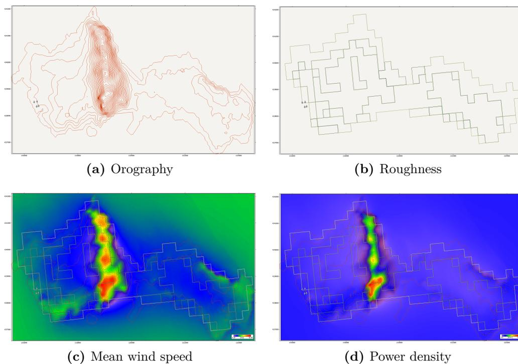
**Figure 2.14:** Most important wind-related characteristics of Favignana. To be noticed, the highest values of wind speed and power density are on the top of the hill.
