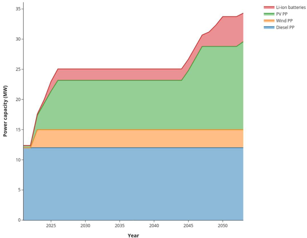
**Figure 5.4:** Power capacity in Favignana when the demand is constant and the CO<sub>2</sub> emissions target is zero. The constant slope between 2027 and 2045 means that the CO<sub>2</sub> target requirements are satisfied. The solver, in fact, installs enough renewables power plant at the beginning of the simulation probably because it would reduce the overall costs.
