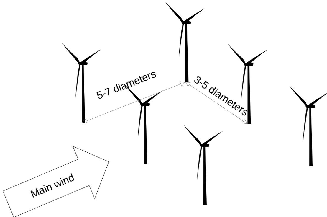
**Figure 2.8:** Distancing between the turbines in the same site [28].
