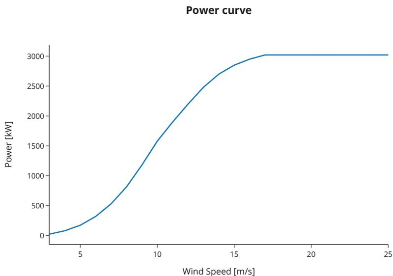
**Figure 3.6:** Enercon E82 power curve [24]
