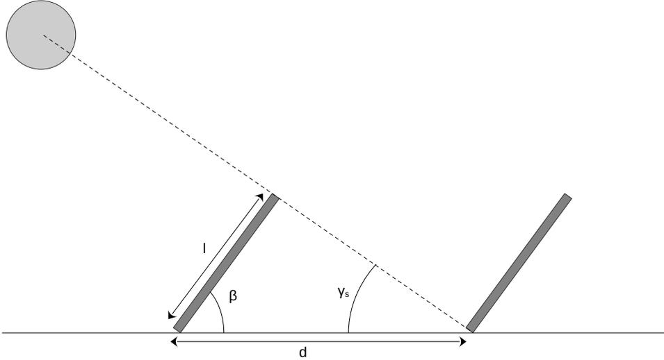
**Figure 2.11:** Spacing of the ground panels
