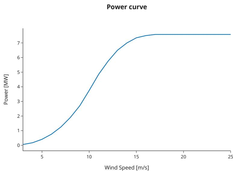
**Figure 3.4:** Enercon E126 power curve [22]
