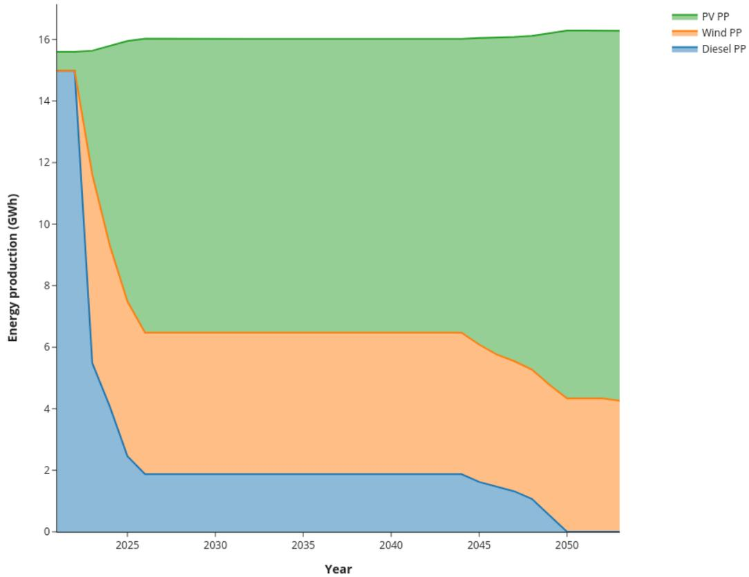
**Figure 5.5:** Energy production in Favignana when the demand is constant and the CO<sub>2</sub> emissions target is zero. As it is possible to see, there is a little increment in the generated power. This could be associated to the installation of the storage in the system. The storages, in fact, have energy losses in both the phases of charging and discharging.
