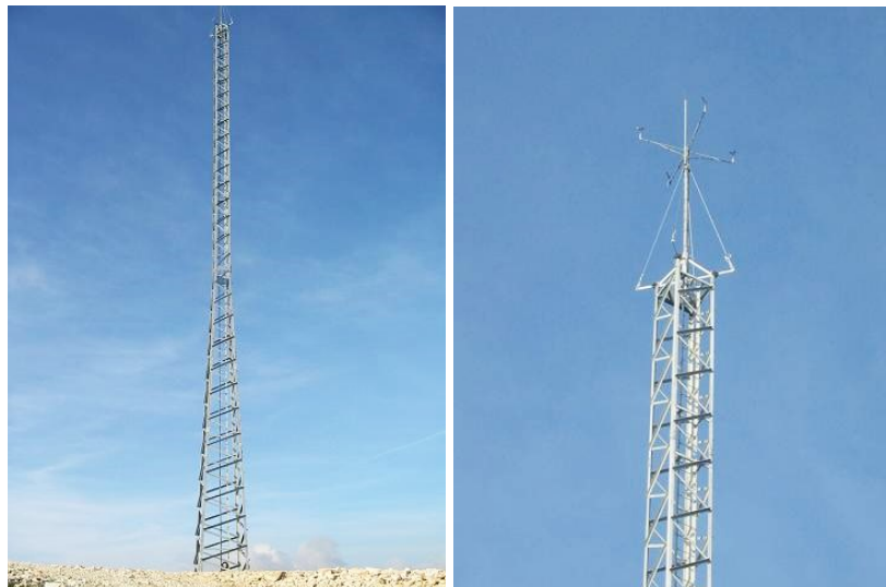
Figure 4.15 – Anemometric tower and wind sensors
