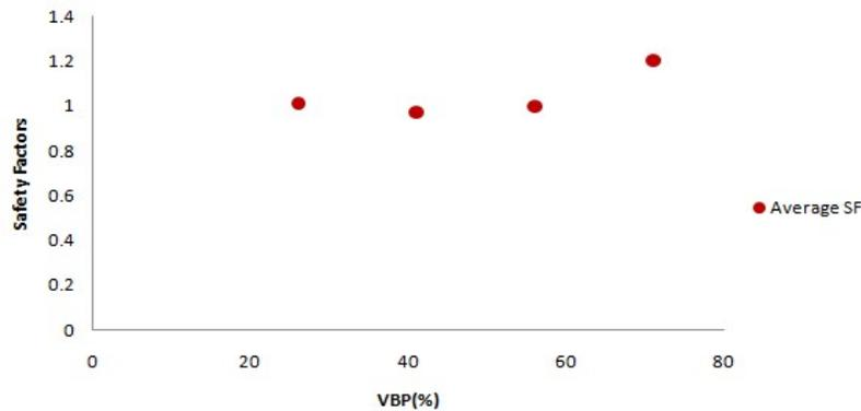
Figure 39 Safety factors with respect to VBP when cohesion of the block- matrix interfaces is reduced by 50%
