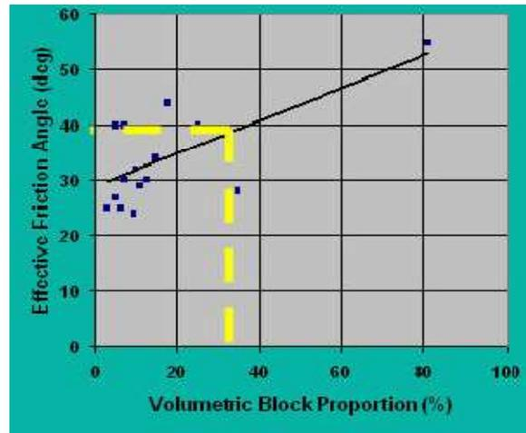
Figure 3 Plot of effective angle of friction as a function of volumetric block proportion, generated from laboratory testing of Franciscan melange specimens obtained from core drilling at Scott Dam, northern California (After Goodman and Ahlgren, 2000)
