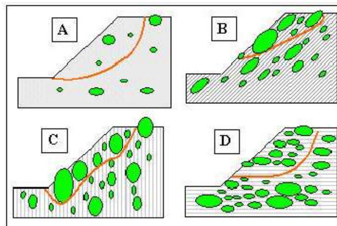
Figure 6 Some possible failure surfaces in bimsoils. A) Low block proportion with critical failure surface unimpeded by blocks. B) Anisotropic bimrock, such as melange, with blocks and shears oriented out of slope, and failure surface guided by the fabric. C) Blocks and shears oriented vertically such that failure surface is
