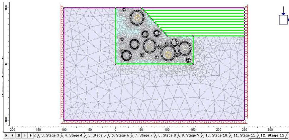
Figure 15 Example of a bimslope model including blocks with interfaces (inRS2)
