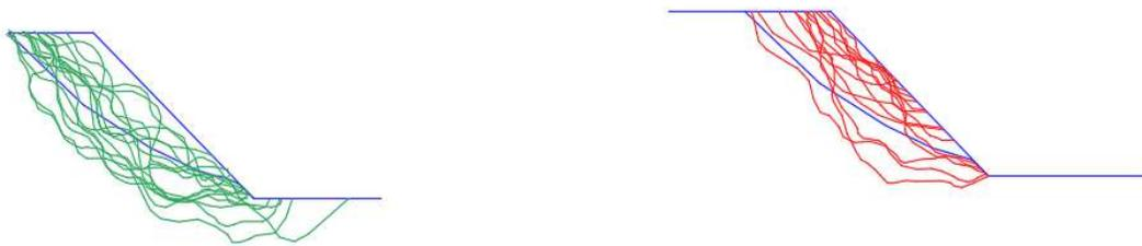
*Figure 46 Comparison of failure surface of bimsoils (green lines) and bimrocks (red lines) (70% VBP when the cohesion and tensile strength of the block-matrix interfaces were reduced by 100%)*
