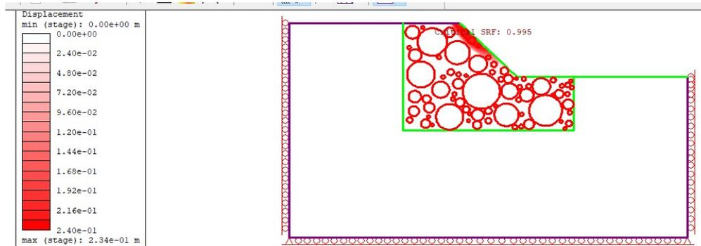
Figure 25 Total displacements of the 55% VBP model when the cohesion is reduced by 50%
