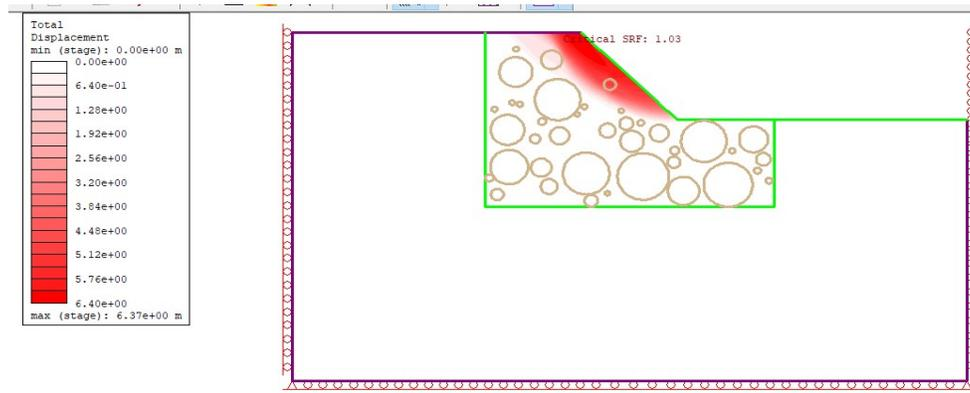
Figure 33 Total displacements in 40% VBP model when cohesion is reduced by 100%
