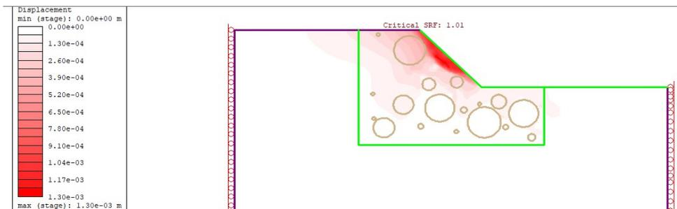
Figure 31 Total displacements in 25% VBP model when cohesion of the block- matrix is reduced by 100%
