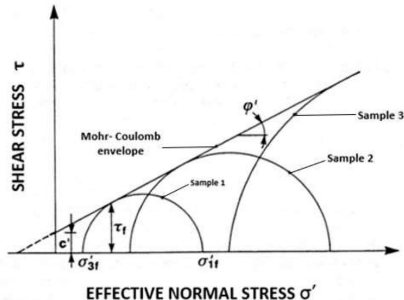
Figure 13 Mohr – Coulomb circles at failure and strength characteristics in effective stresses (AGI, 1994)
