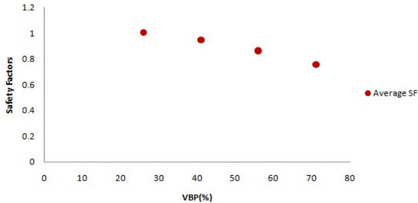
Figure 41 Safety factors with respect to VBP when cohesion is reduced by 100%
