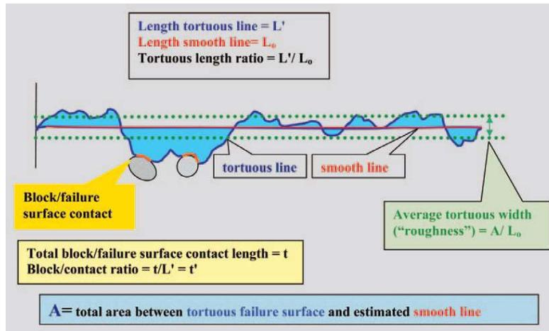
Figure 5 Parameters measured and calculated from traced lines of tortuous failure surfaces. (Medley, 2004)
