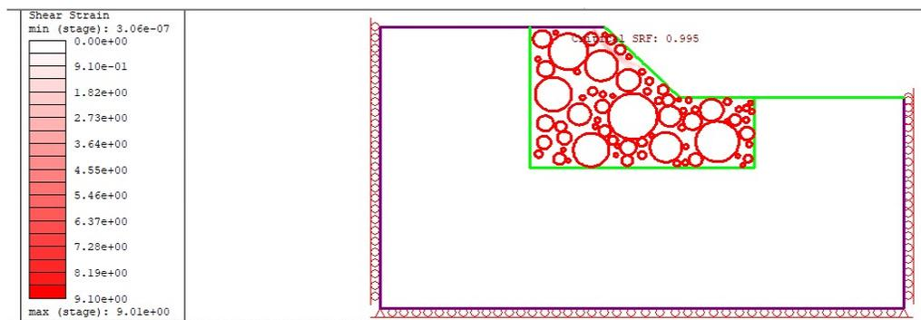
Figure 24 Maximum shear strain of the 55% VBP model when the cohesion of the block interfaces is reduced by 50%.
