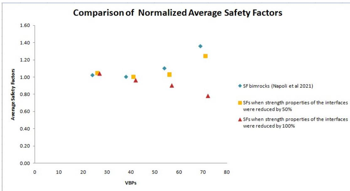
Figure 43 Comparison between the normalized average safety factors of bimrocks and bimsoil models with strength properties of the block- matrix interfaces reduced by 50% and 100% with respect to the properties of the matrix
