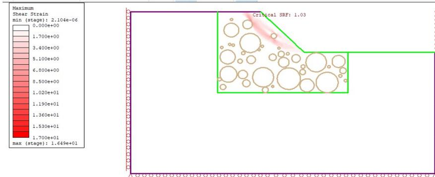
Figure 32 Maximum shear strains of 40% VBP model when the cohesion of the block- matrix interfaces is reduced by 100%.
