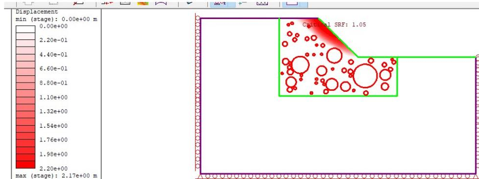
Figure 21 Total displacements in 25% VBP model when cohesion is reduced by 50%
