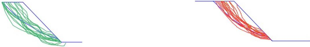
*Figure 45 Comparison of failure surface of bimsoils (green lines) and bimrocks (red lines) (25% VBP when properties of interfaces were reduced by 50%)*
