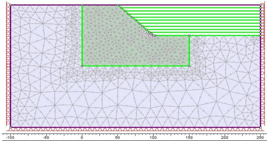
Figure 14 A bimslope model without the blocks (0% VBP) (inRS2)
