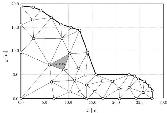
Figure 8 Triangular meshes inside the polygon of the bimslope boundary with each triangle filled with circular blocks of different sizes (Montoya-Araque et al., 2020).
