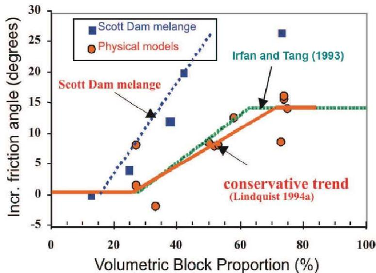
Figure 4 Increment of friction angle with respect to volume proportion of the blocks (after Lindquist, 1994)
