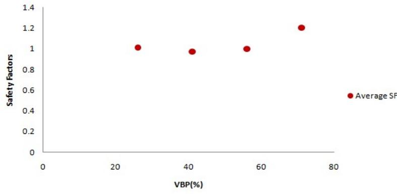
Figure 28 Safety factor with increasing VBPs when cohesion and tensile strength of the block-matrix interfaces were reduced by 50%
