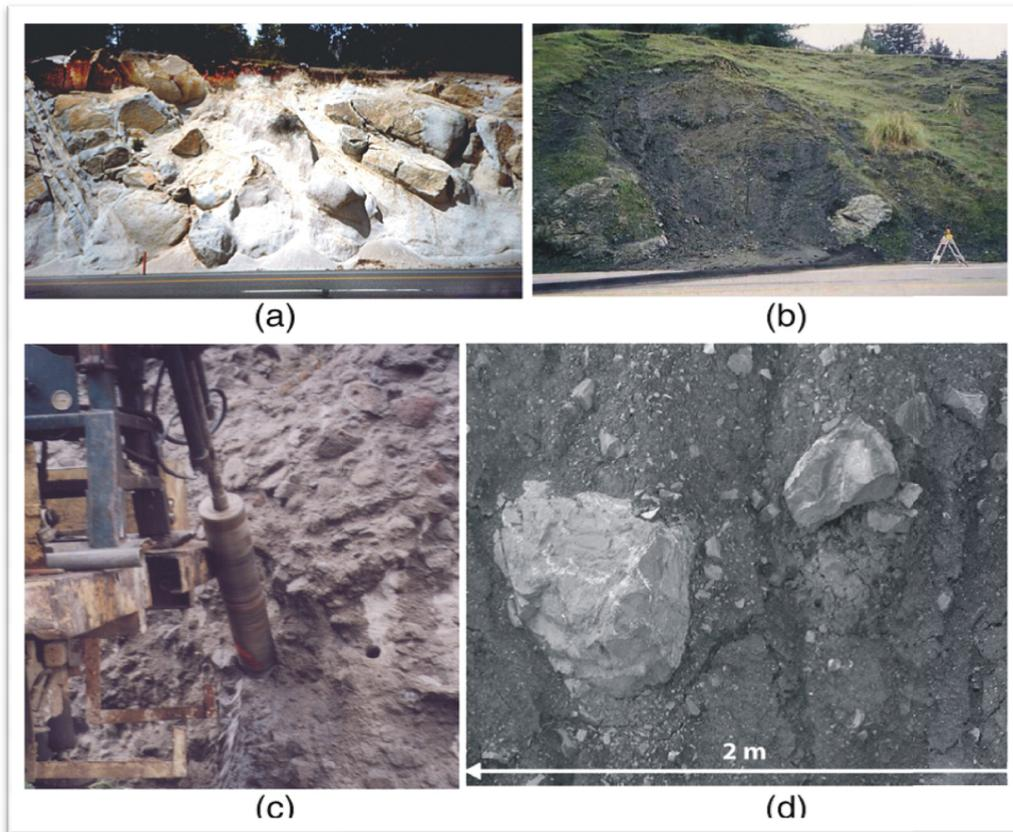
*Figure 1 Some pictures of different kinds of bimrocks, (a) a decomposed granite (weathered rock) bimrock in the Sierra Nevada of California (photo: Dr. E. Medley), (b) Franciscan Complex mélangé, Northern California (photo: Dr. E. Medley), (c) a welded bimrock Ankara agglomerate (photo: Dr. H. Sonmez), (d) a view of mélangé in the Santa Barbara mine of the Northern Appennines (Italy) (from Coli et al., 2011).*
