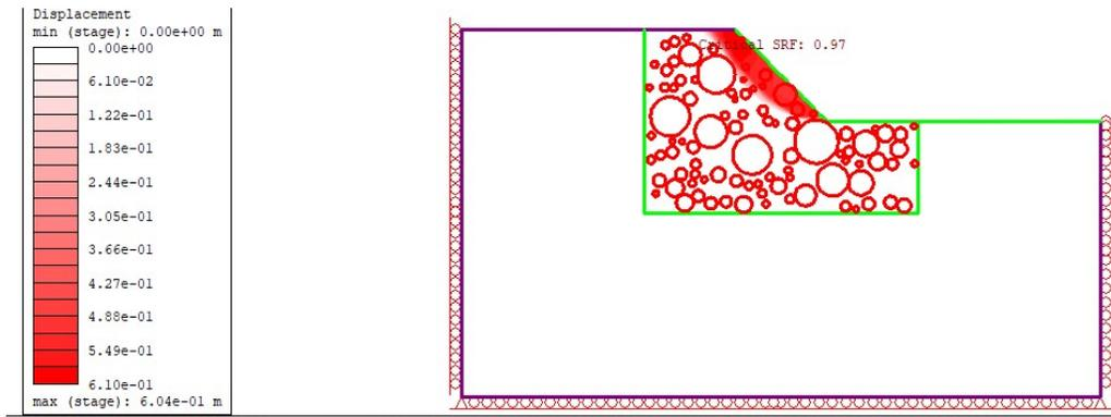
Figure 23 Total displacements of the 40% VBP model when cohesion is reduced by 50%
