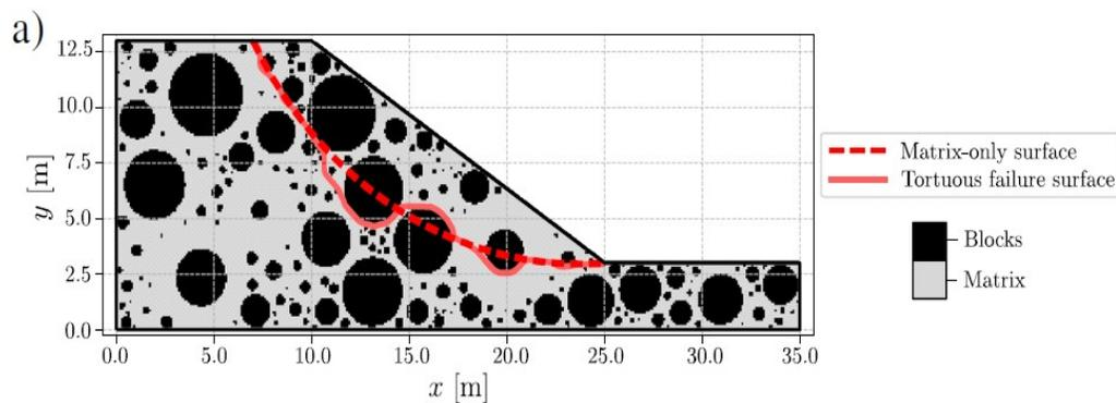
Figure 10 Matrix-only circular failure surface and tortuous failure surface inside a bimslope (Montoya-Araque et al., 2020).
