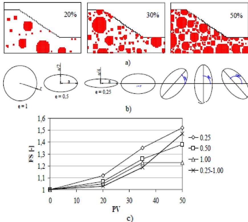
Figure 12 a) Slope models with different VBP b) Shapes and orientations of blocks analysed c) Trend of changing Factor of Safety (Barbero et al., 2006)
