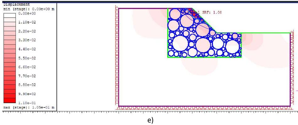
Figure 16 Failure surfaces when the strength parameters of block matrix interface were same as that of the matrix a) 0% VBP b) 25% VBP c) 40% VBP d) 55% VBP e) 70% VBP
