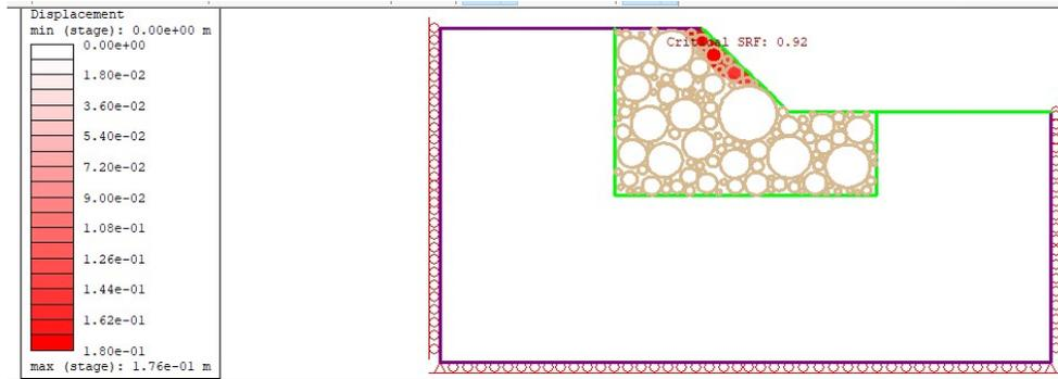
Figure 37 Total displacements of the 70% VBP model when cohesion is reduced by 100%
