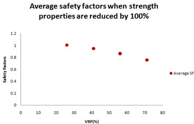
Figure 38 Safety factors with increasing VBP when cohesion and tensile strength of the block-matrix interfaces were reduced by 100%
