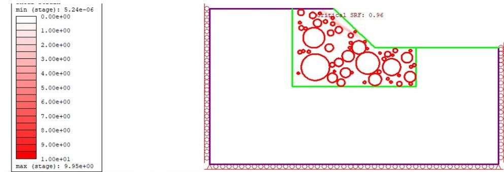
Figure 22 Maximum shear strains of the 40% VBP model when the cohesion of the block interfaces is reduced by 50%.
