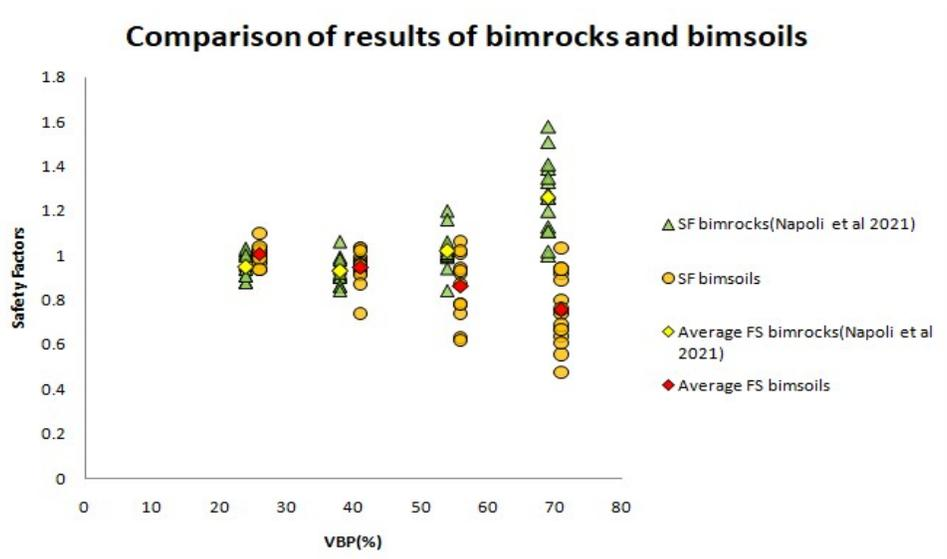
Figure 42 Comparison of Safety factors of bimrocks and bimsoil models with strength properties of block-matrix interfaces reduced to 100%
