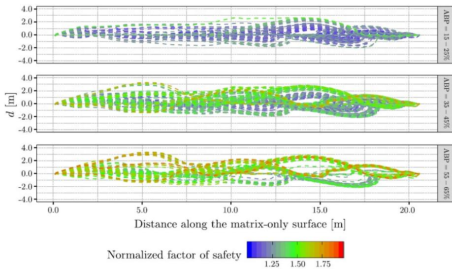
Figure 11 Possible Tortuous failure surfaces profiles for different Areal Block Proportions (ABPs) with respect the perpendicular depth  $d$  starting from the slope surface. It's evident that the roughest profiles are traced for the highest ABP (Montoya-Araque et al., 2020).
