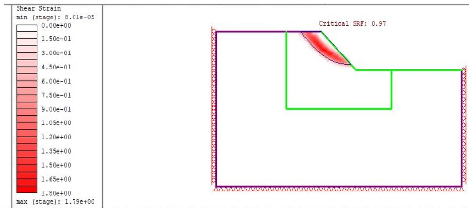
Figure 17 Maximum shear strain of the matrix only model (Napoli et al 2021)
