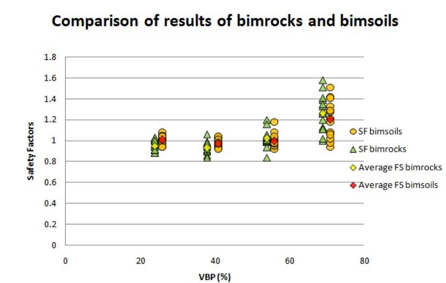
*Figure 29* Comparison of safety factors of bimrocks and bimsoils when cohesion and tensile strength of the block- matrix interfaces were reduced by 50%
