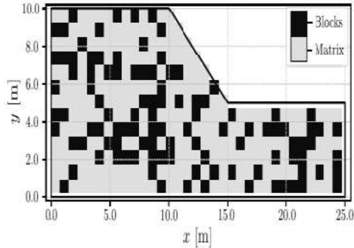
Figure 7 The most basic bimslope model (Montoya-Araque et al., 2020).
