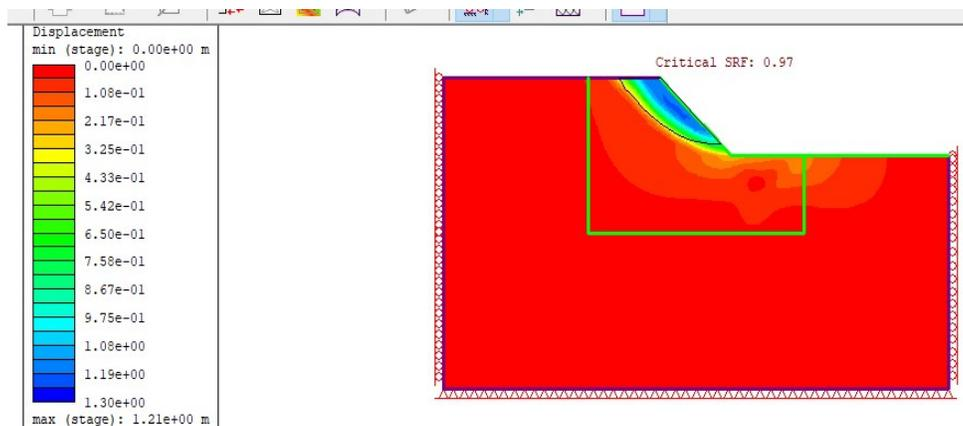
Figure 18 Total displacements of matrix only model. (Napoli et al 2021)
