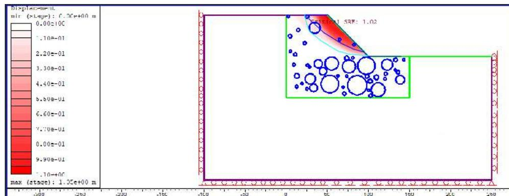
Figure 44 Failure surface of 25% VBP when strength properties of block- matrix interfaces and matrix are equal
