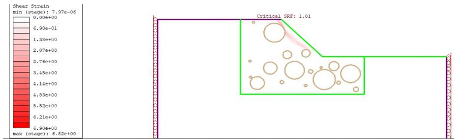
Figure 30 Maximum shear strains of 25% VBP model when the cohesion of the block-matrix interfaces is reduced by 100%.
