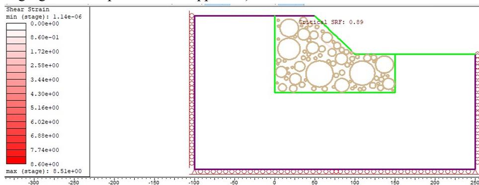
Figure 34 Maximum shear strain of the 55% VBP model when the cohesion of the block interfaces is reduced by 100%.
