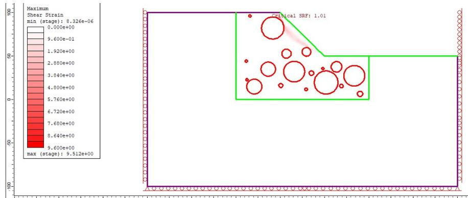
Figure 20 Maximum shear strain of the 25% VBP model when the cohesion of the block- matrix interfaces is reduced by 50%.
