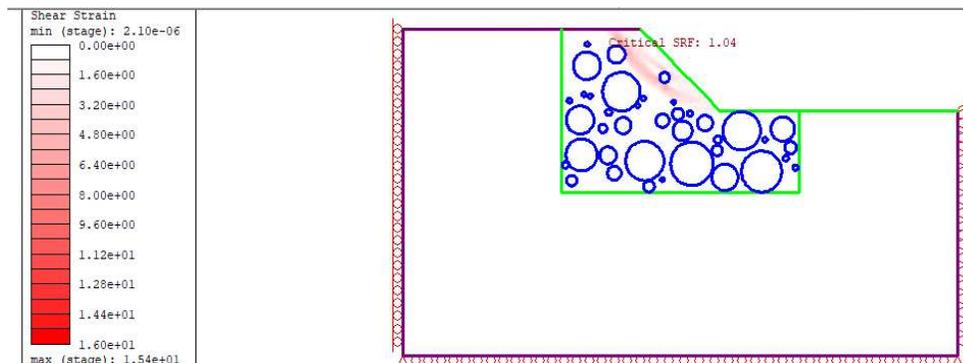
*Figure 19 maximum shear strains of the model with 40% VBP when the block- matrix interfaces have same strength properties as that of the matrix*
