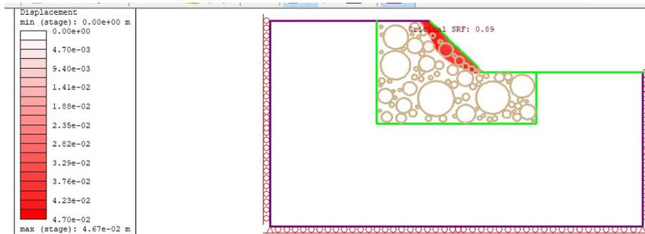
Figure 35 Total displacements in 55% VBP model when cohesion is reduced by 100%
