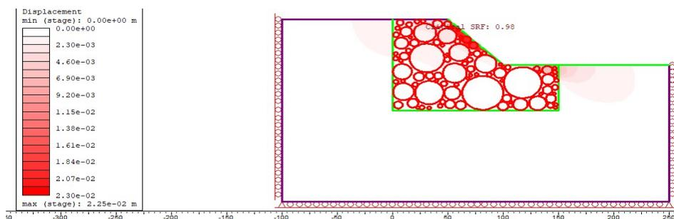
Figure 27 Total displacements in 70% VBP model when cohesion was reduced by 50%
