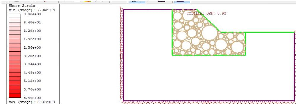
Figure 36 Maximum shear strain of the 70% VBP model when the cohesion of the block interfaces is reduced by 100%.
