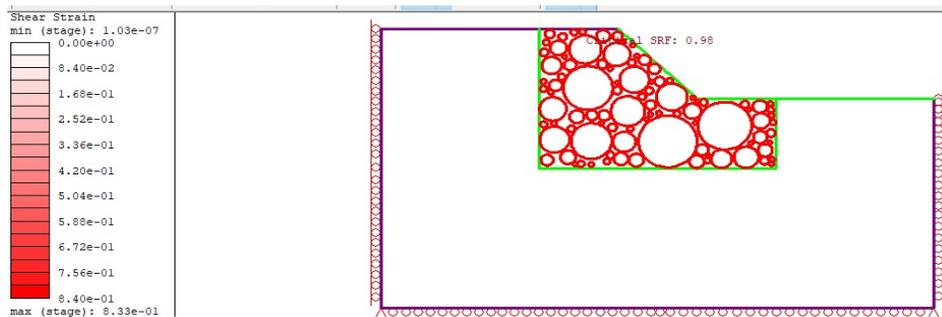
Figure 26 Maximum shear strain of the 70% VBP model when the cohesion of the block- matrix interfaces was reduced by 50%.
