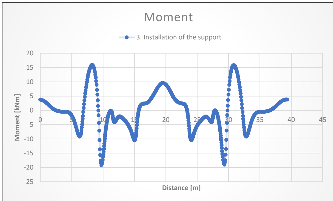
Figure 101 Bending moment vs the lining boundary distance
