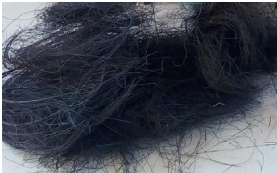
Figure 5: Steel fibers obtained after recycling the tires [10]
