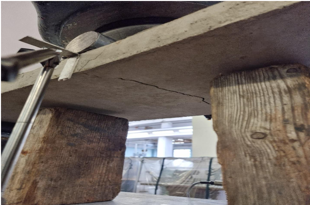
Figure 14: Failure of Reinforced Cement Concrete Under Tension Loading
