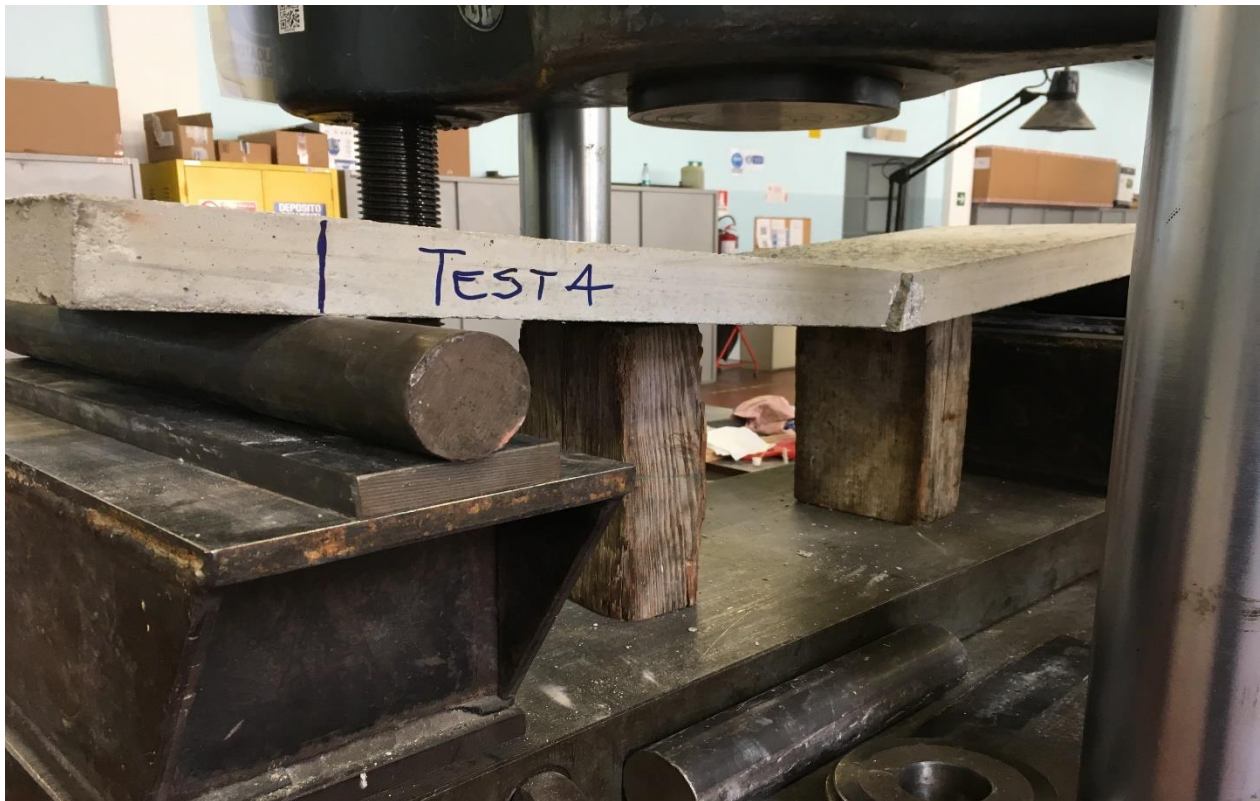
Figure 13: Failure of Plain Cement Concrete Under Tension Loading
