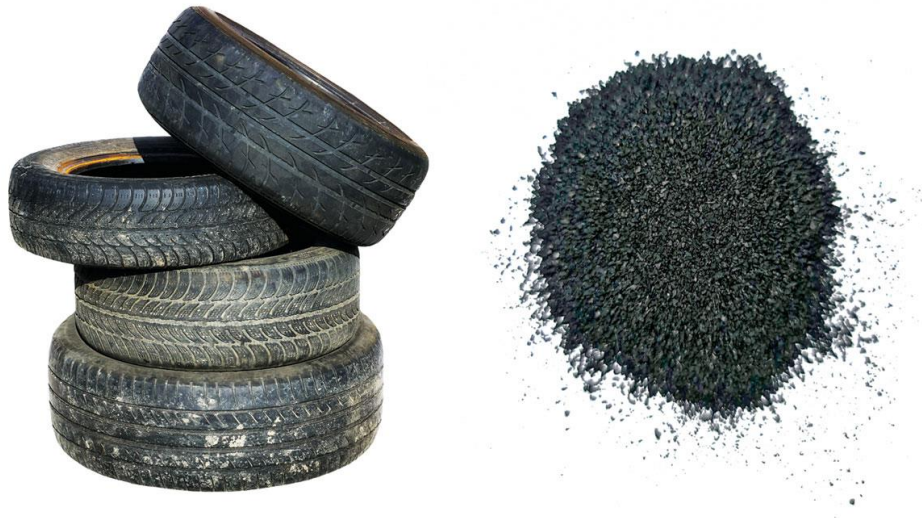
Figure 3: Granular finish obtained from Waste Tires
