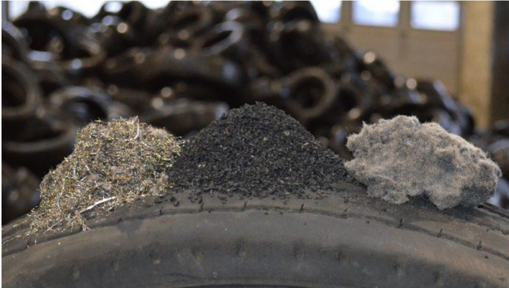
Figure 4: Different Recycled Components from Waste Tires
