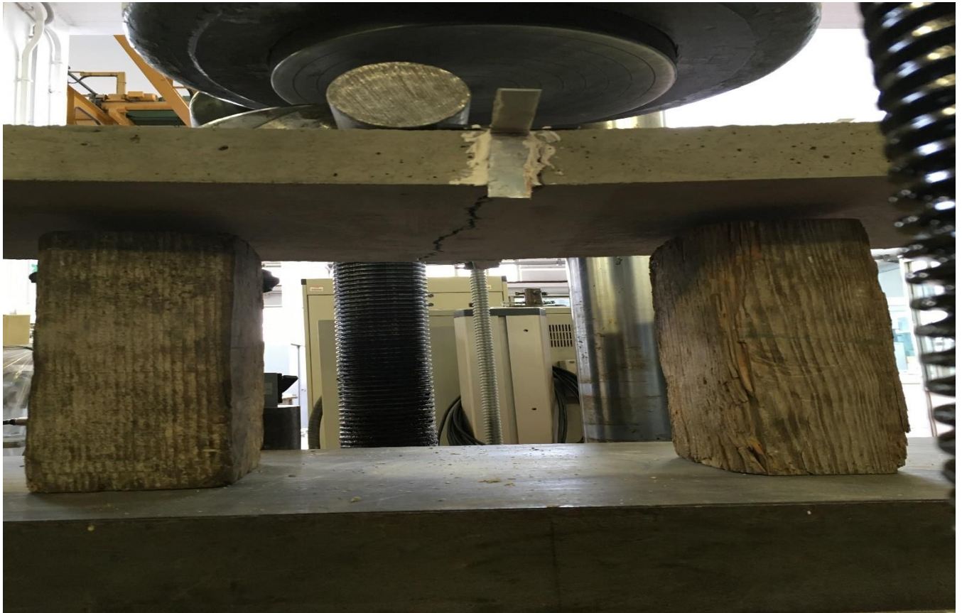
Figure 16: Failure in Steel and Recycled Steel Fiber Reinforced Concrete
