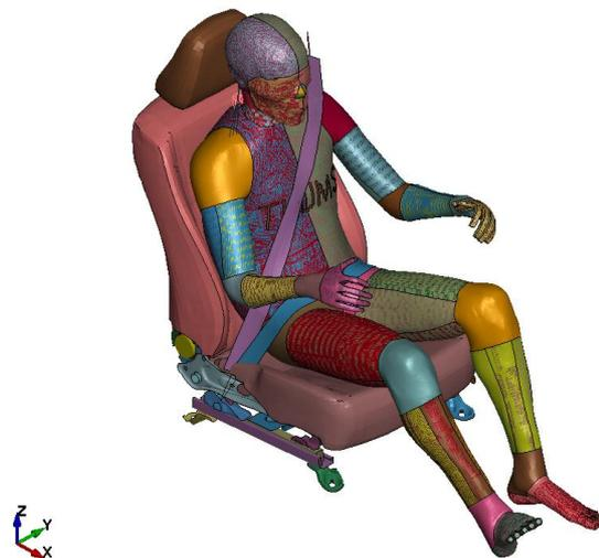
*Figure 18 THUMS positioned with the seatbelt model*
