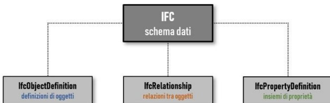
FIGURA 53 STRUTTURA GERARCHICA DI UN FILE IFC [FONTE: BIM.ACCA.IT]
