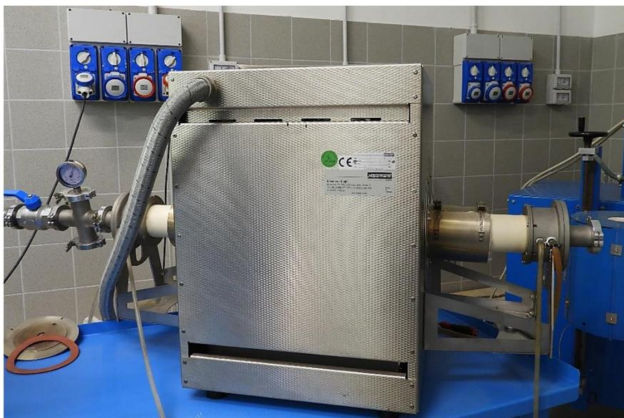
*Figura 3.4 - Forno Nabertherm, RHTH 70-150/16, Germany*
