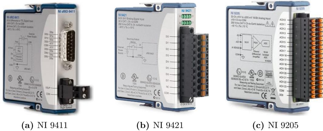
Figure 4.3: NI acquisition boards
