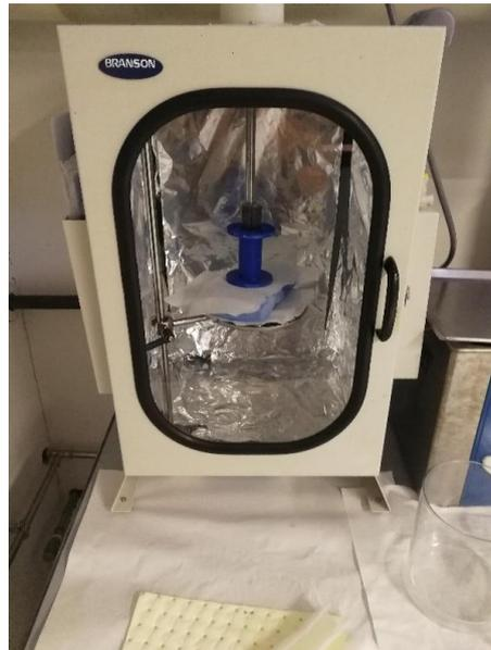
Figure 4.1: Branson ultrasonicator used to better disperse MWCNTs inside the solution.
