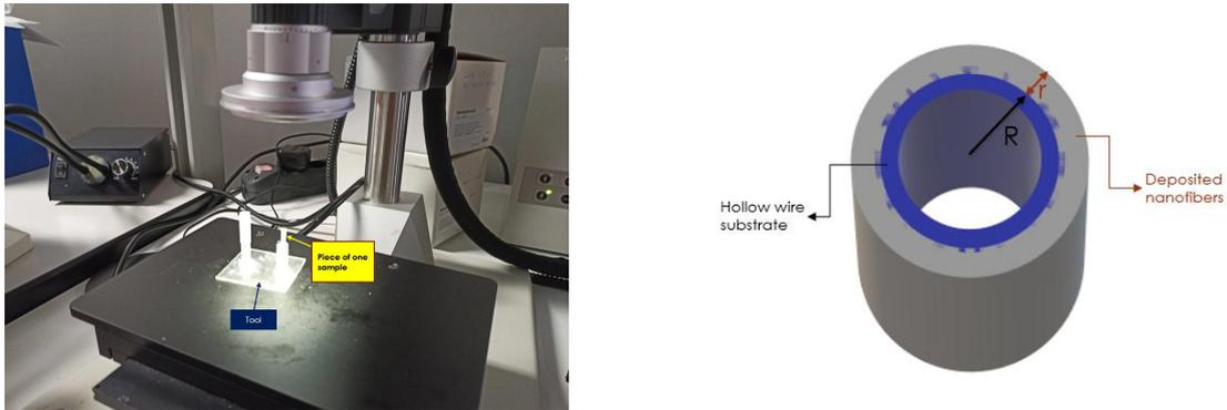
Figure B.4: (Left) Set up used for nanofiber mat thickness. (Right) Schematic representation of a sample cross section.
