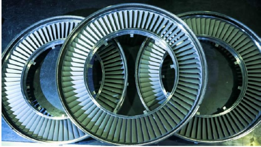
**Figure 2.1: Example of cyclic symmetry structure.**
