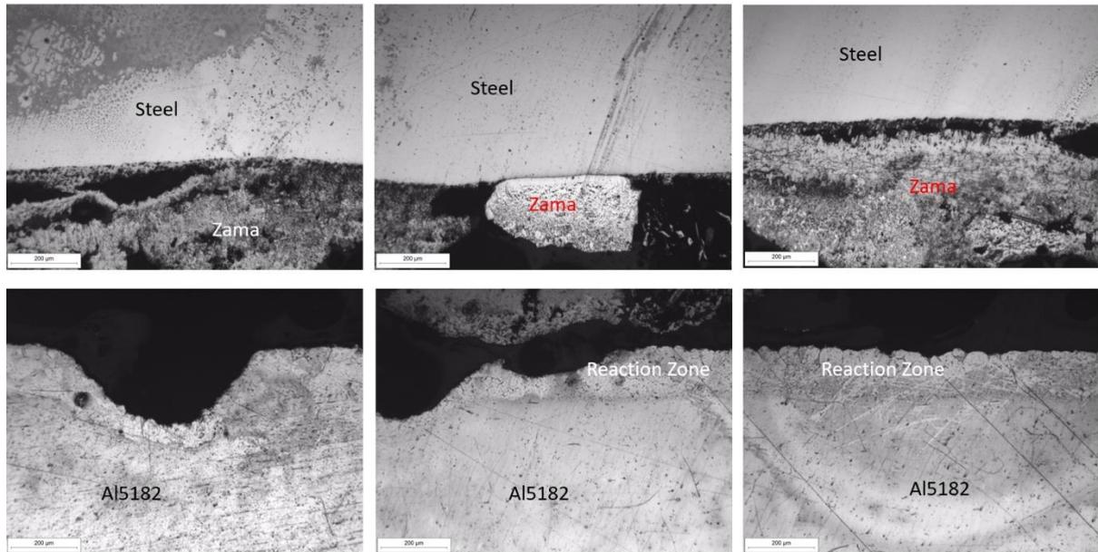
Figure 74: Optical microscope images of the transverse section of the samples of Zn-steel, Al5182, Zama at 50x magnification
