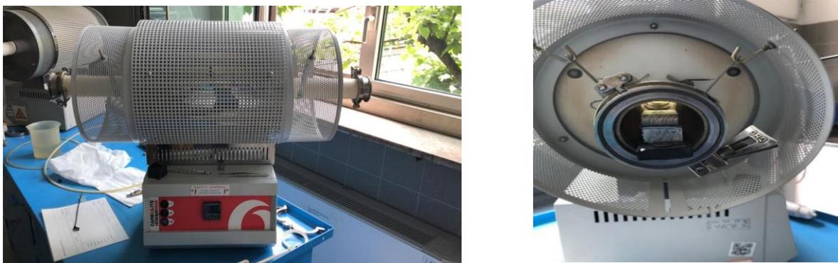
Figure 38: Tubular furnace for brazing
