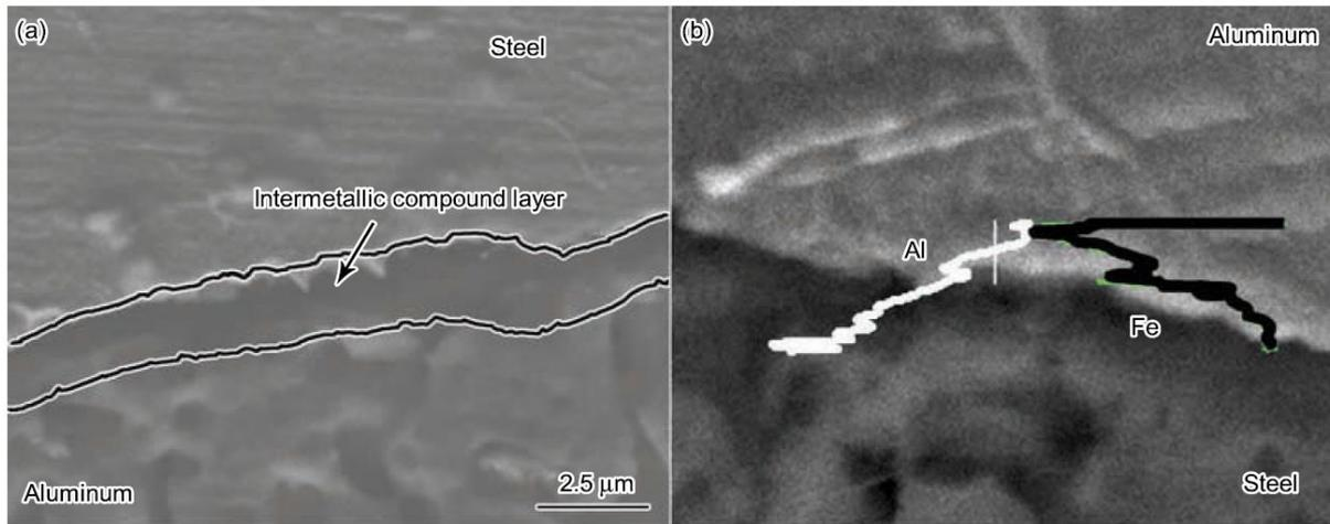
Figure 11: microstructures of spot welding (a) SEM images for IMC layers, (b) EDX analysis crossing the IMC layer [27]
