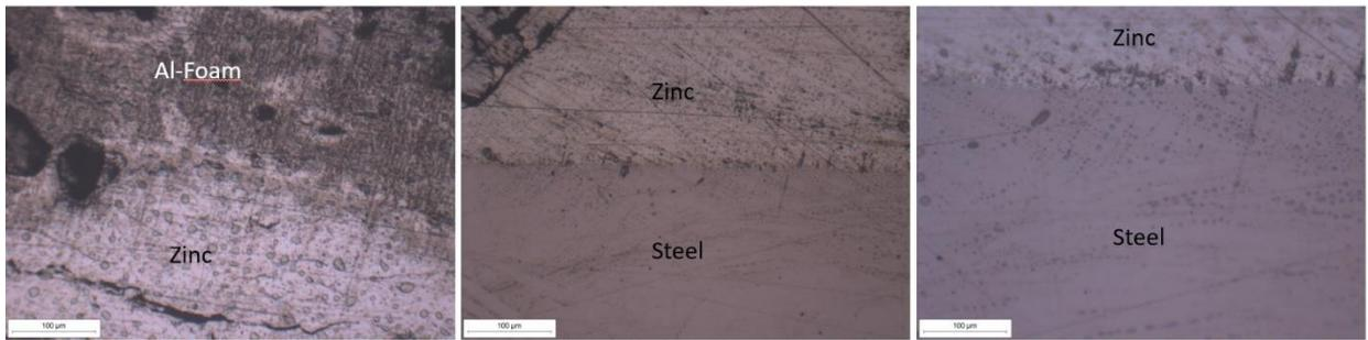
Figure 90: Optical microscope images of the transverse section of the samples of Zn-steel, Al-Foam, Zinc at 200x magnification
