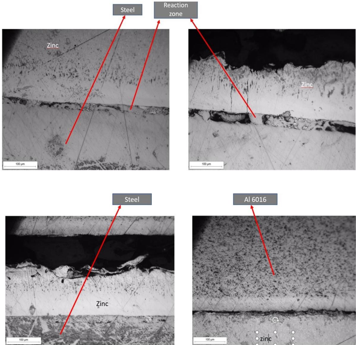
Figure 61: Optical microscope images of the transverse section of the samples of Zn-steel, Al6016 and Zn at higher magnifications
