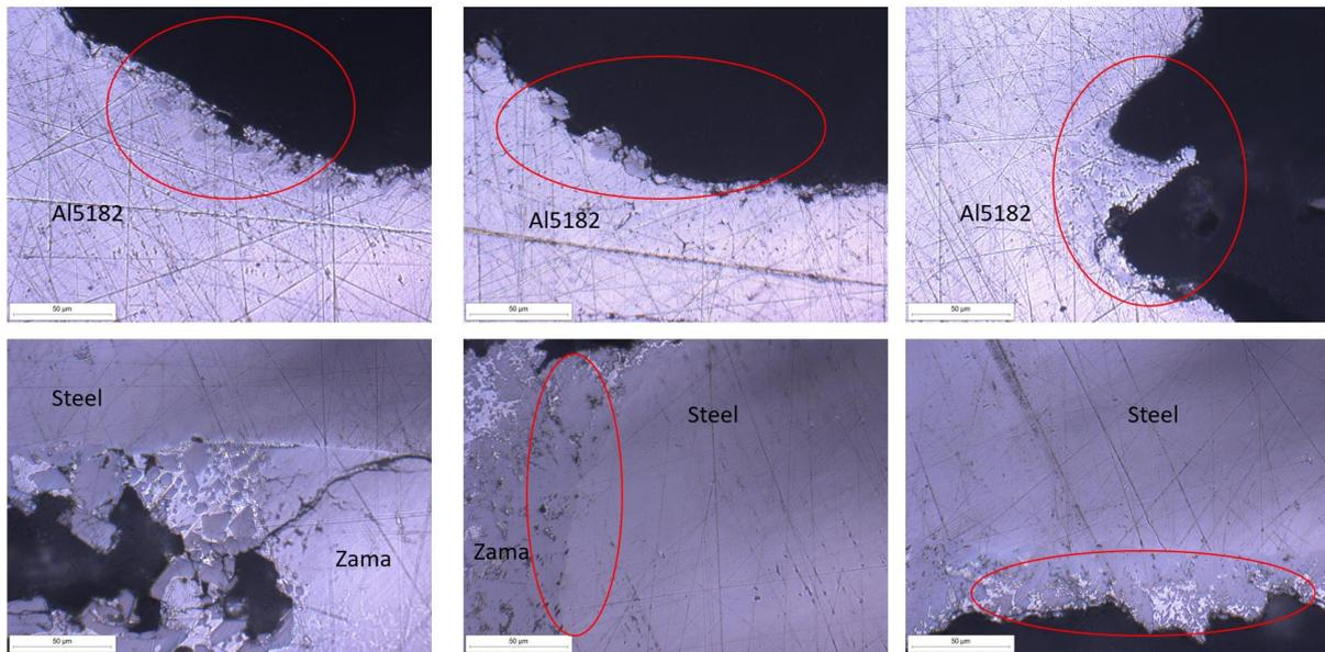
Figure 86: Optical microscope images of the transverse section of the samples of Zn-steel, Al5182, Zama at 500x magnification
