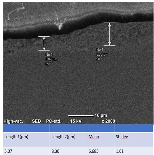
Figure 56: Width of Zn coating in Zinc coated steel
