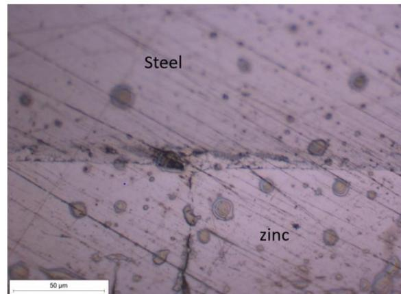
Figure 64: Optical microscope images of the transverse section of the samples of Zn-steel, Al6016 (no flux) and Zn at different magnifications
