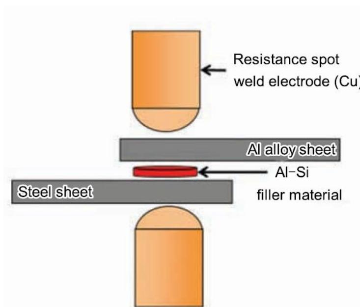
Figure 12:schematic drawing of specimen using filler metal for resistance spot brazing[27]
