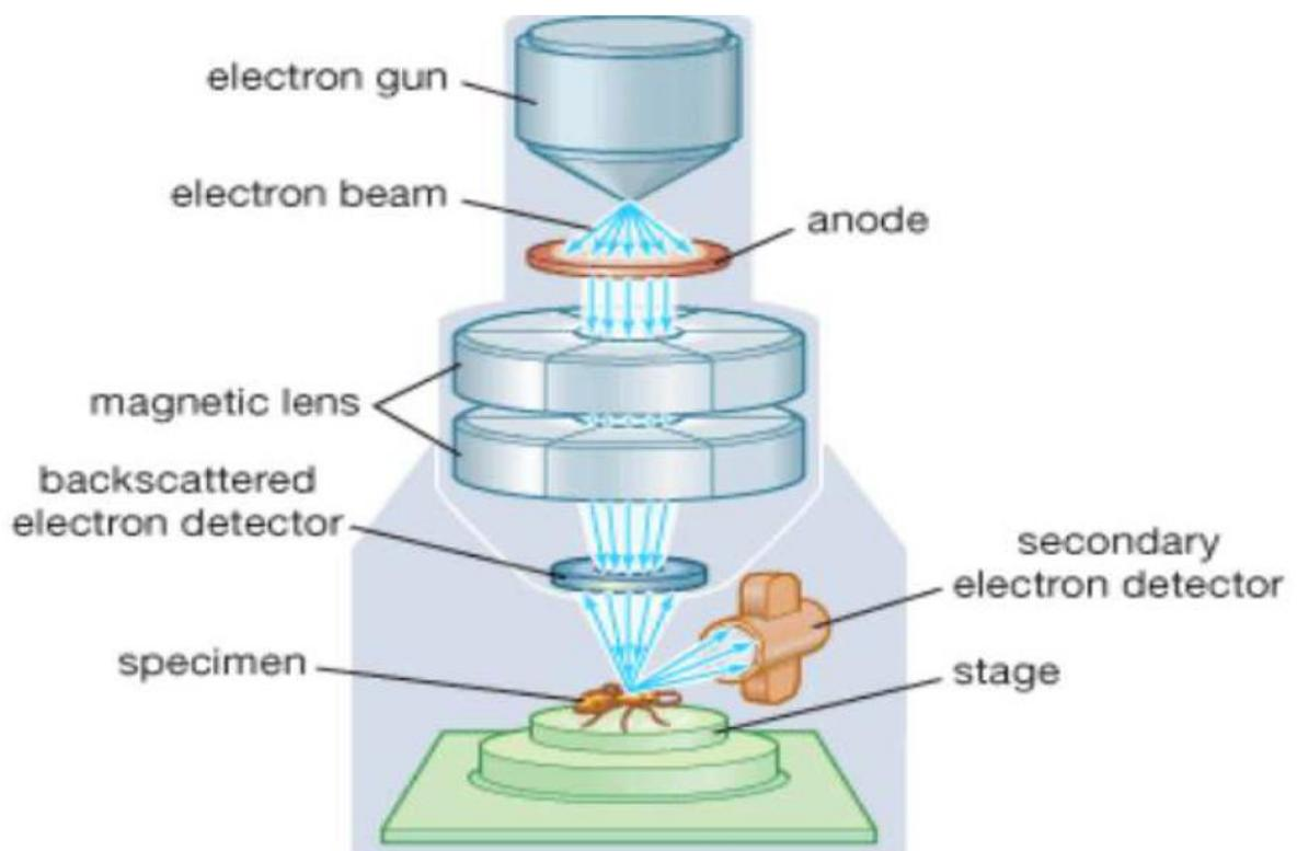
Figure 46: Basic Configuration of SEM[46]
