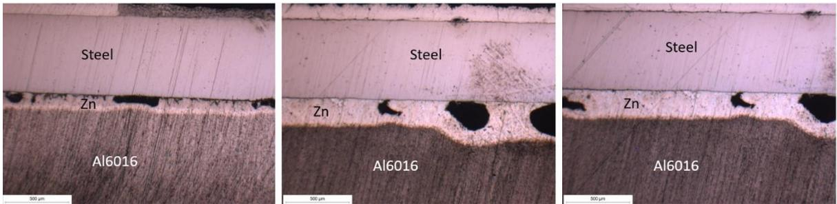
Figure 66: Optical microscope images of the transverse section of the samples of Zn-steel, Al6016 (flux) and Zn at 50x magnification
