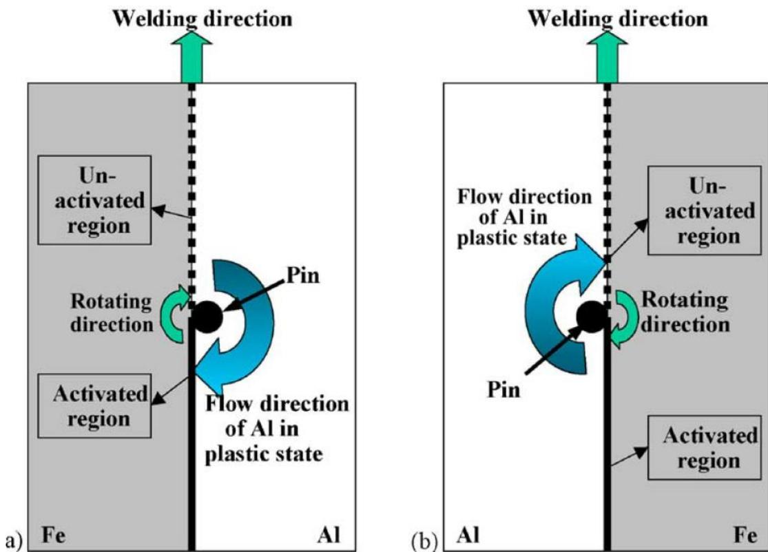
Figure 20: schematic representation of the rotating direction of the pin and activated surface of steel [32]
