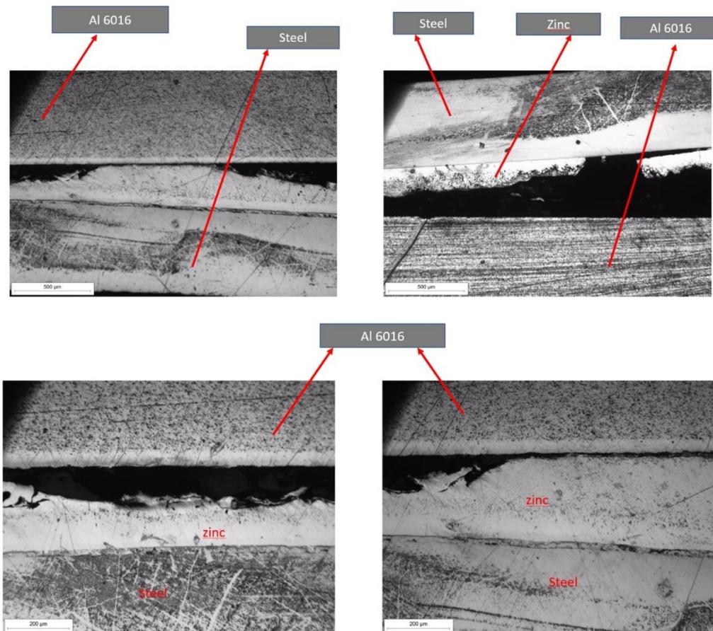
Figure 60: Optical microscope images of the transverse section of the samples of Zn-steel, Al6016 and Zn at different magnifications
