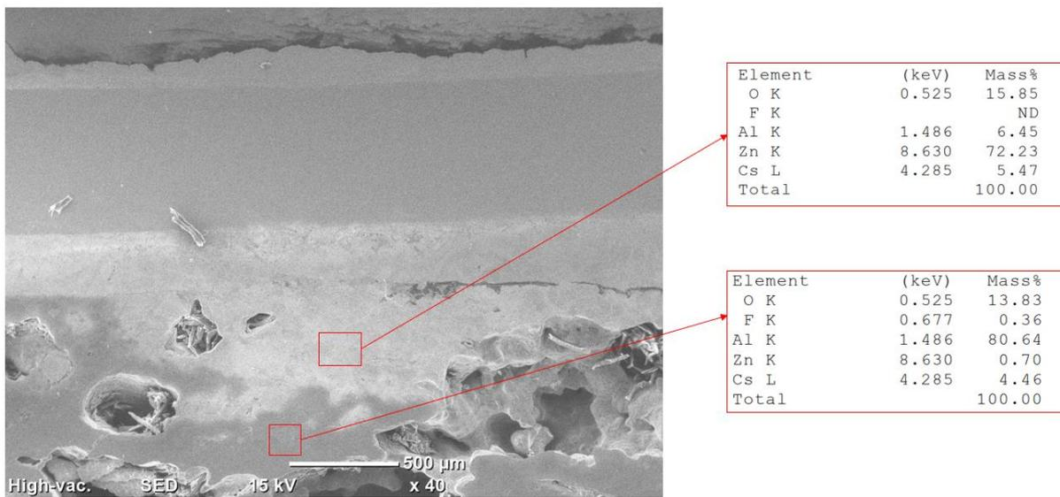
Figure 94: EDS analysis of Al-foam (FLUX), Zn-Steel and Zn at 40x magnification
