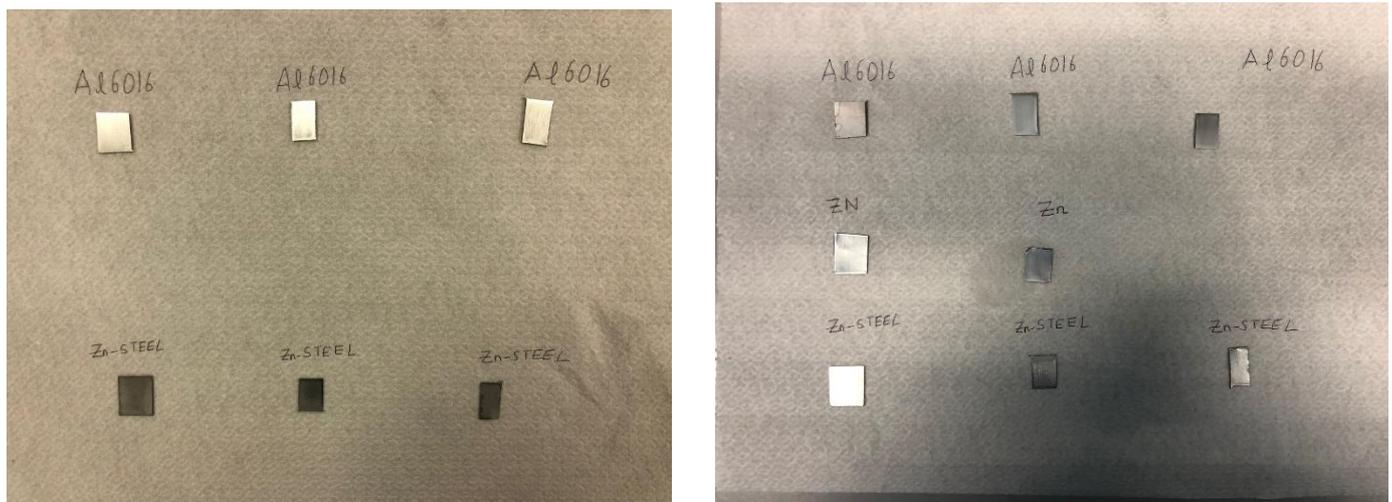
Figure 62: (a left) samples after treated with P320 abrasive paper (b right) samples after cleaning in ultrasonic bath
