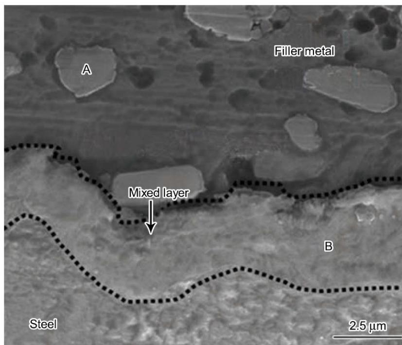
Figure 13: Microstructure of interfacial layer between the filler metal layer and steel sheet for resistance spot brazed [27]
