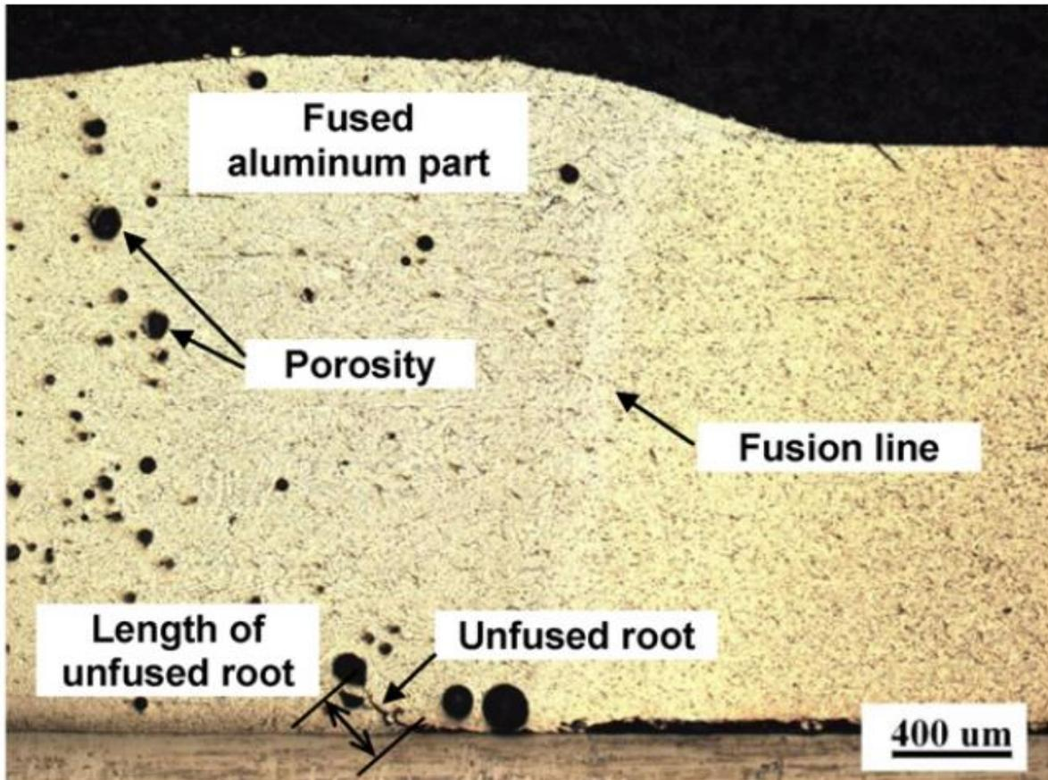
Figure 27: micro defects in cross-section [34]
