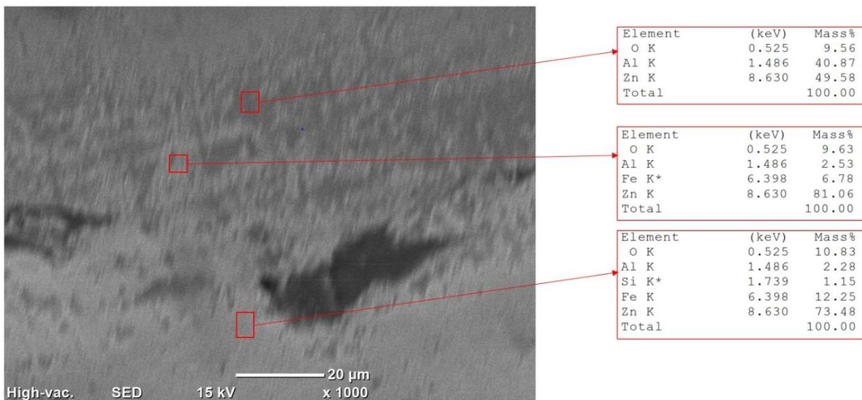
Figure 103: EDS analysis of Al-Foam, Zn-steel, and Zinc at 1000x magnification
