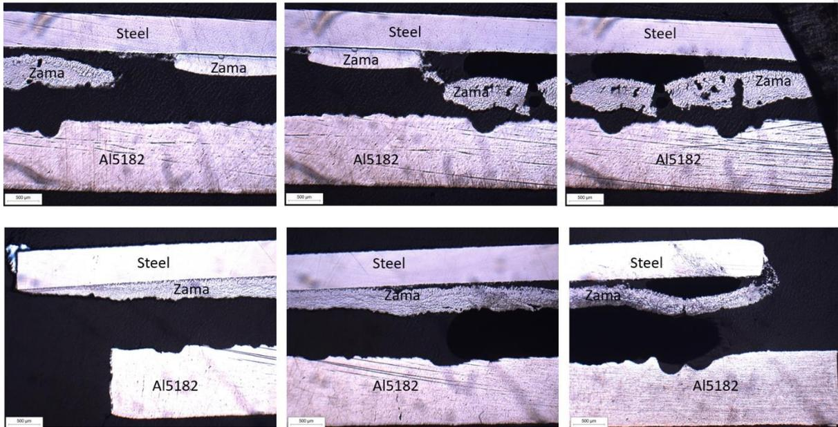
Figure 82: Optical microscope images of the transverse section of the samples of Zn-steel, Al5182, Zama at 20x magnification
