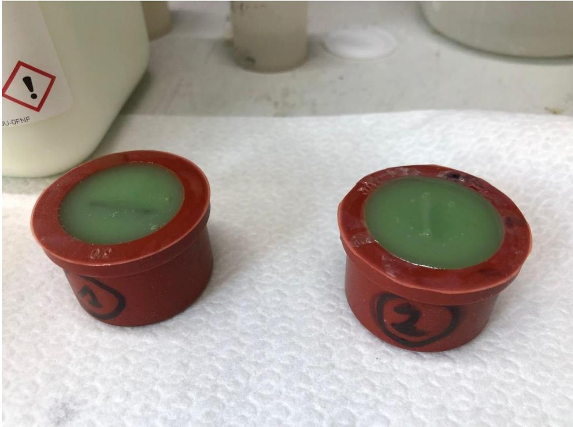
*Figure 42: Samples after they are inside the resin*
