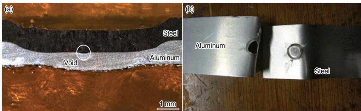
Figure 10: resistance spot welding specimen (a) formation of the IMC layers and voids (b) button fracture of aluminum [27]
