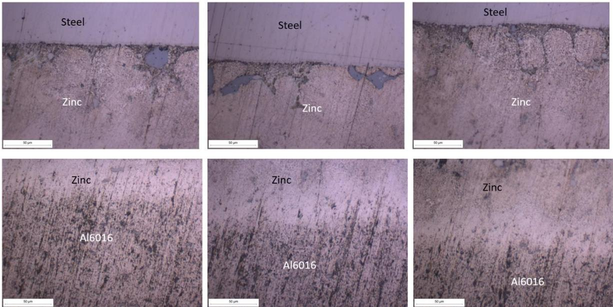
Figure 69: Optical microscope images of the transverse section of the samples of Zn-steel, Al6016 (flux) and Zn at 400x magnification
