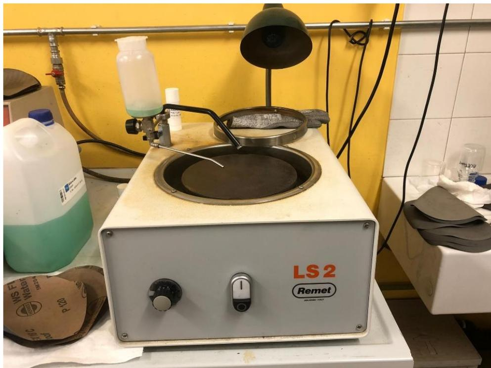
*Figure 44: Polishing Machine used in experimentation*
