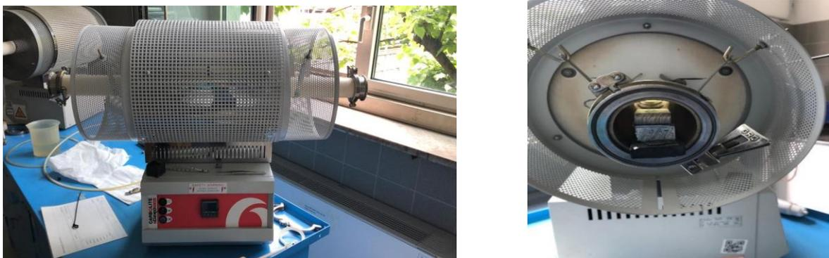
Figure 38: Tubular furnace for brazing
