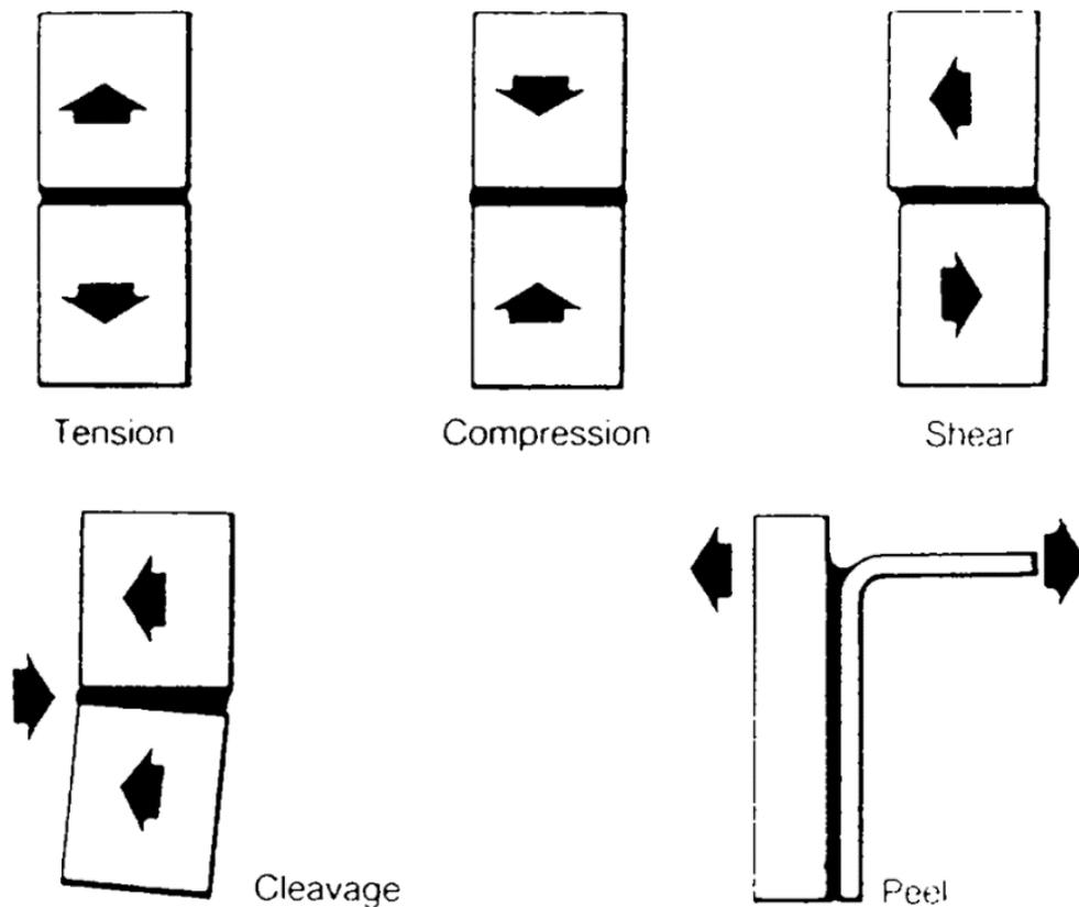
Figure 3: loading conditions for adhesive bonded joints [10]
