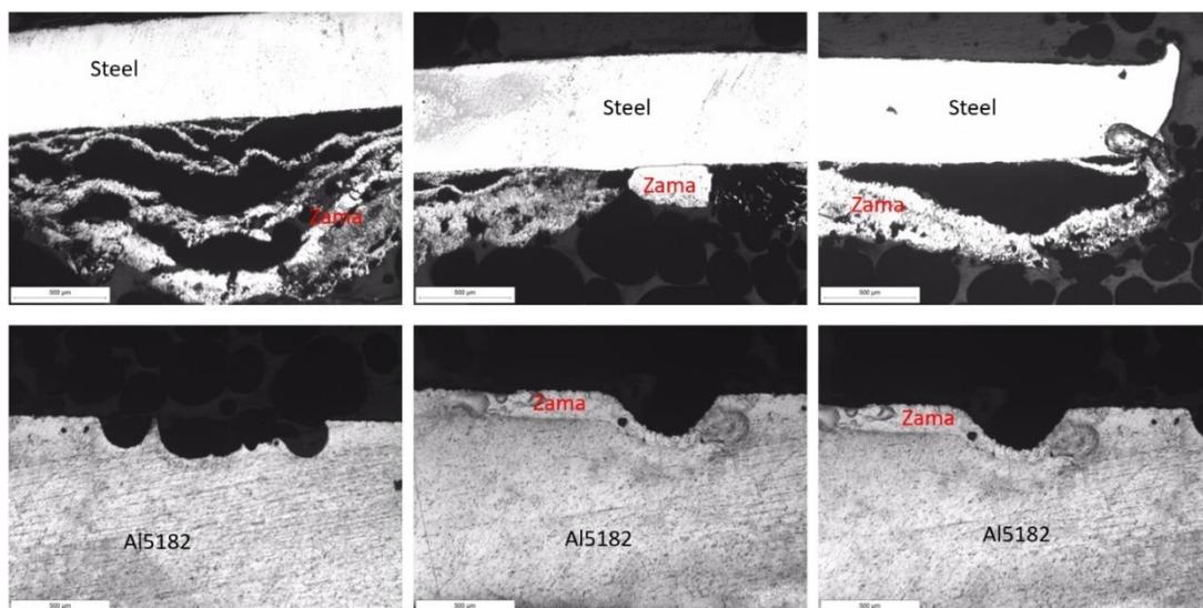
Figure 73: Optical microscope images of the transverse section of the samples of Zn-steel, Al5182, Zama at 20x magnification
