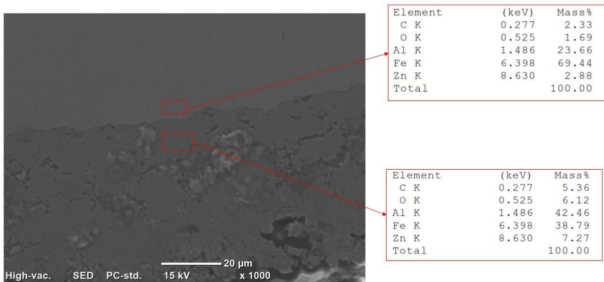
Figure 78 : EDS analysis of Al5182, Zn-steel and Zama
