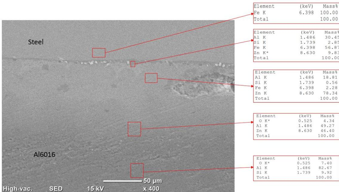
Figure 72: SEM and EDS analysis of Al6016(flux), Zn-steel, Zn at 400x magnification
