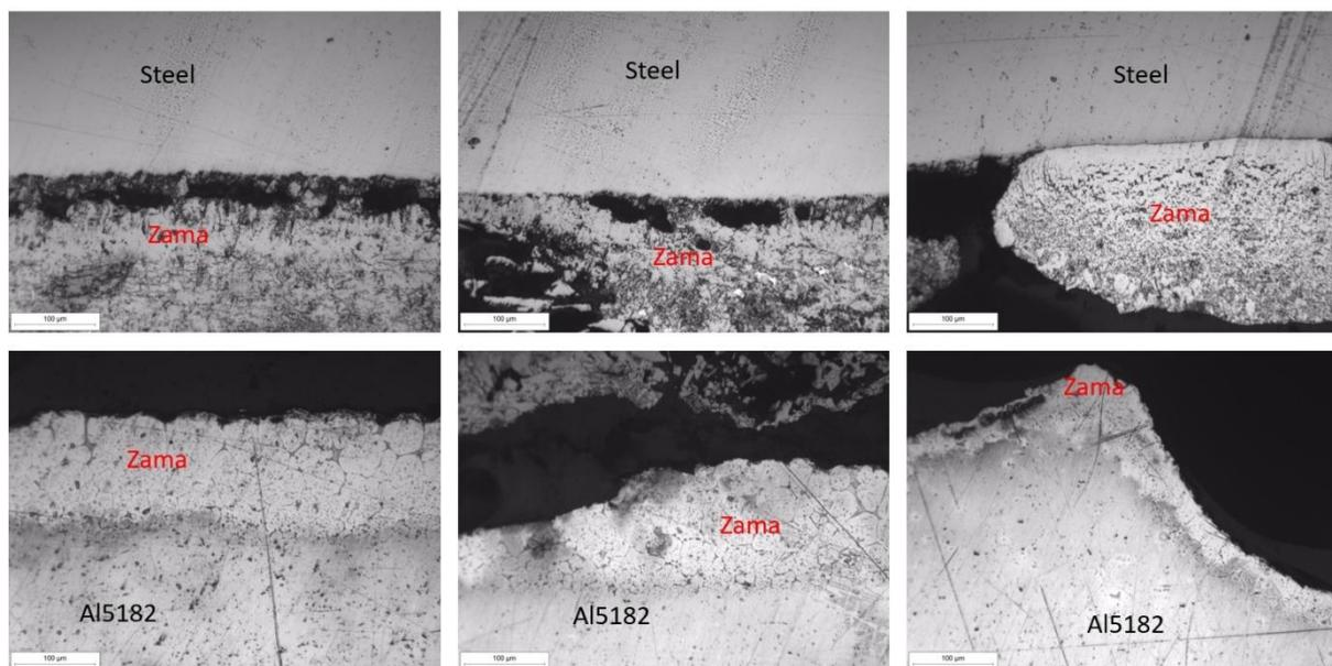
Figure 75: Optical microscope images of the transverse section of the samples of Zn-steel, Al5182, Zama at 100x magnification
