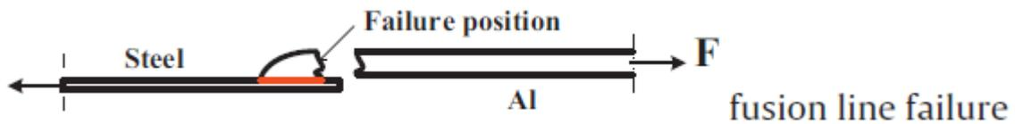
Figure 26: Depiction of Failure Mode[34]
