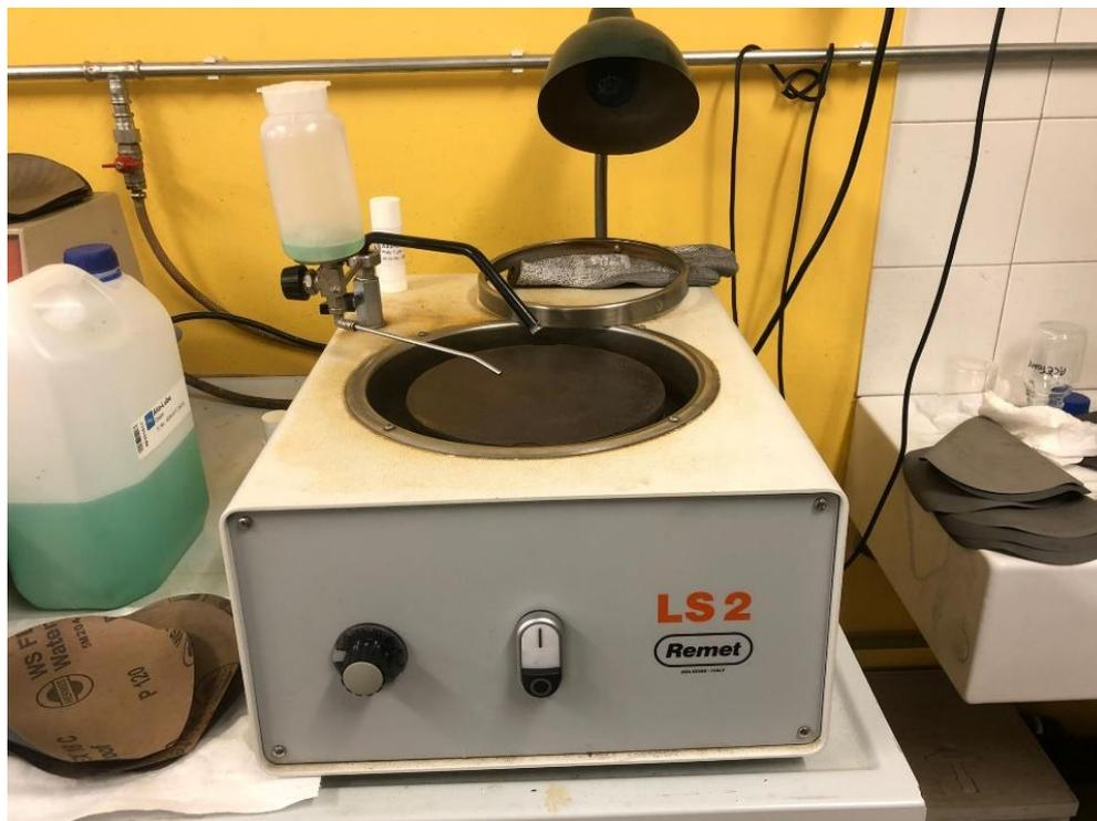
*Figure 44: Polishing Machine used in experimentation*
