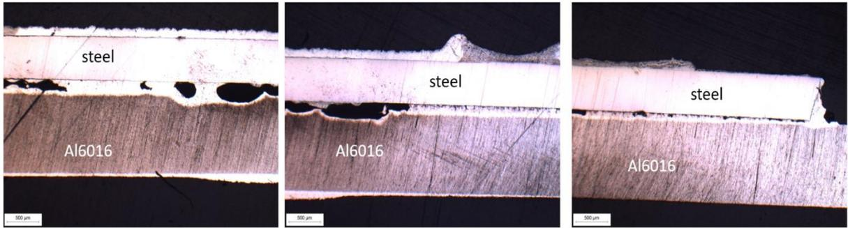
Figure 65: Optical microscope images of the transverse section of the samples of Zn-steel, Al6016 (flux) and Zn at 20x magnification
