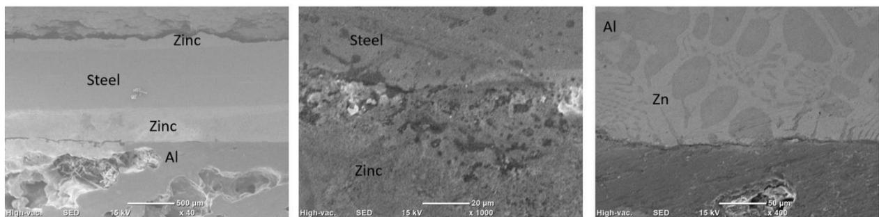
Figure 92: Images taken by SEM at 40x, 1000x and 400x
