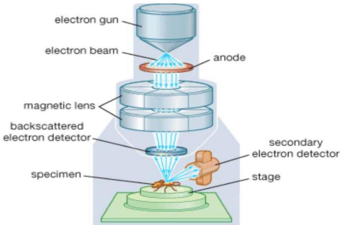
Figure 46: Basic Configuration of SEM[46]
