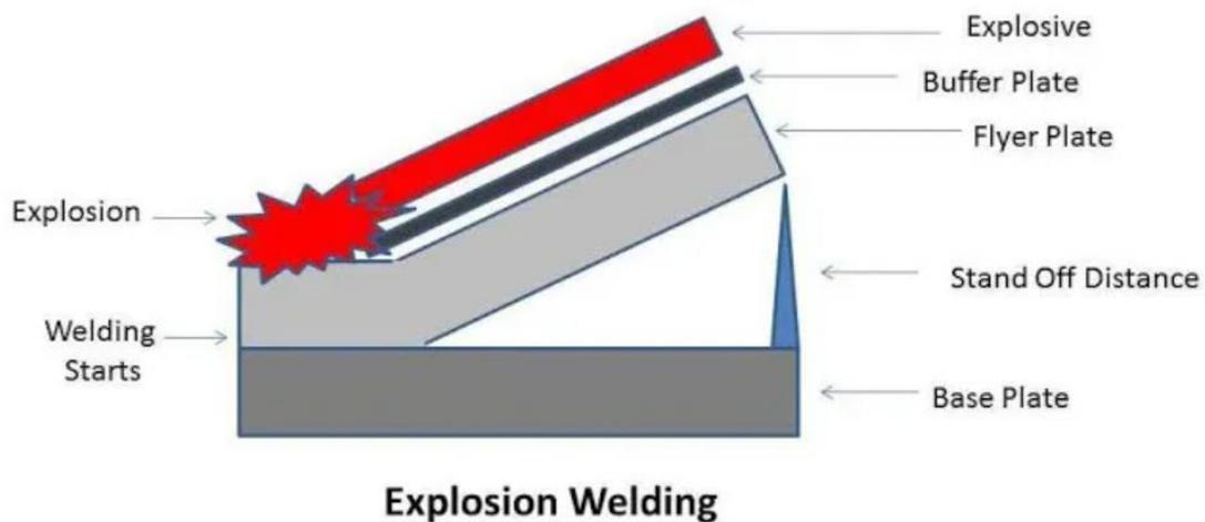
Figure 9: explosion welding schematic[22]
