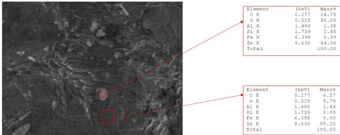
Figure 53: Point analysis of the Zn-steel top surface at magnifications of 2000x
