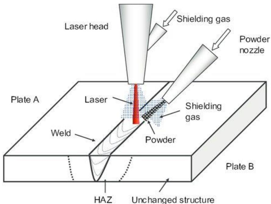
Figure 4: Laser Beam Welding
