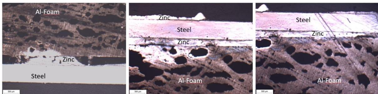
Figure 87: Optical microscope images of the transverse section of the samples of Zn-steel, Al-Foam, Zinc at 20x magnification
