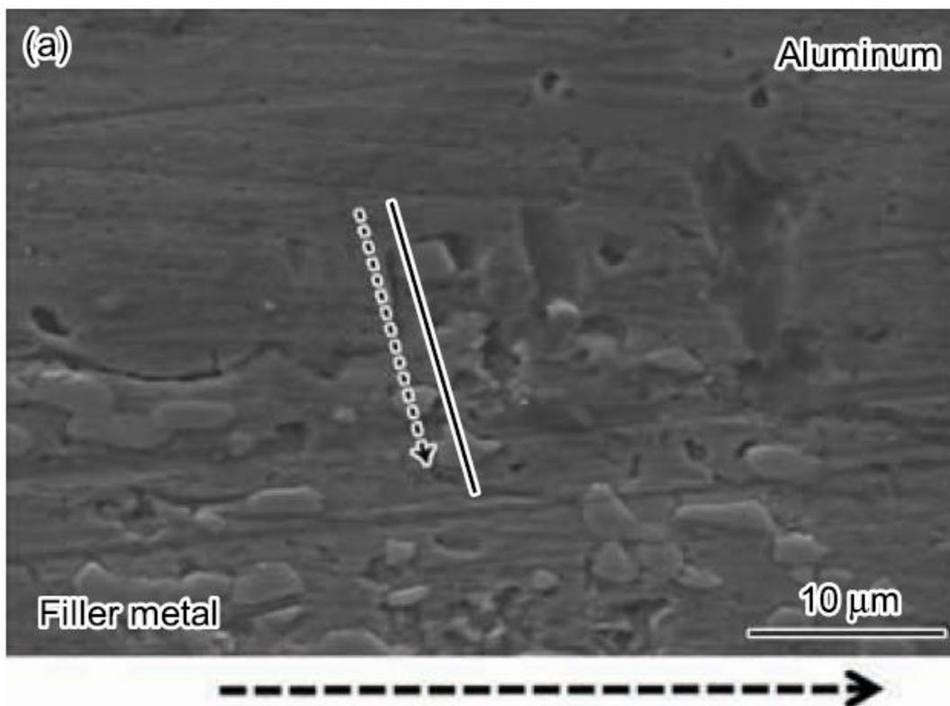
Figure 14: Line scanning of EDX analysis of interfacial layer [27]
