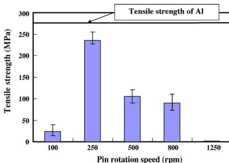
Figure 18: relation between pin rotation speed and tensile strength of the joint [32]
