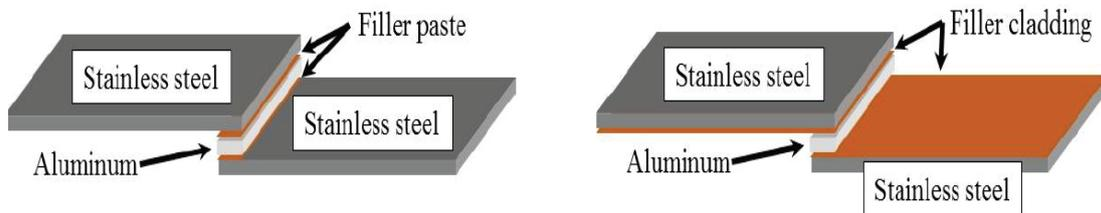
Figure 15: different setups for brazing joints[30]
