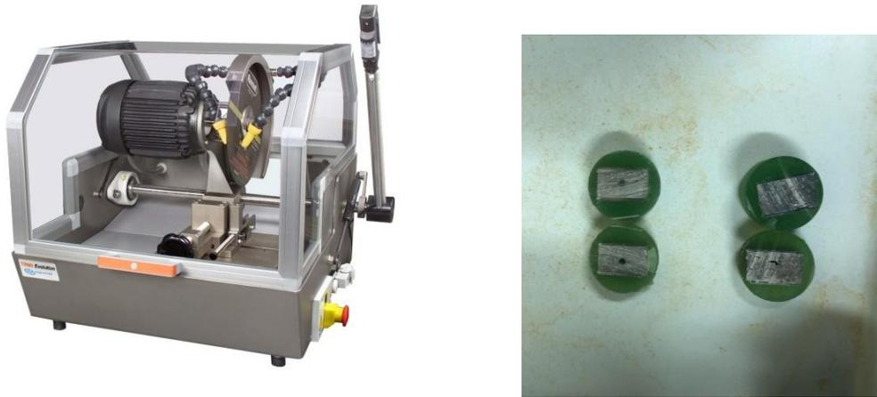
Figure 43: (a) TR80 EVOLUTION Abrasive Cutter (b) Sample after being transversely cut
