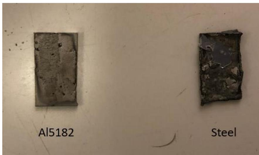
Figure 80: Unjoin sample of Al5182, Steel and Zama for 10 minutes dwell time
