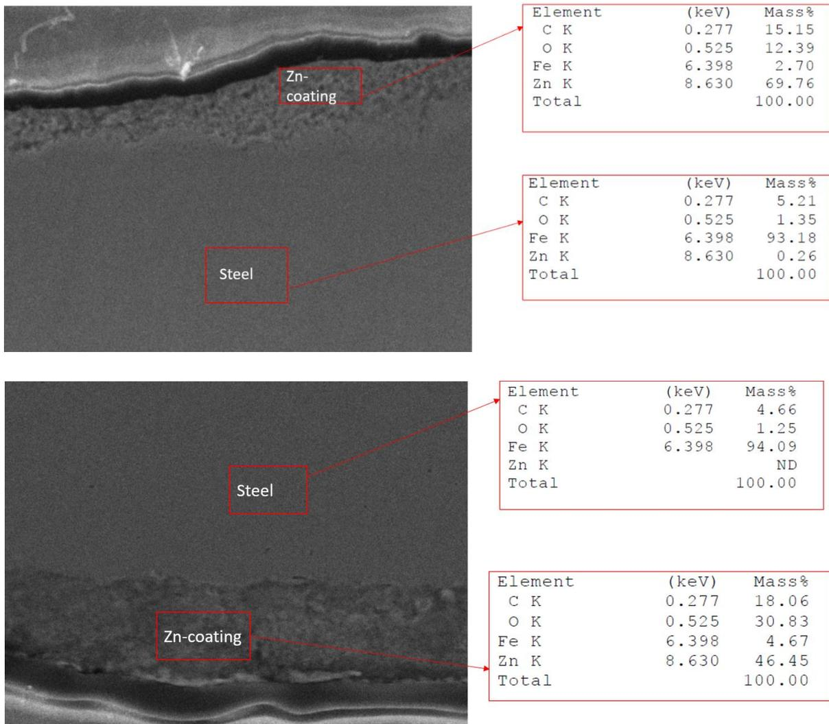
Figure 55:EDS point analysis of Zn-Coated steel section on 2 different points
