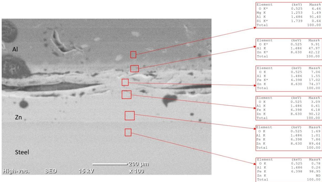
Figure 102: EDS analysis of Al-Foam, Zn-steel, and Zinc at 100x magnification
