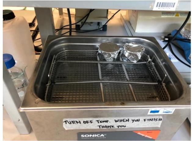
Figure 35 Ultrasonic cleaner for cleaning the sample
