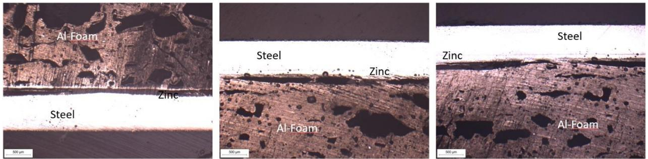
Figure 97: Optical microscope images of the transverse section of the samples of Zn-steel, Al-Foam, Zinc at 20x magnification
