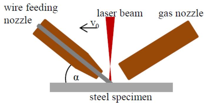
Figure 21: Setup for bead-on-plate laser brazing [33]
