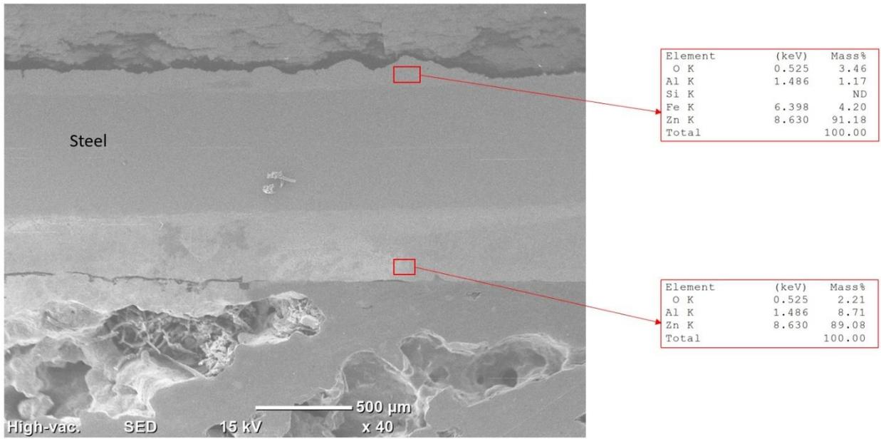
Figure 93: EDS analysis of Al-foam (FLUX), Zn-Steel and Zn at 40x magnification
