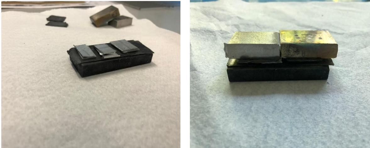
Figure 37 (a) Sandwich of Al, Zn, Zn-steel (b) final sample to put in furnace
