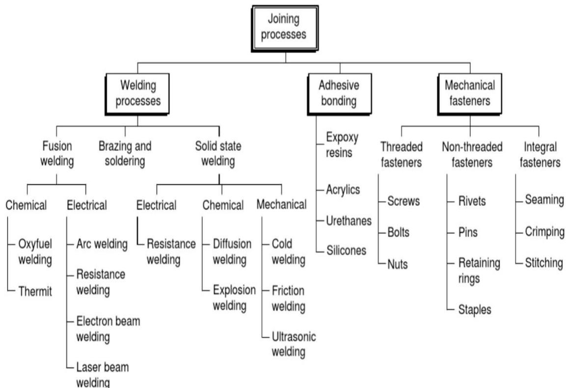
Figure 1: classification for the generic joining processes[7]
