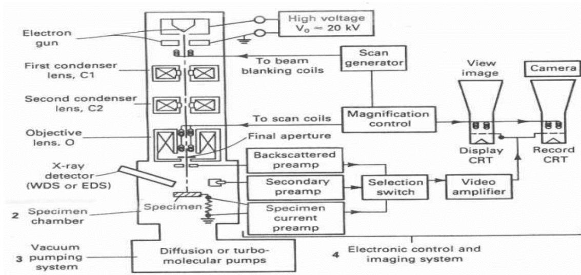
Figure 47: Detailed Working Diagram of SEM[46]
