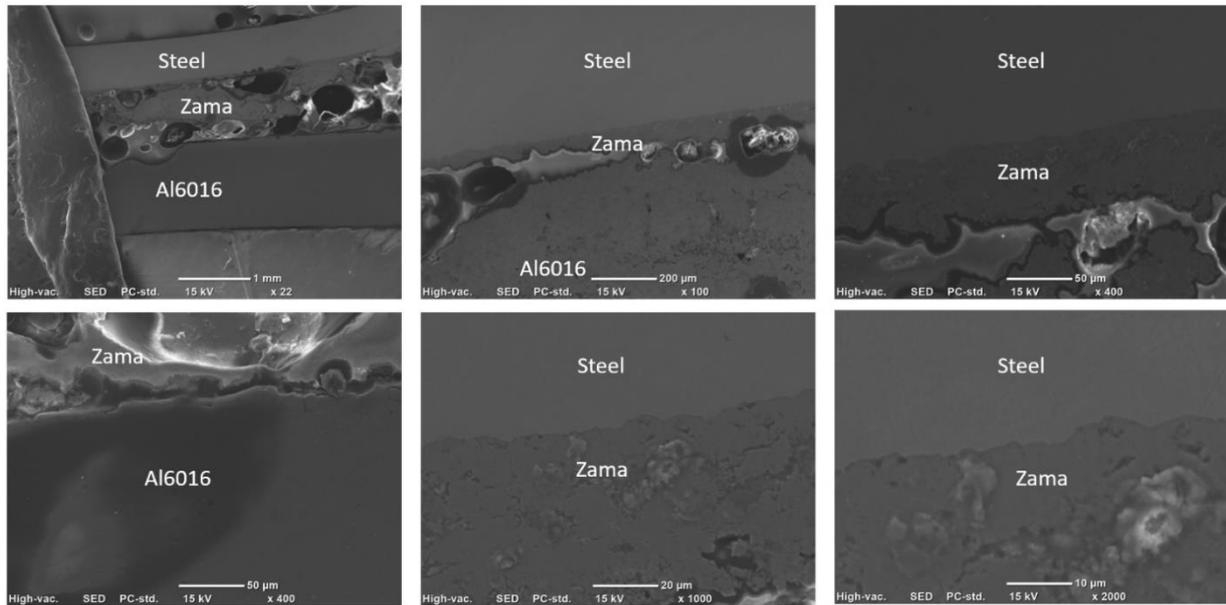
Figure 76: SEM images for Al5182, Zn-Steel, Zama at 22x, 100x, 400x, 1000x, 2000x magnification
