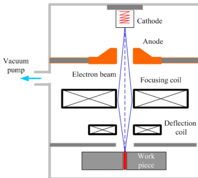
Figure 5: Electron Beam Welding
