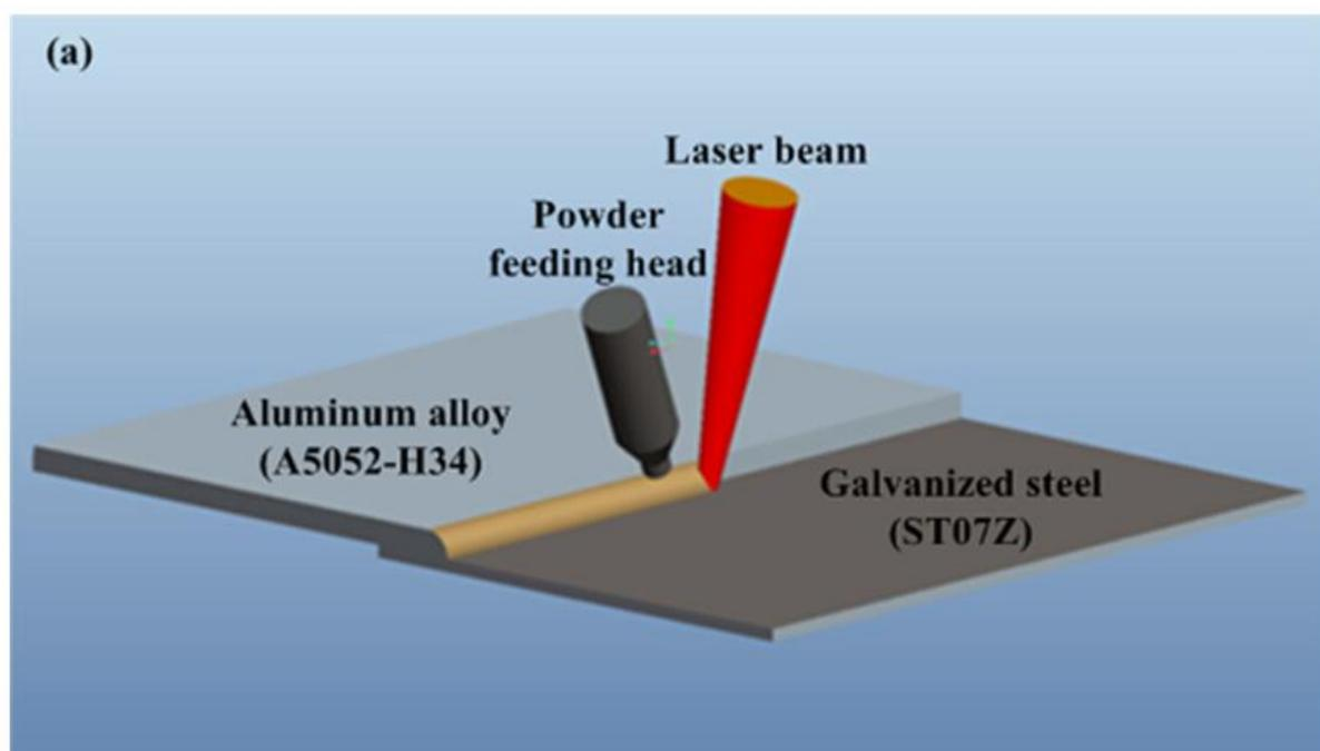
Figure 28: 3-D schematic view of the welding process [38]
