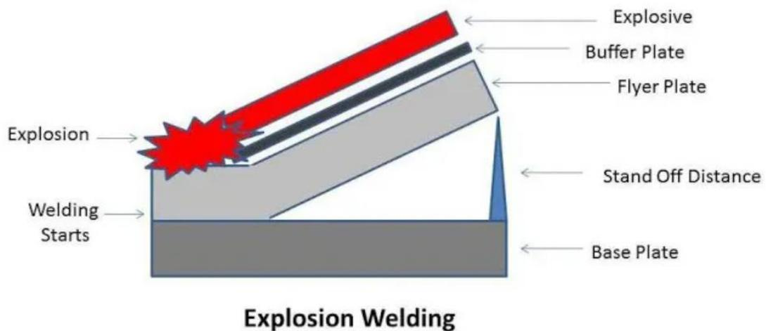
Figure 9: explosion welding schematic[22]
