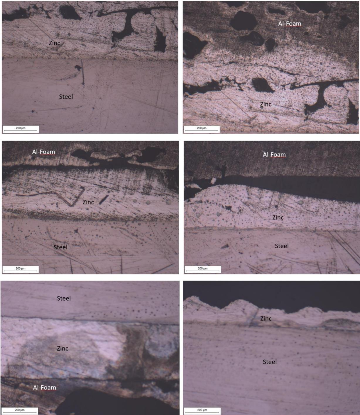
Figure 89: Optical microscope images of the transverse section of the samples of Zn-steel, Al-Foam, Zinc at 100x magnification
