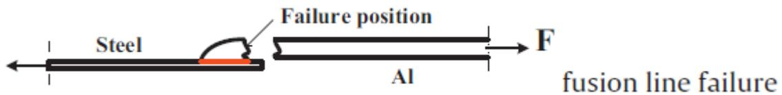
Figure 26: Depiction of Failure Mode[34]
