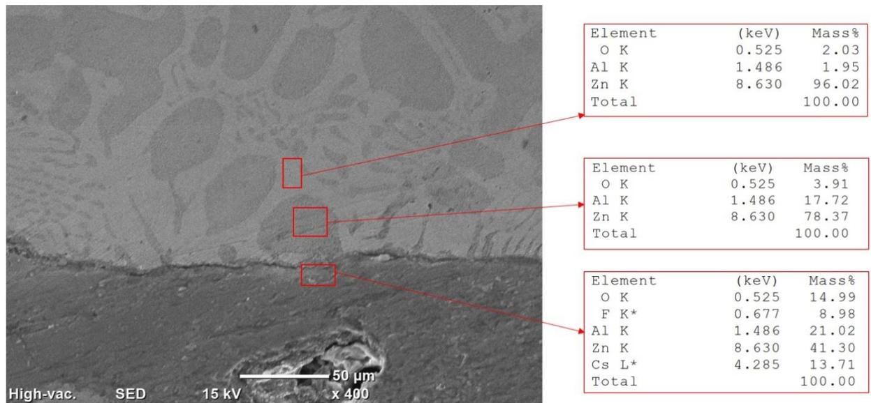
Figure 95: EDS analysis of Al-foam (FLUX), Zn-Steel and Zn at 400x magnification
