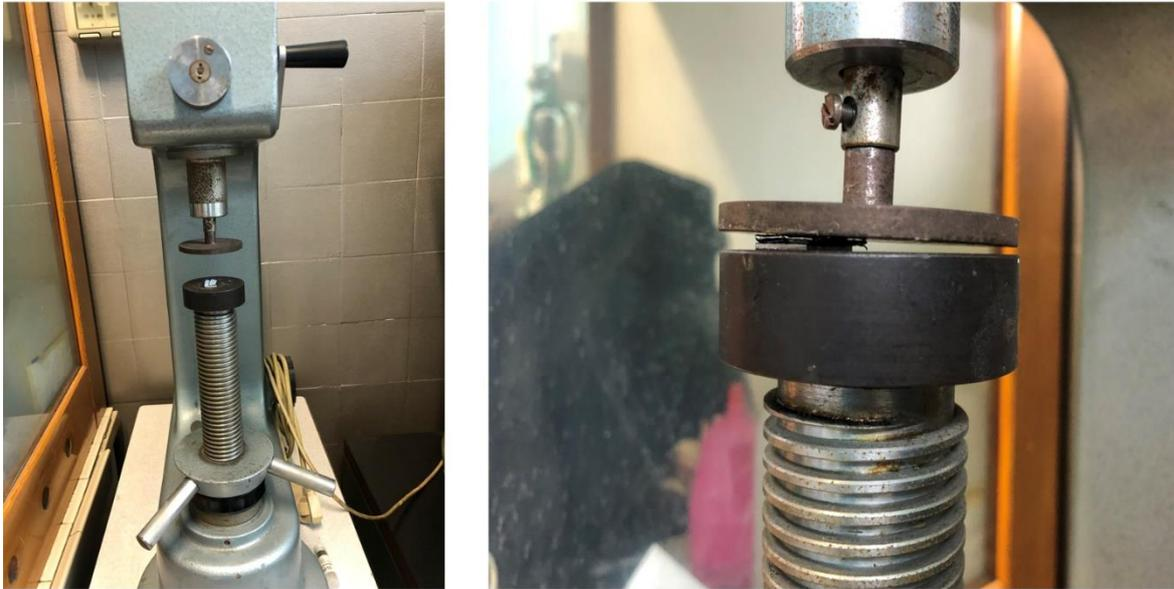
*Figure 107: Mechanical load applied to make Zama chips and sandwich more flat*
