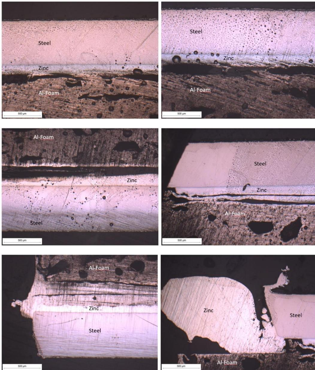
Figure 98: Optical microscope images of the transverse section of the samples of Zn-steel, Al-Foam, Zinc at 50x magnification
