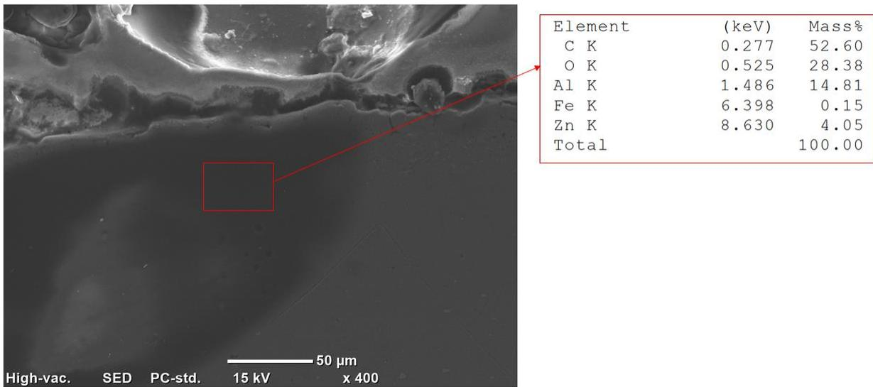
Figure 79: EDS analysis of Al5182, Zn-steel and Zama
