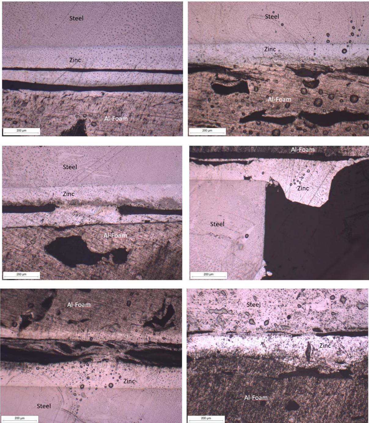
Figure 99: Optical microscope images of the transverse section of the samples of Zn-steel, Al-Foam, Zinc at 100x magnification
