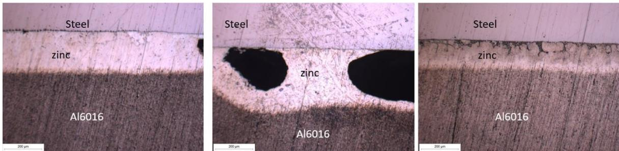
Figure 67: Optical microscope images of the transverse section of the samples of Zn-steel, Al6016 (flux) and Zn at 100x magnification
