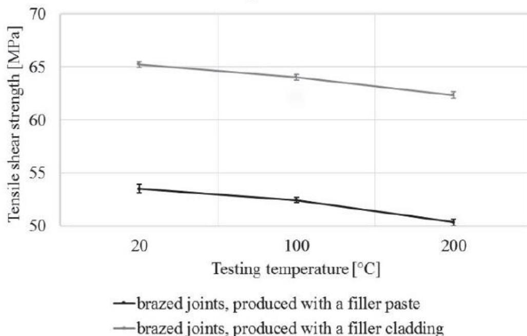
Figure 16: tensile test results of the sample[30]
