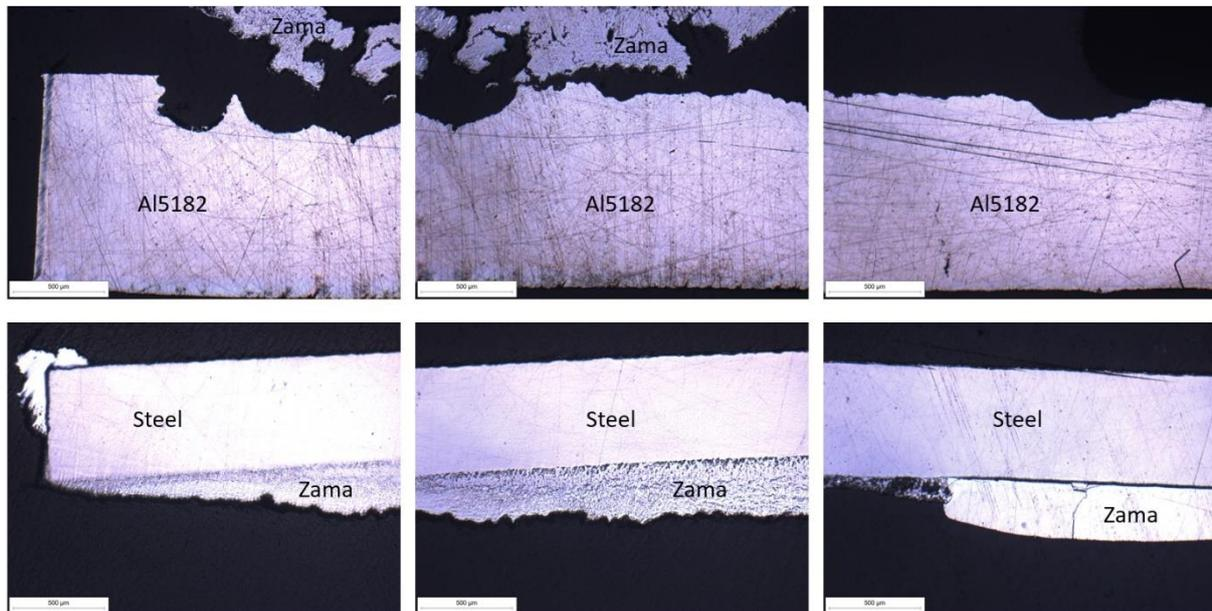
Figure 83: Optical microscope images of the transverse section of the samples of Zn-steel, Al5182, Zama at 50x magnification
