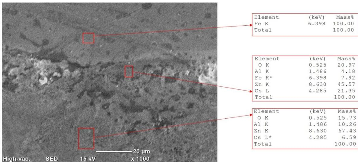
Figure 96: EDS analysis of Al-foam (FLUX), Zn-Steel and Zn at 1000x magnification
