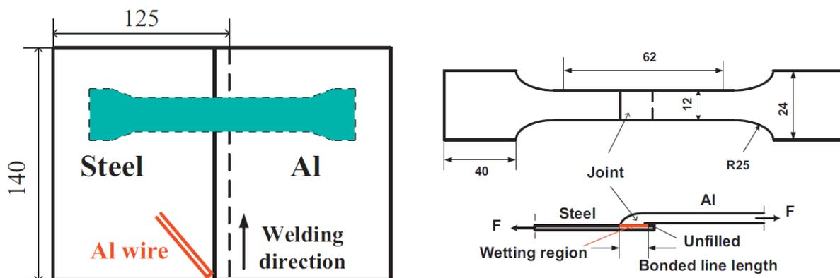
Figure 24: Shape and dimension of sample for lap-shear test [34]
