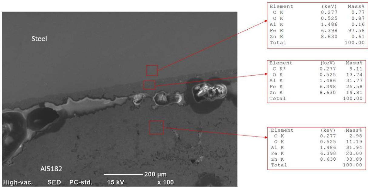
Figure 77: EDS analysis of Al5182, Zn-steel and Zama
