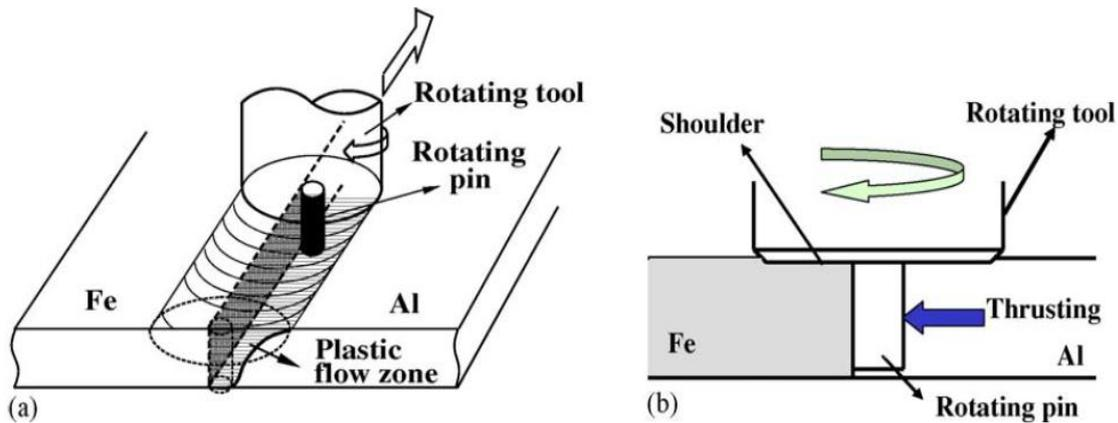
Figure 17: Rotating pin position: (a) birds eye view, (b) cross-section view perpendicular to the weld surface [32]
