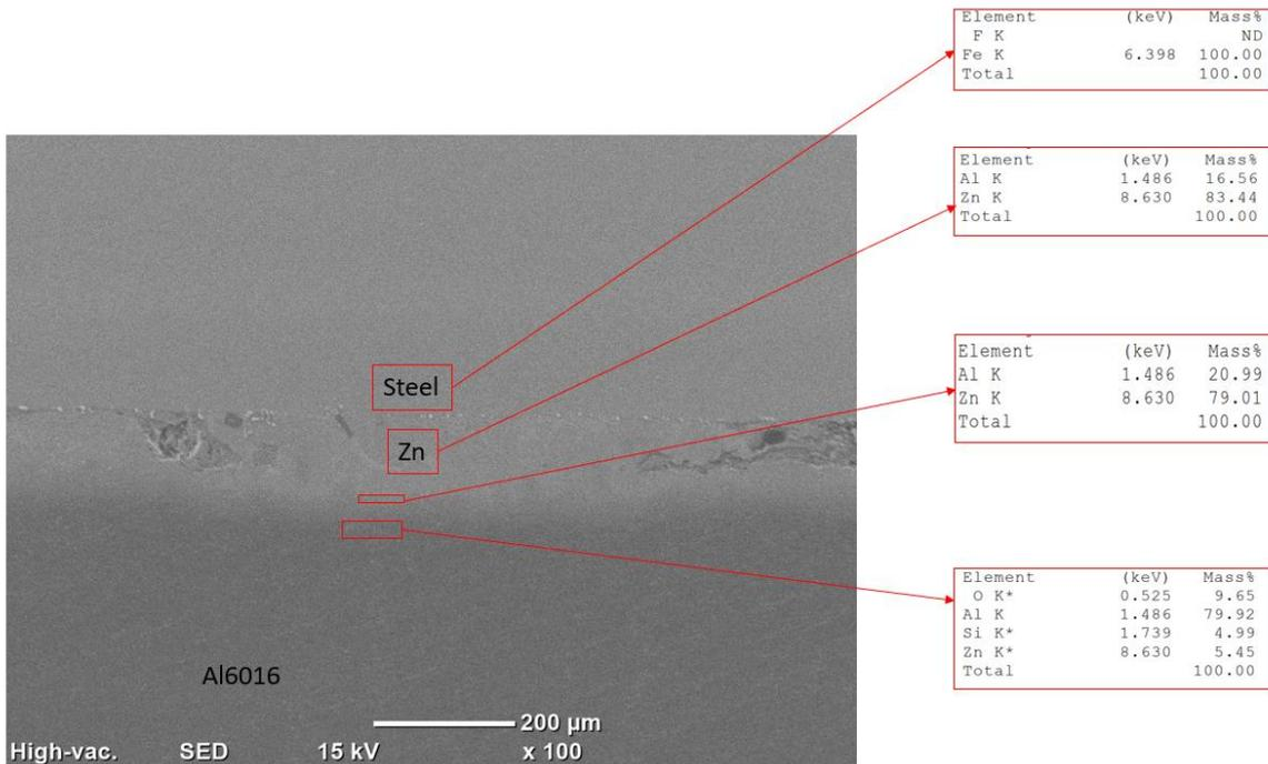
Figure 71: Point analysis using SEM and EDS of Al6016(flux), Zn-steel and Zn at 100x magnification
