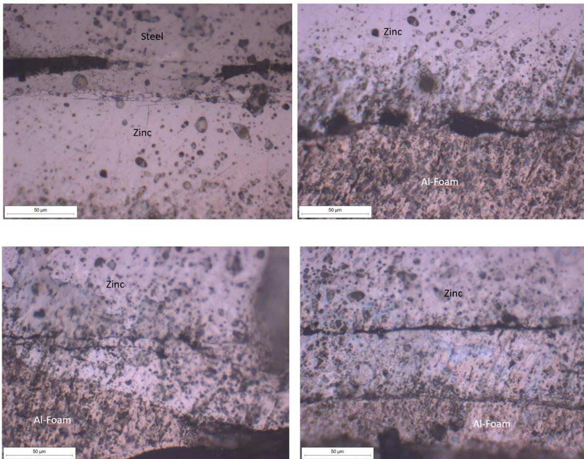
Figure 100: Optical microscope images of the transverse section of the samples of Zn-steel, Al-Foam, Zinc at 200x magnification
