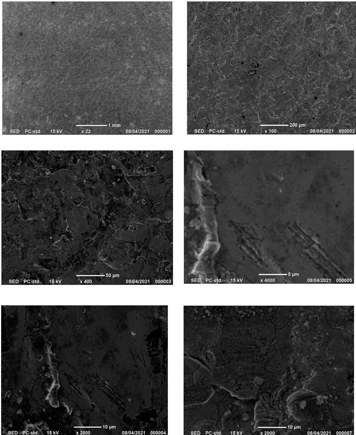
Figure 50: Top of Zn-coated steel at different magnifications using SEM
