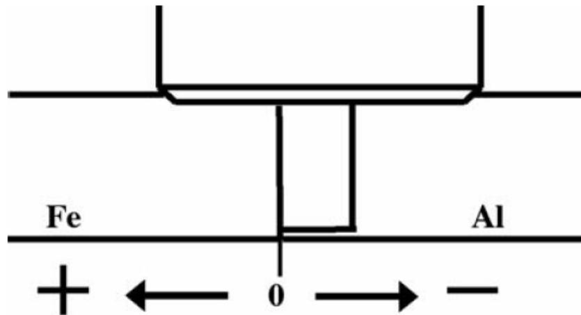
*Figure 19: Offset of the Rotating tool*
