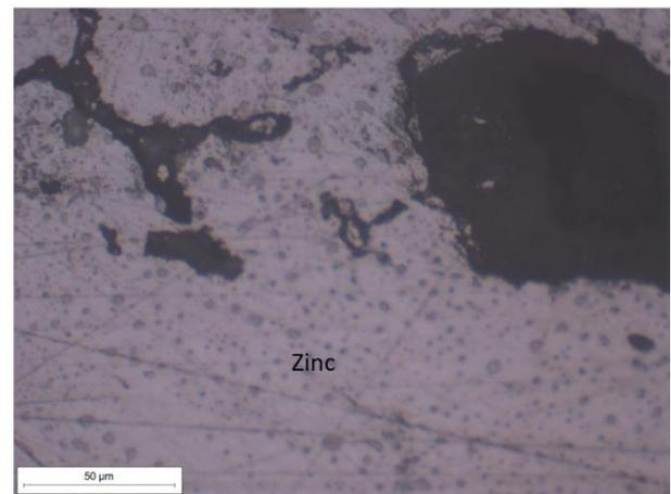
Figure 91: Optical microscope images of the transverse section of the samples of Zn-steel, Al-Foam, Zinc at 500x magnification
