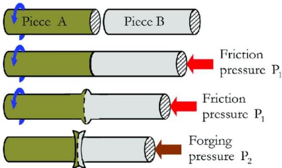
Figure 7: Friction welding schematic[19]
