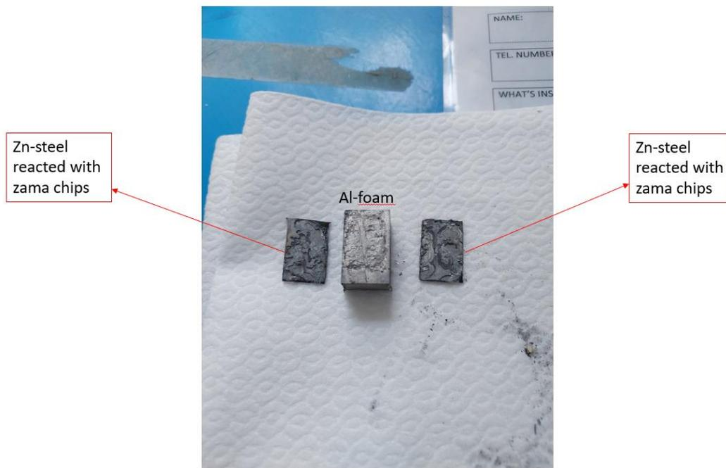
Figure 106: Brazing of Al-foam (flux) and Zn coated steel with Zama as filler
