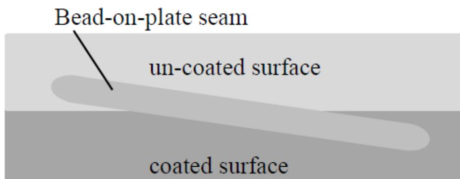
Figure 23: partially coated specimen[33]
