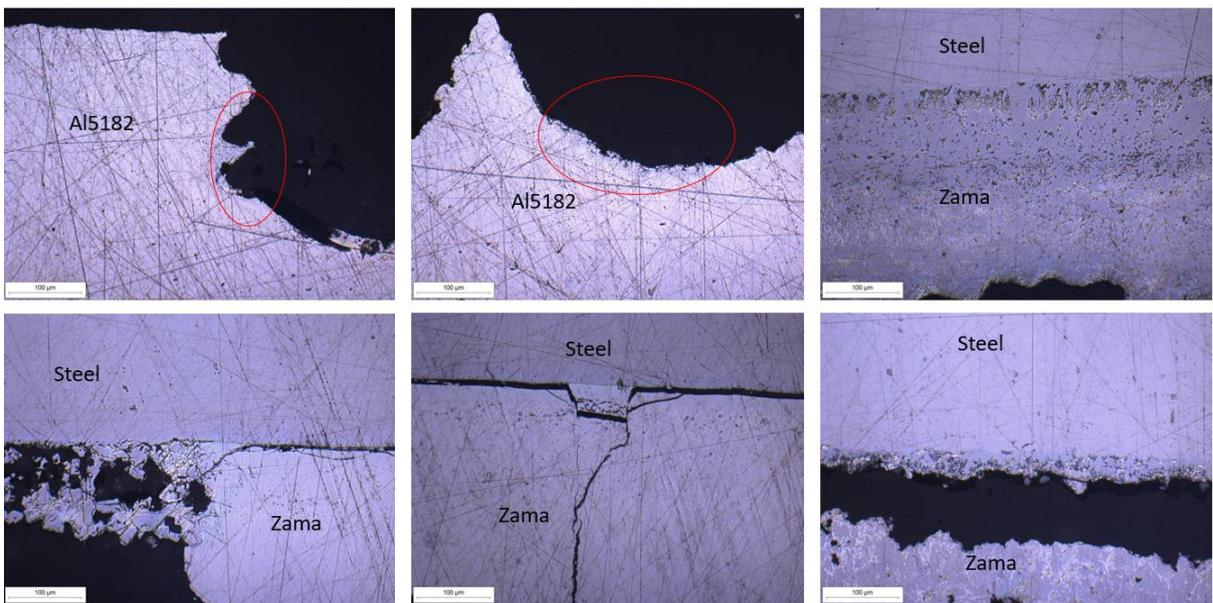
Figure 84: Optical microscope images of the transverse section of the samples of Zn-steel, Al5182, Zama at 200x magnification
