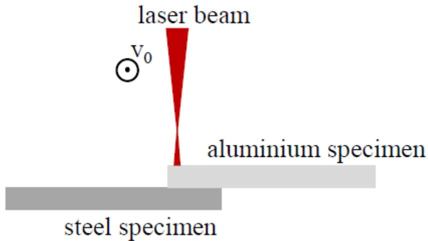
Figure 22: setup for laser beam overlap welding [33]
