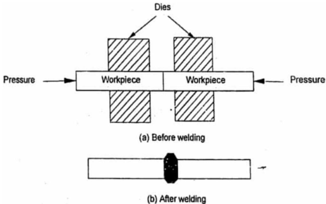
Figure 8: schematic for cold welding
