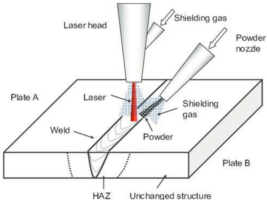
Figure 4: Laser Beam Welding
