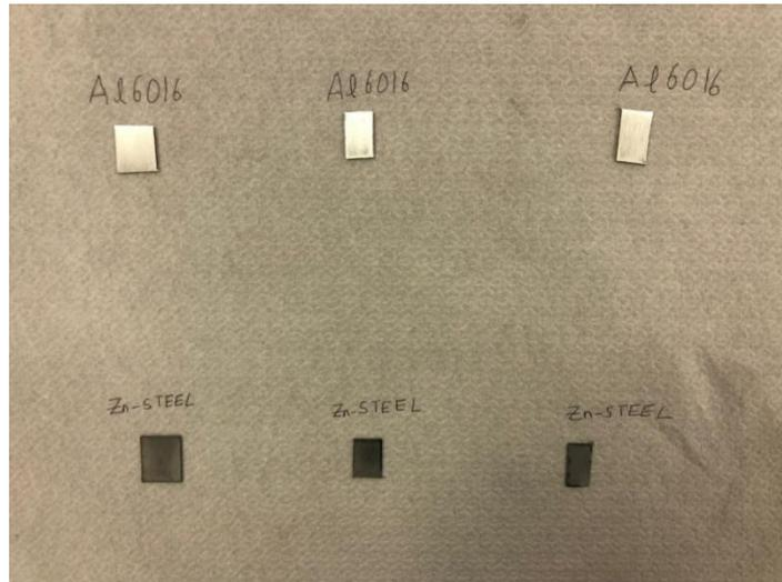
*Figure 32 samples after preparation with abrasive paper*
