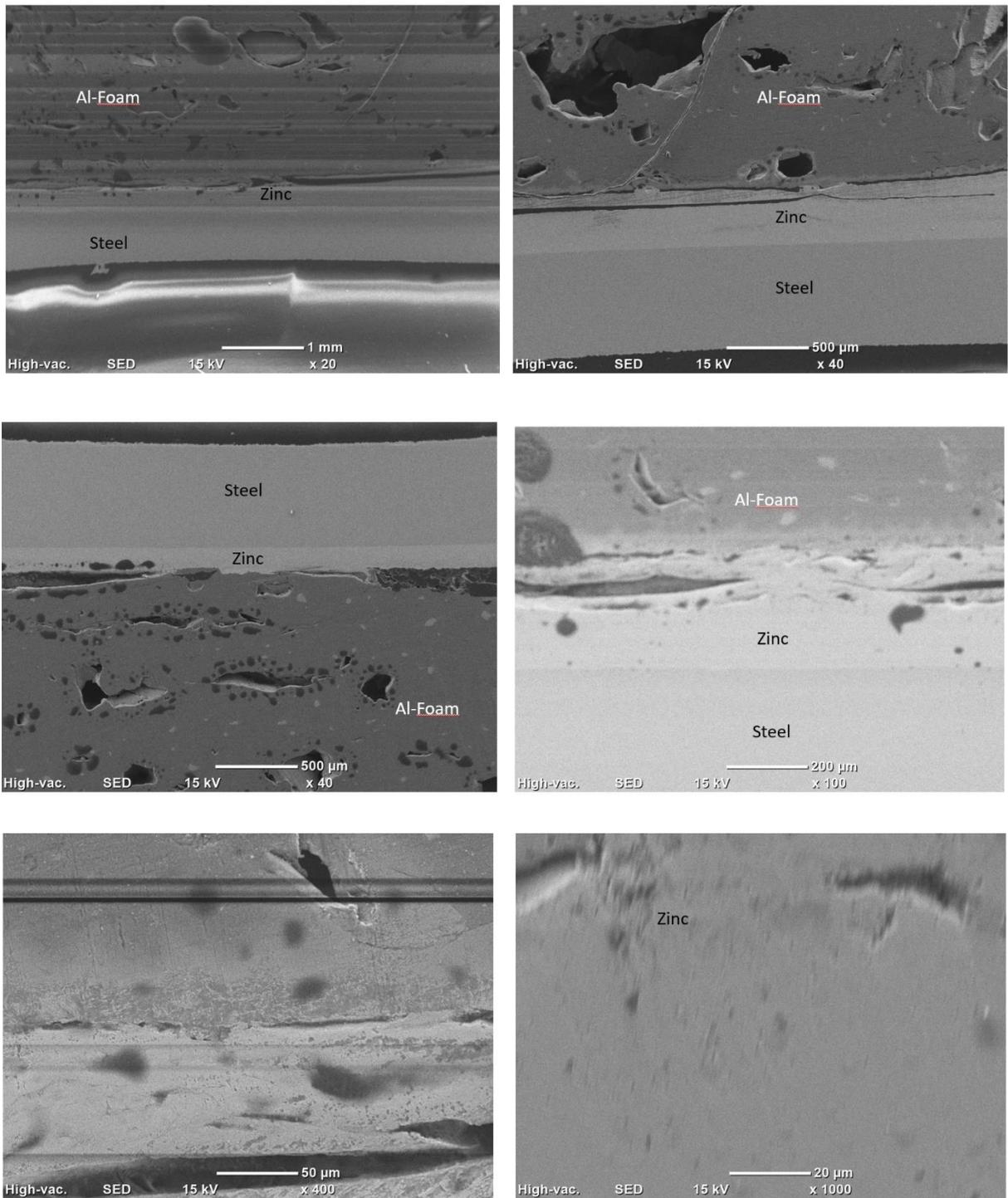
Figure 101: SEM images of the transverse section of the samples of Zn-steel, Al-Foam, Zinc at 20x, 40x, 100x, 400x, 1000x
