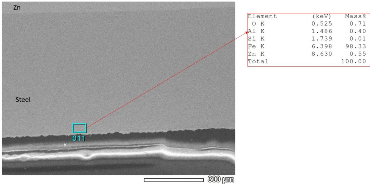
Figure 104: EDS analysis of Al-Foam, Zn-steel, and Zinc at 100x magnification
