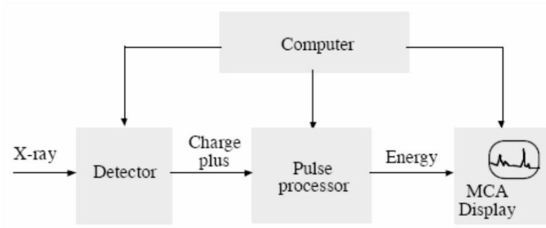
Figure 49: X-Ray Spectral Measurement[48]
