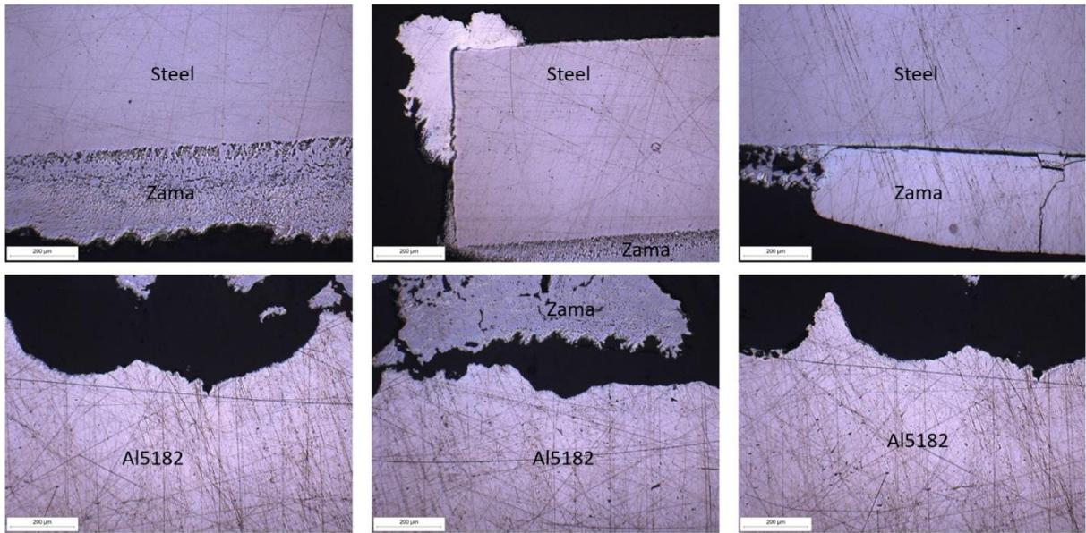
Figure 85: Optical microscope images of the transverse section of the samples of Zn-steel, Al5182, Zama at 100x magnification
