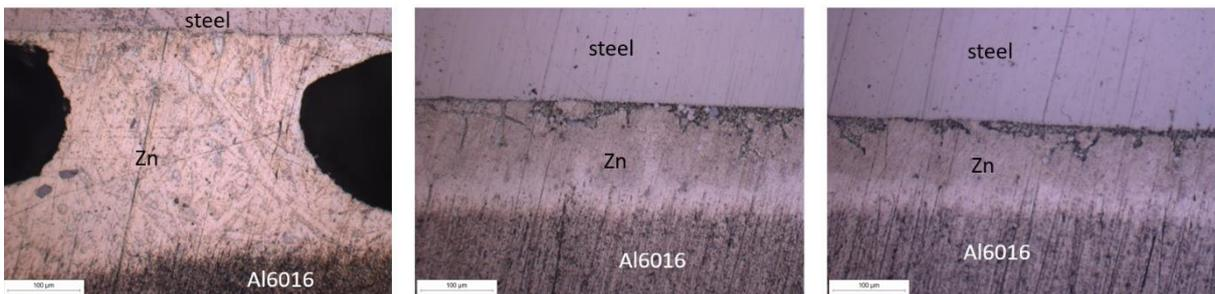
Figure 68: Optical microscope images of the transverse section of the samples of Zn-steel, Al6016 (flux) and Zn at 200x magnification
