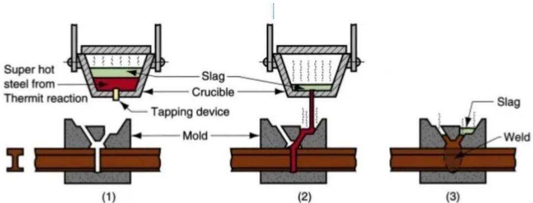
Figure 6: Use of Thermit Welding
