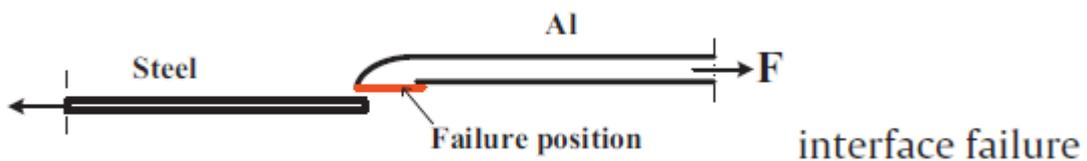
Figure 25: Depiction of failure mode[34]
