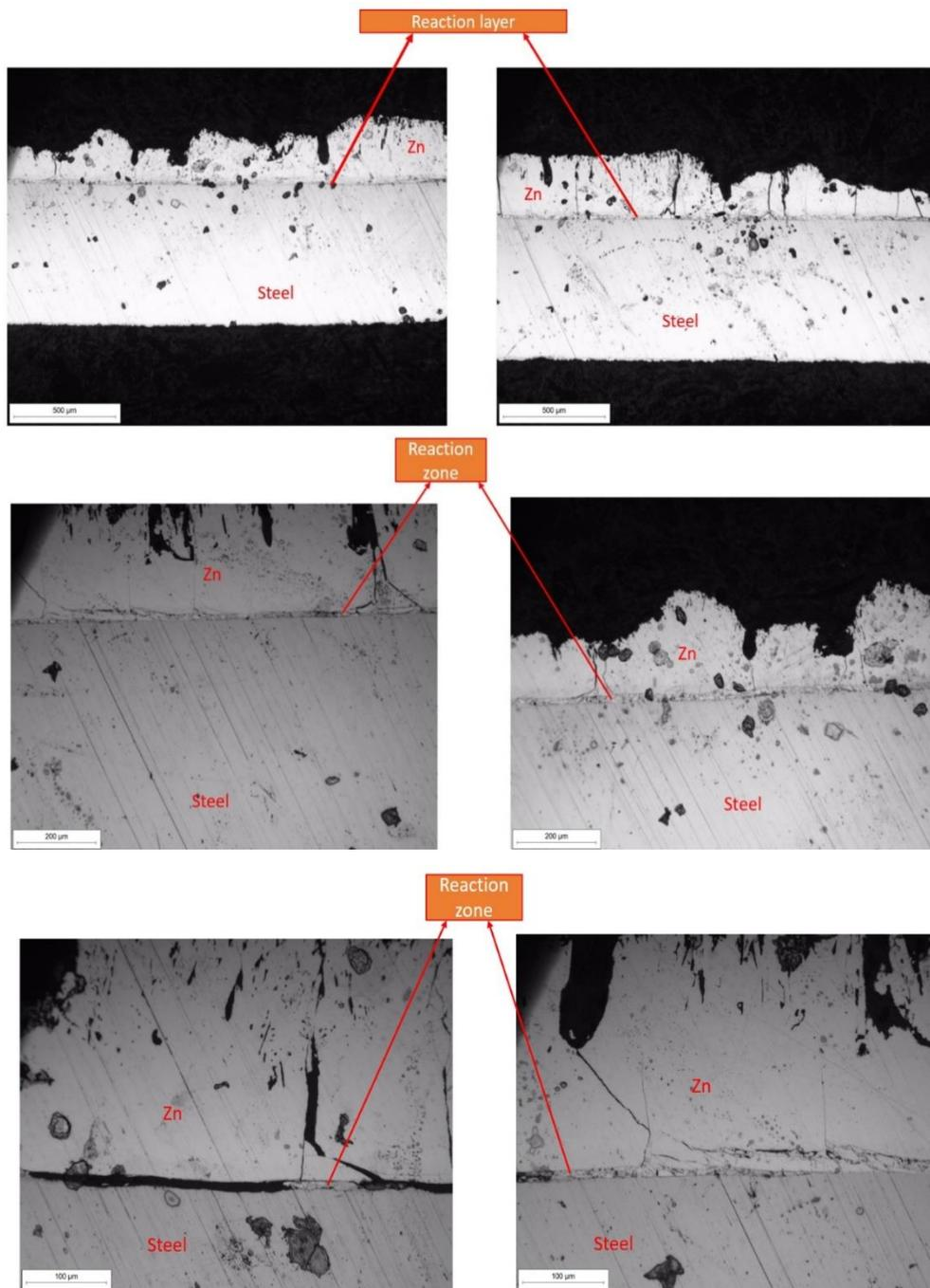
Figure 59: Optical microscope images of the transverse section of the samples of Zn-steel and Zn at different magnifications
