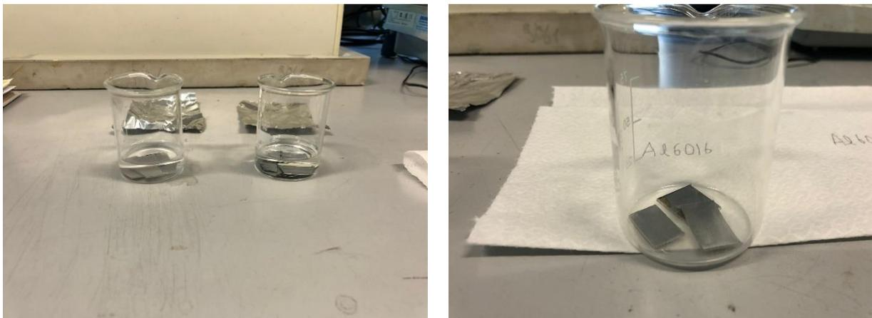
*Figure 34: (a) samples dipped in ethanol solution (b) Aluminum Alloy cleaned in ethanol solution*
