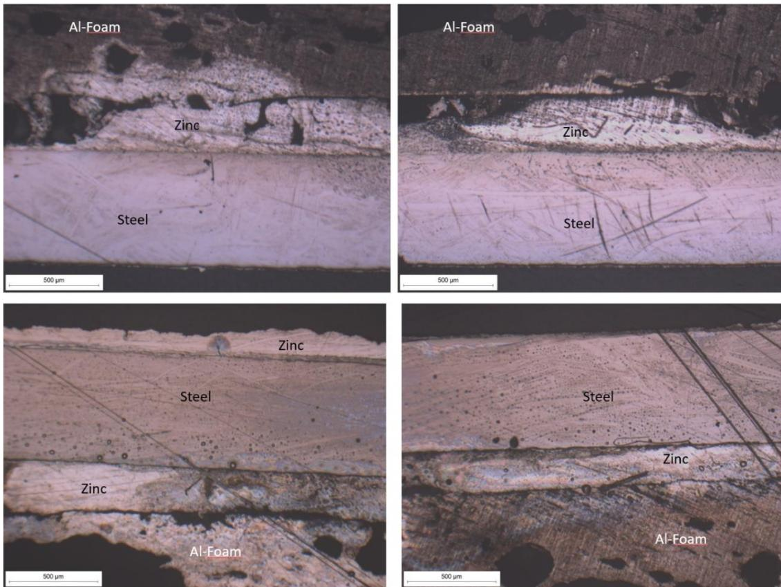
Figure 88: Optical microscope images of the transverse section of the samples of Zn-steel, Al-Foam, Zinc at 50x magnification
