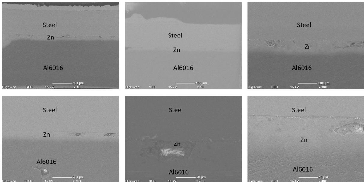
Figure 70: SEM images for Al6016(flux), Zn-coated Steel and Zn at 40x, 100x, 200x, 400x
