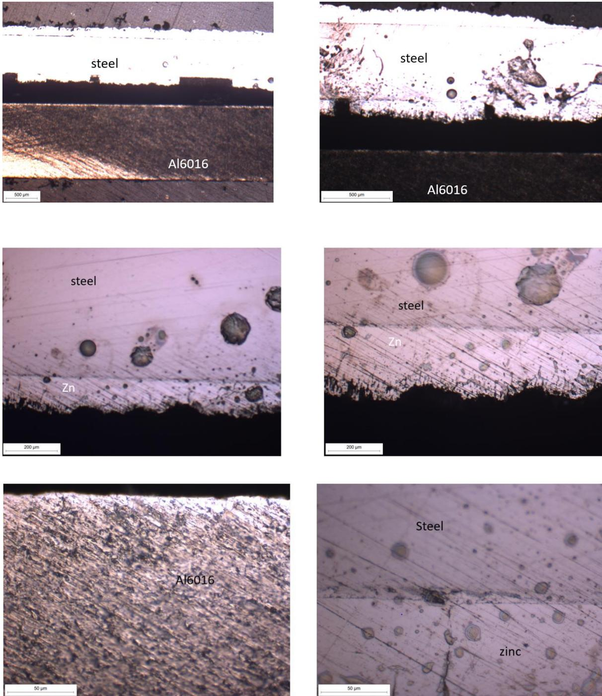
Figure 64: Optical microscope images of the transverse section of the samples of Zn-steel, Al6016 (no flux) and Zn at different magnifications
