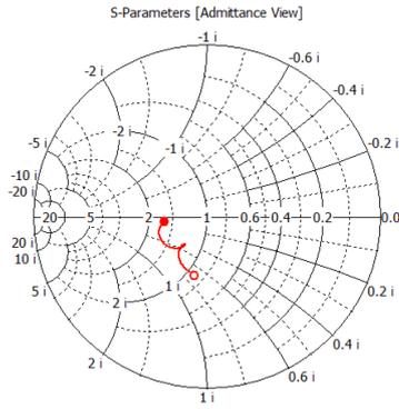
Figure 4.22: Z smith chart of optimised antenna at 2.45 GHz
