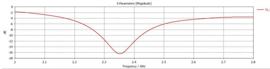
Figure 4.7: Simulated S11 of the patch antenna
