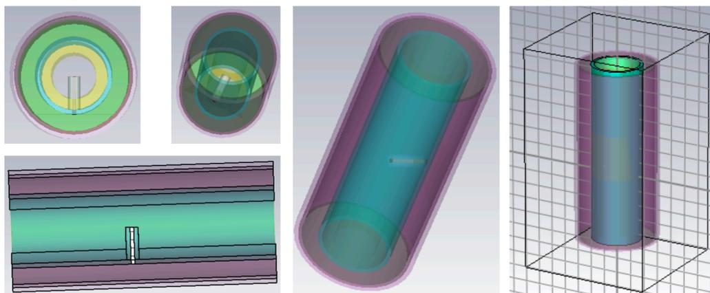
Figure 4.20: different views of Cylindrical patch antenna
