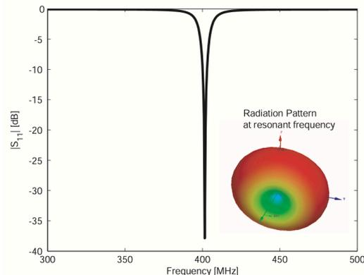
Figure 2.3 Matching Performance and 3D radiation pattern of the final structure considering a free space environment [18]
