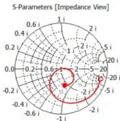
Figure 4.17 : Z smith chart of optimised antenna at 2.45 GHz
