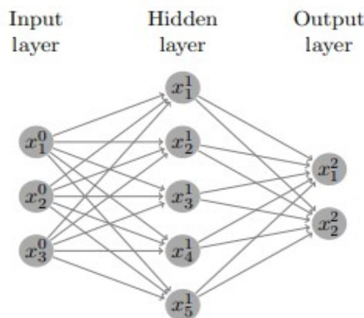
Figure 3.1: Deep Feedforward Neural Network with 3 layers.
