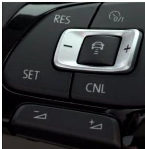
**Figure 5.2:** ACC controller in steering wheel
