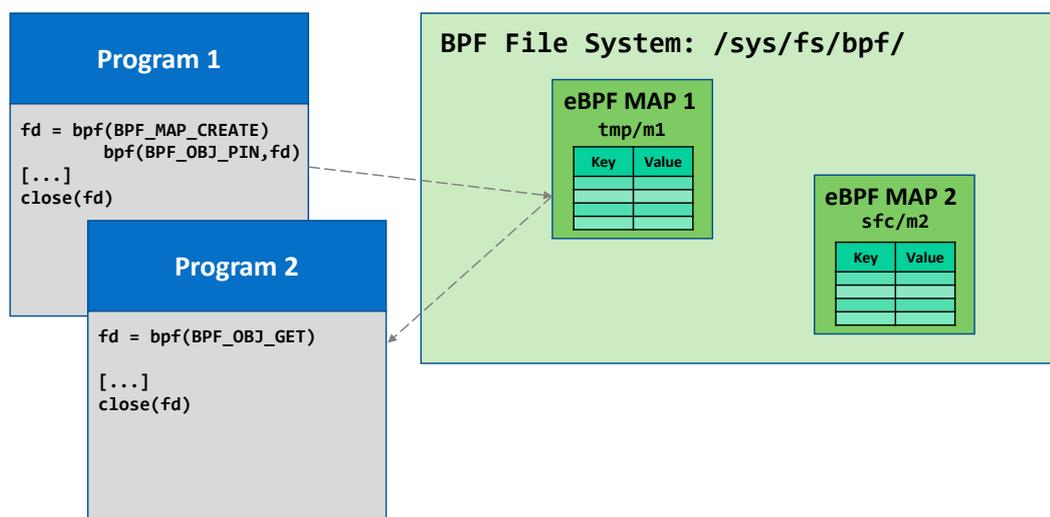
**Figure 3.2:** An example of object pinning on BPF file system.
