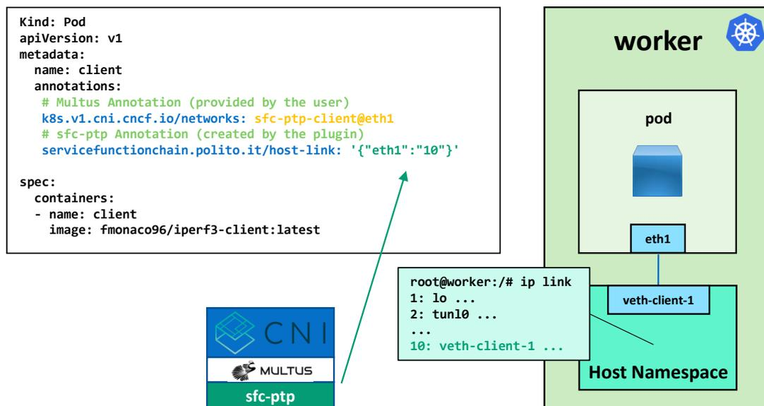
Figure 5.2: Host-link annotation configured in a Pod resource.
