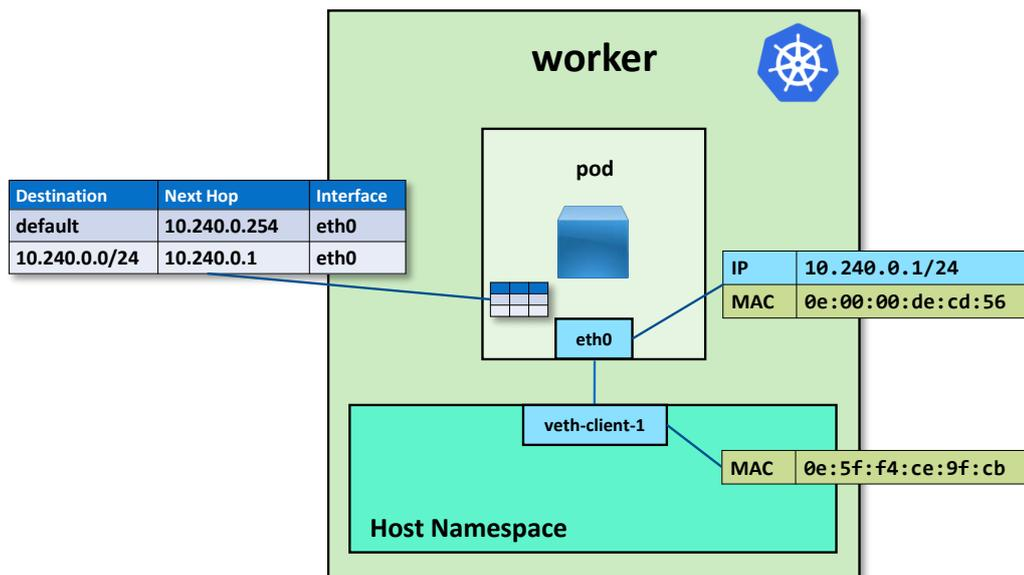
**Figure 5.1:** Pod connected with host through a veth pair created by *sfc-ptp*.
