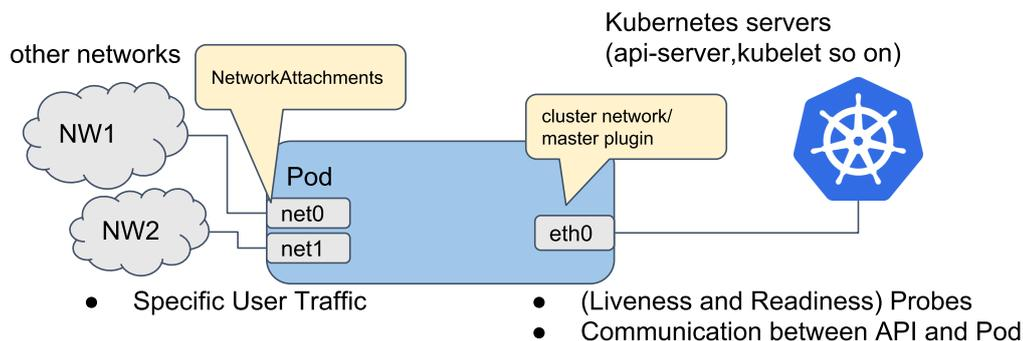
**Figure 3.3:** A pod with multiple attached interfaces [16].
