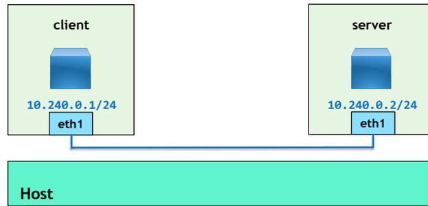
Figure 6.1: Client-Server connected through a veth pair.
