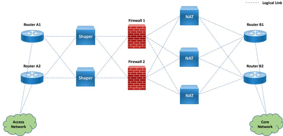
**Figure 1.2:** A possible scaled Service Function Chain.
