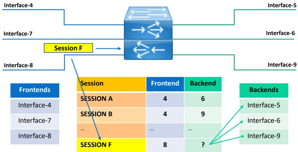
**Figure 4.3:** A load balancer receiving a packet for a new session.
