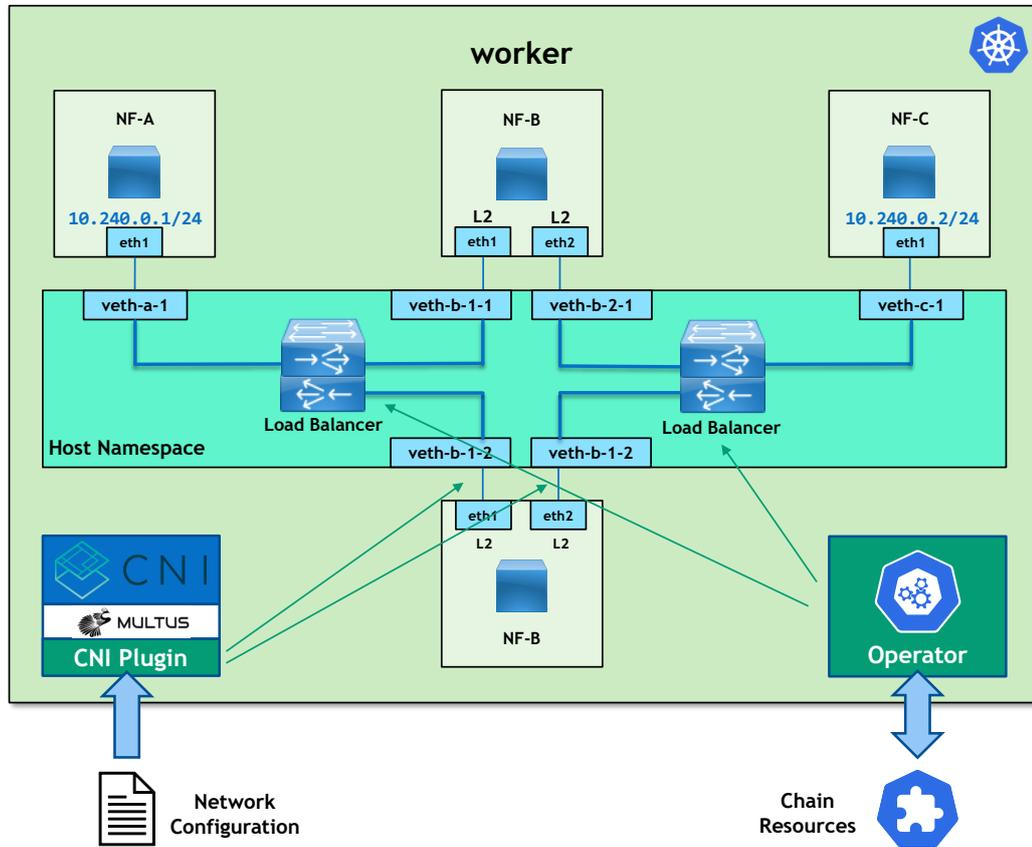
Figure 4.1: System components on a Kubernetes node.
