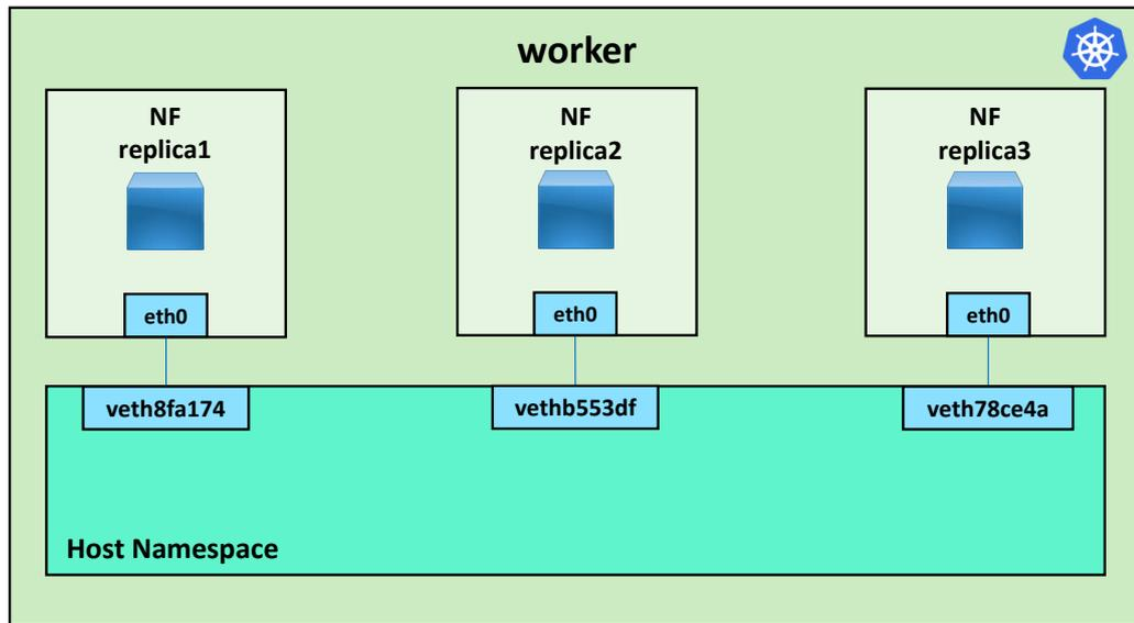
Figure 5.3: Veth interfaces with arbitrary names on the host side.
