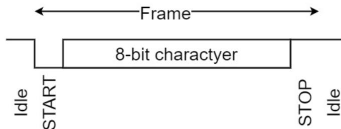
Figure 3.3: UART frame structure
