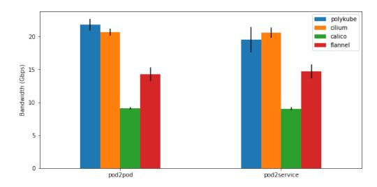
Figure 5.5: Different nodes throughput comparison for TCP traffic
