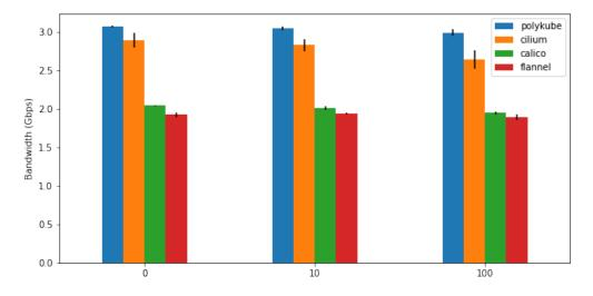
Figure 5.4: Same node throughput comparison for UDP traffic with an increasing number of Services/Pods
