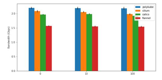
Figure 5.8: Different nodes throughput comparison for UDP traffic with an increasing number of Services/Pods  $\,$
