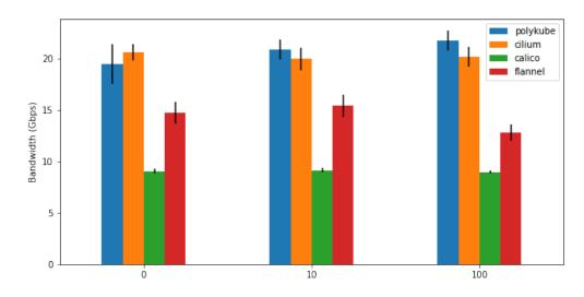
**Figure 5.6:** Different nodes throughput comparison for TCP traffic with an increasing number of Services/Pods
