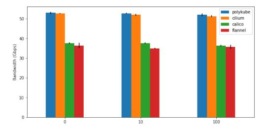
Figure 5.2: Same node throughput comparison for TCP traffic with an increasing number of Services/Pods
