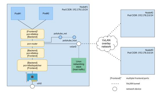
**Figure 3.4:** The new architecture virtual network topology
