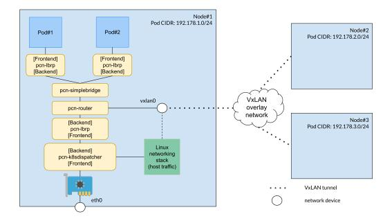
Figure 3.1: The base architecture virtual network topology
