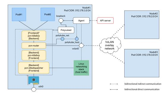
Figure 3.5: Network provider architecture
