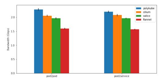
Figure 5.7: Different nodes throughput comparison for UDP traffic
