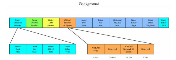
Figure 2.9: The VxLAN packet structure
