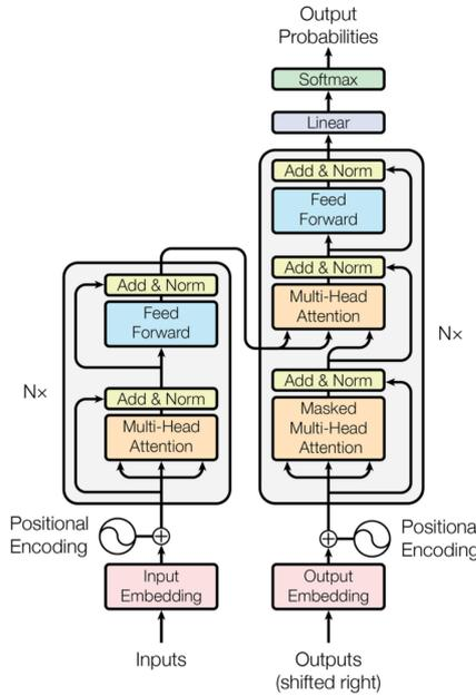
**Figure 4.7:** Attention mechanism representation
