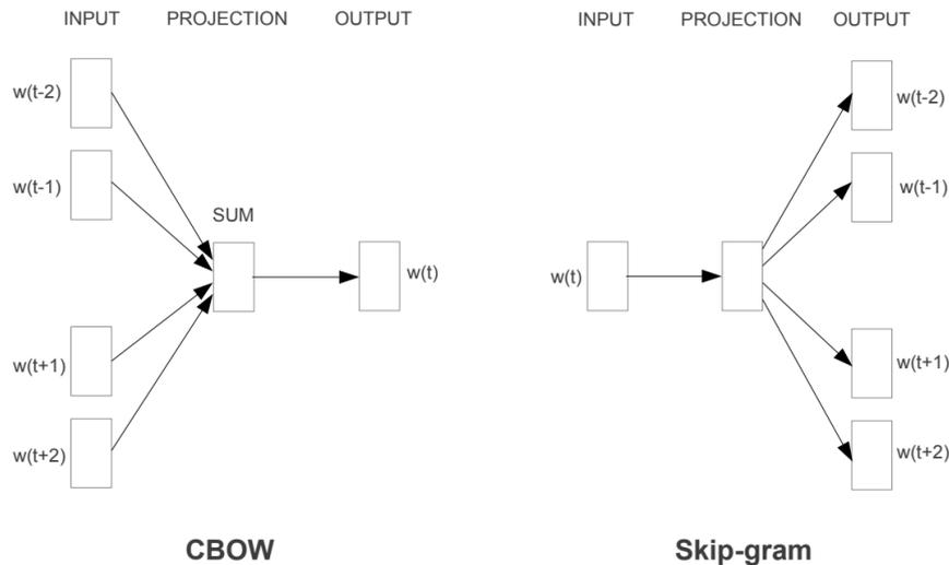
**Figure 4.6:** Word2Vec Continuous Bag of Word and Skip Gram architecture
