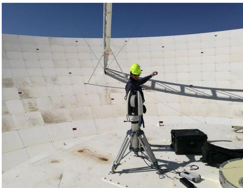
*Figura 4.3 – Sardinia Radio Telescope, Laser Tracker Leica AT960 LR, Axist*
