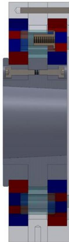
Figure 3.43 – Internal position of the carrier for neutral gear
