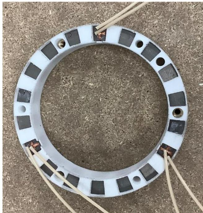
Figure 2.3 – Photo of the carrier with the ferromagnetic pole-pieces inside the resin structure and with winding attached for magnetic flux evaluation.
