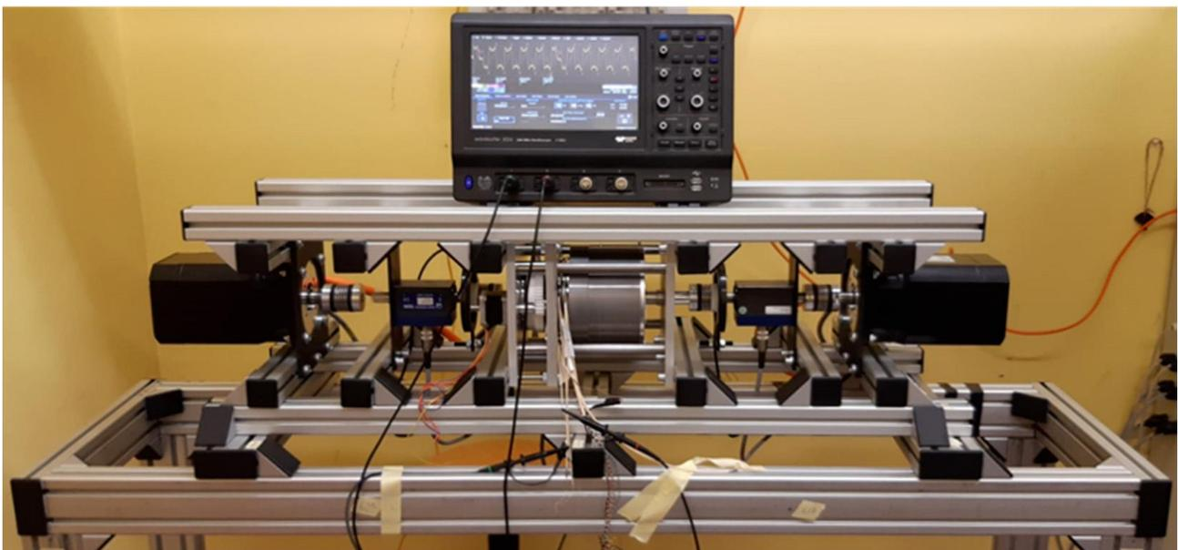
Figure 2.10 – focus on the active part of the test bench while magnetic fluxes are being sampled with an oscilloscope.
