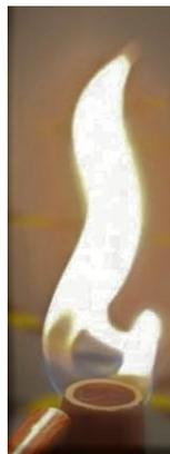
*Figure 3.2. Detail of the flame 'pierced' by the laminar air jet.*
