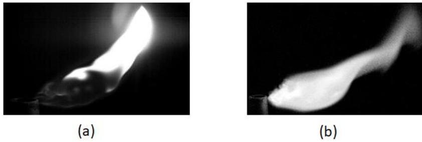
Figure 1.10. No-Lifted flame (a), Lifted flame (b).
