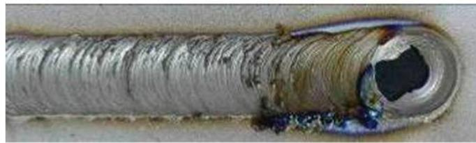
**(a) Overheating and tool penetration defect**
