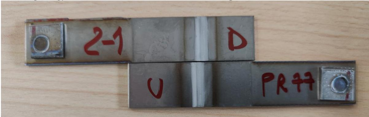
Figure 4.10 Specimen 1 after the tensile test.
