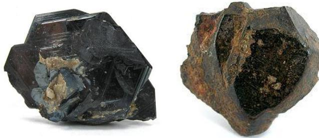
Figure 1.12 On the left a photograph of rutile, on the right a photograph of ilmenite[16], [17].
