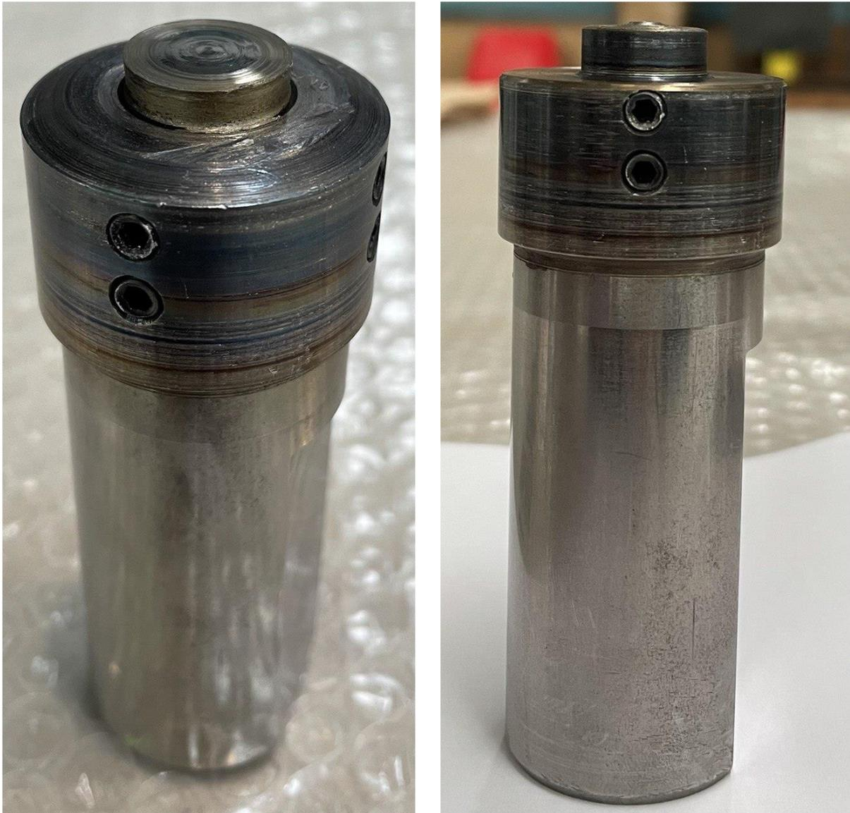
*Figure 4.6 Pictures of the worn tool after welding a joint.*
