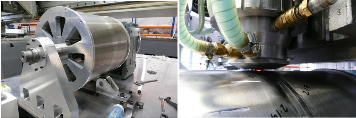
Figure 2.43 On the left the support of the circumferential FSW, on the right welding underway on the cylinder-cylinder[34].
