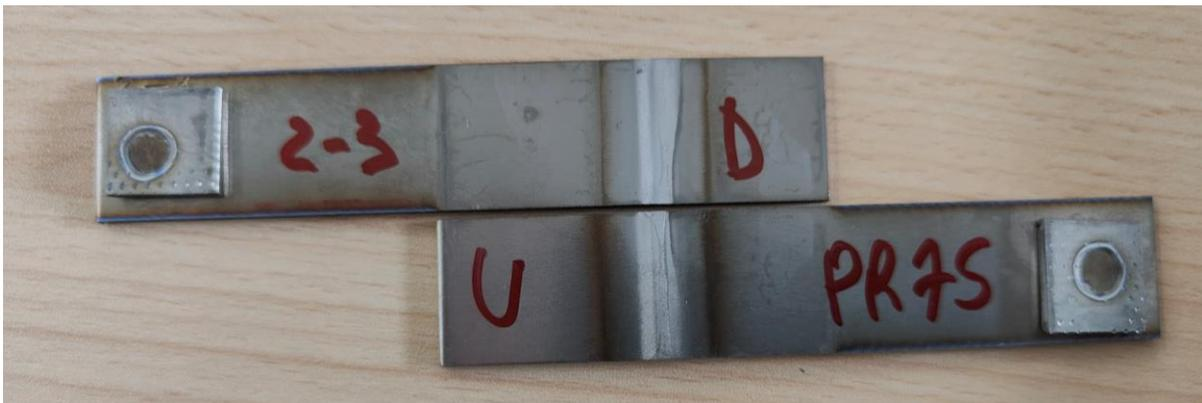
Figure 4.12 Specimen 3 after the tensile test.
