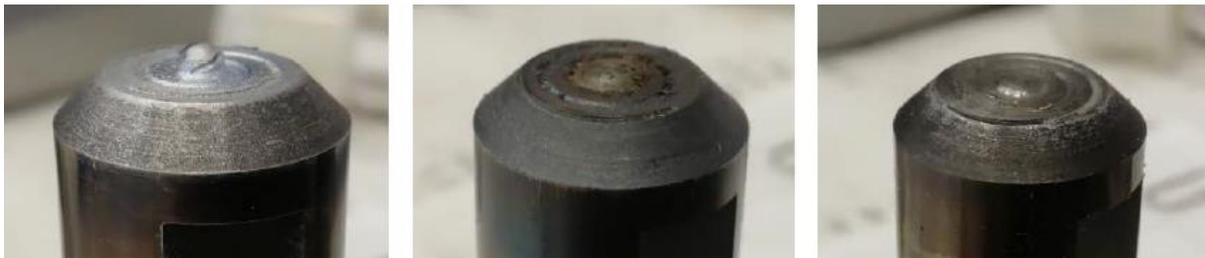
Figure 2.23 The destruction of the pin of the tool from 4H5MFS steel[29].
