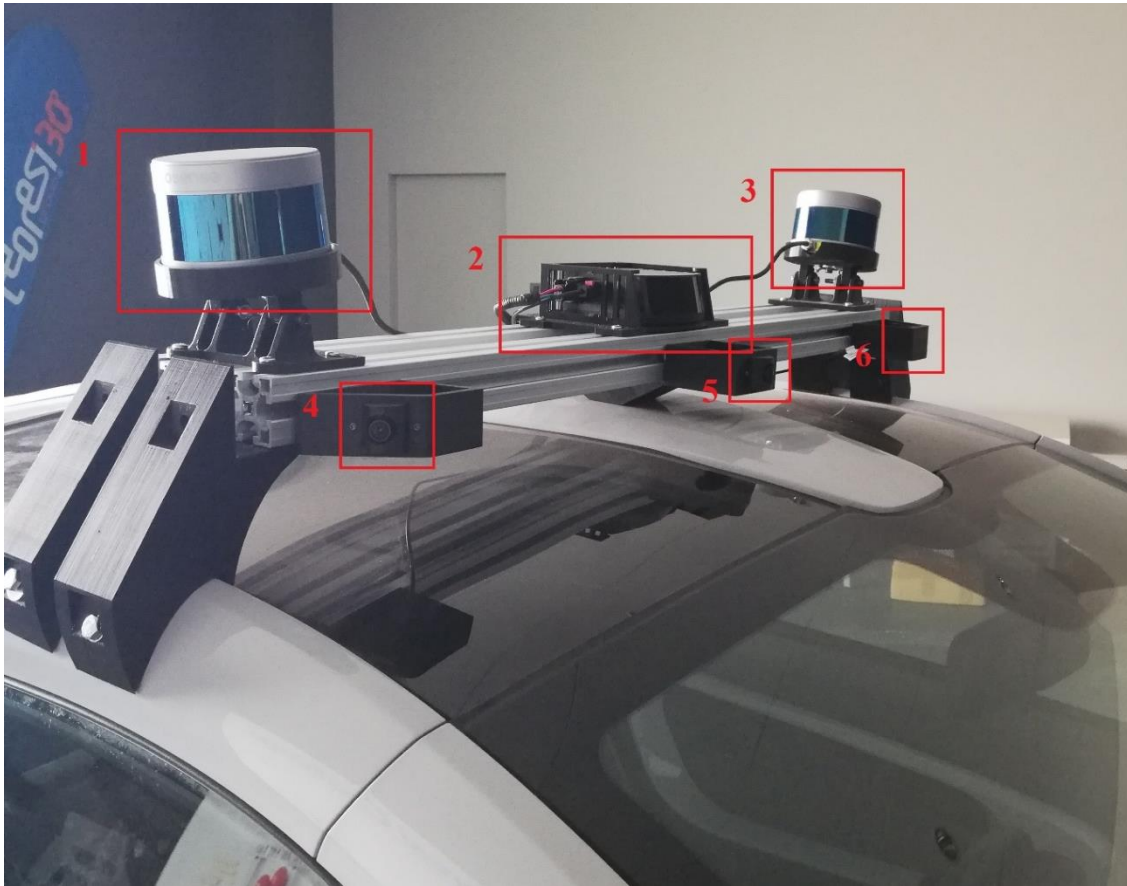
Figure 59. Detail of LiDARs and cameras
