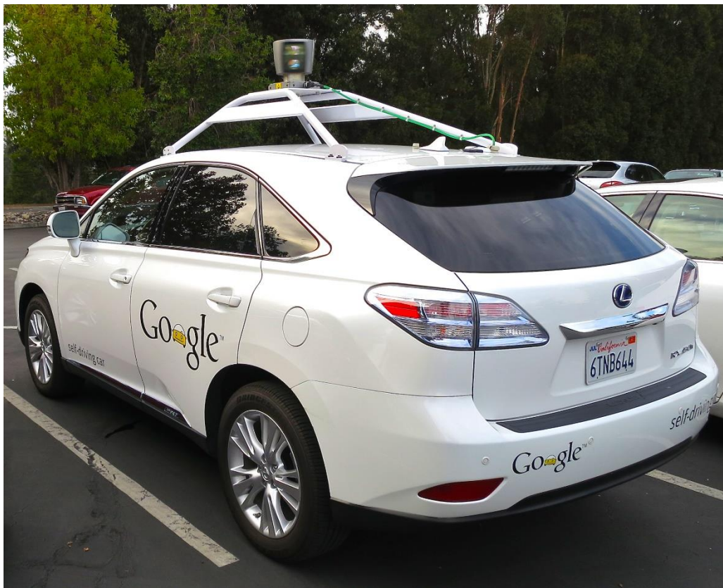
Figure 8. Lexus RX450h modified from Google for testing
