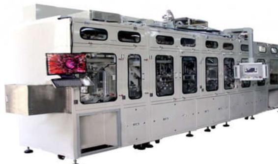
Figura 2.27 - Auto electrolyte filling machine (TMAX BATTERY EQUIPMENTS)
