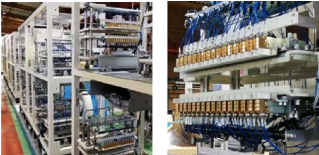
*Figura 2.28 - Automatic formation machine (Nabertherm)*
