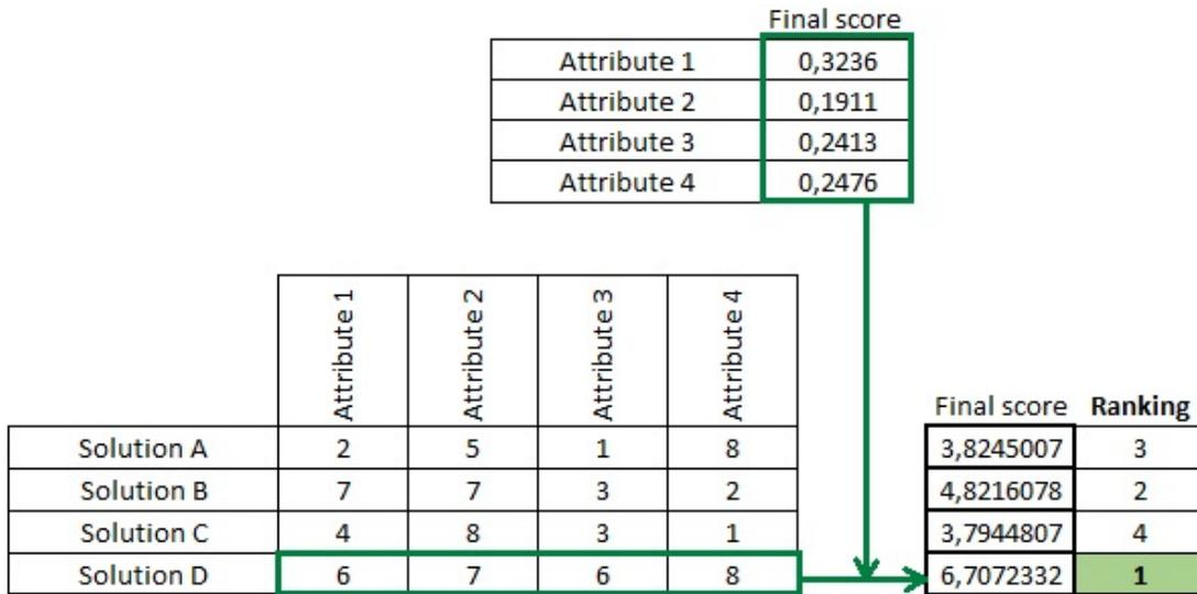
Figure 2.3. AHP Computational Procedure: solution choice
