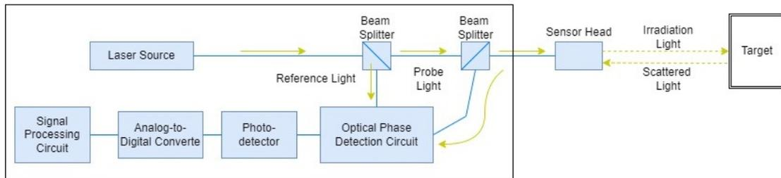
Figure 1.16. General configuration of Laser Doppler Vibrometer
