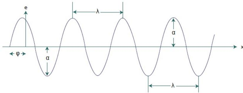
Figure 1.2. Electromagnetic radiation: characteristics of a wave
