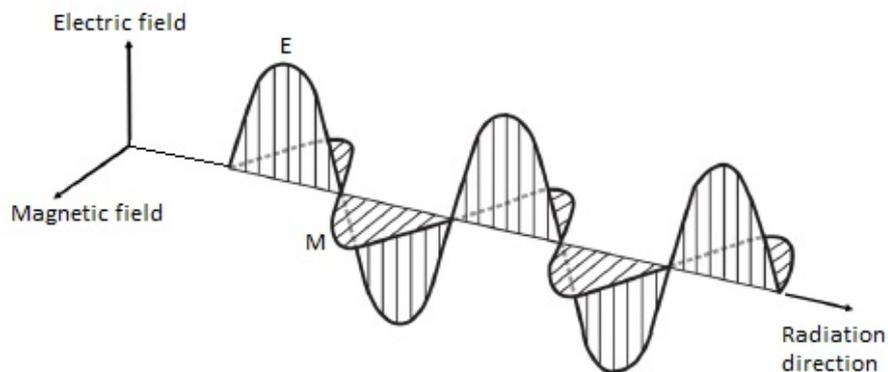
Figure 1.1. Electromagnetic radiation: two oscillation components
