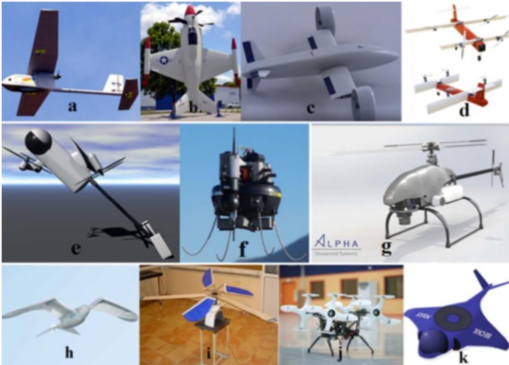
Figure 4.5. Different types of  $\mu$ UAVs, (a) HTOL, (b) VTOL, (c) tilt-rotor, (d) tilt-wing, (e) tilt-body, (f) ducted fan  $\mu$ UAV, (g) helicopter, (h) ornithopter, (i) ornicopter, (j) cyclocopter, and (k) unconventional  $\mu$ UAV [20]
