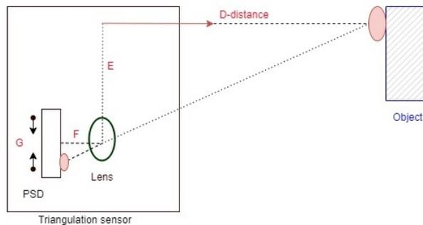
Figure 1.10. Optical triangulation sensor
