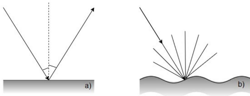
Figure 1.7. Specular a) and Diffuse b) reflection
