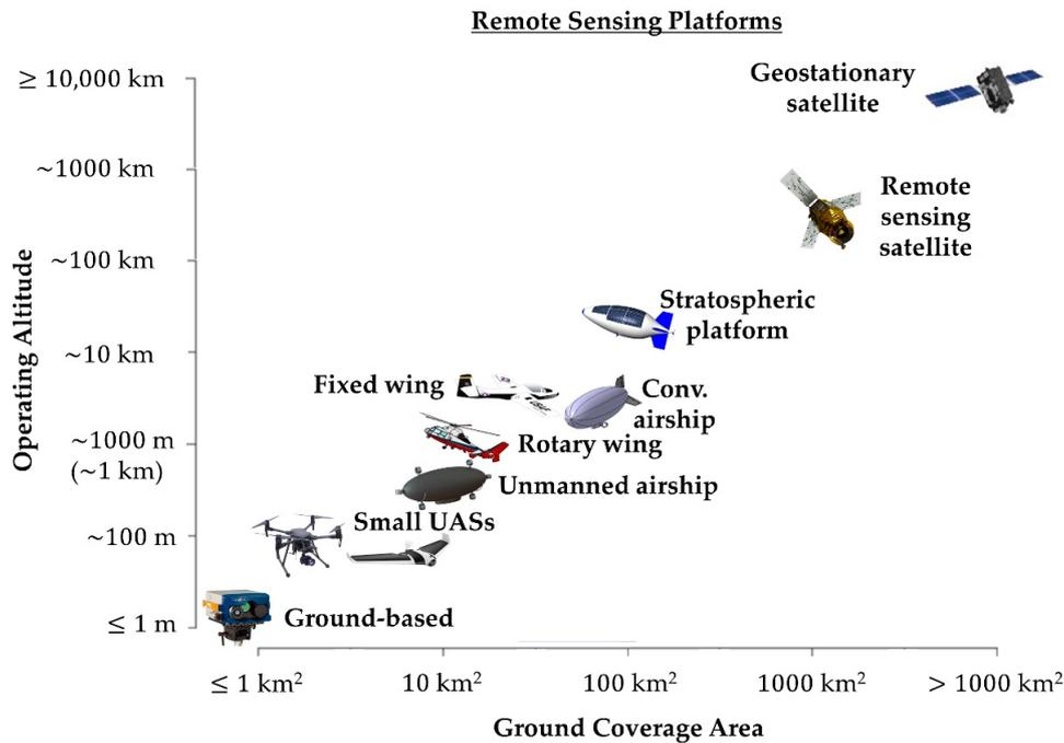
Figure 3.1. Remote Sensing Platforms [15]
