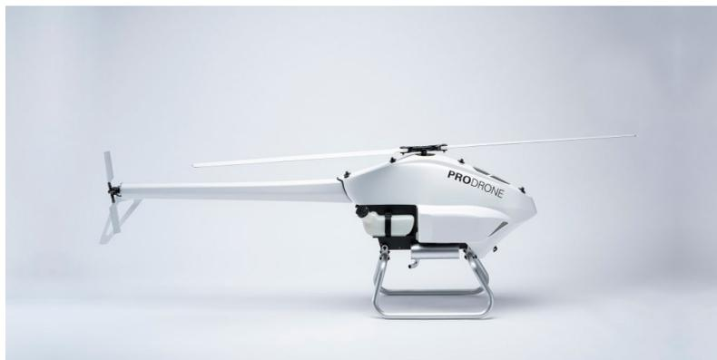
Figure 4.3. An example of single-rotor drone. Credits: [www.prodrone.com](http://www.prodrone.com)
