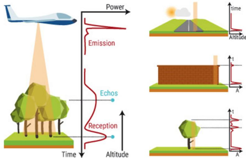
Figure 1.14. LiDAR on UAV. Credits: [www.yellowscan-lidar.com](http://www.yellowscan-lidar.com)
