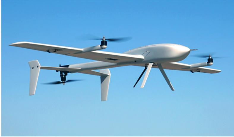
Figure 4.4. An example of hybrid drone. Credits: [www.technosysind.com](http://www.technosysind.com)
