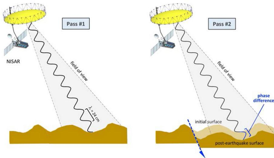
Figure 1.13. InSAR surface deformation measurements. Credit: NASA.
