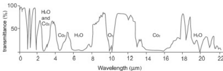
Figure 1.6. Atmospheric transmittance [2]
