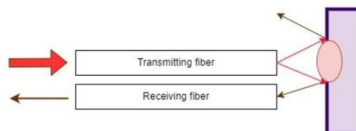
Figure 1.9. An example of fiber optical intensity sensor for distance measurements
