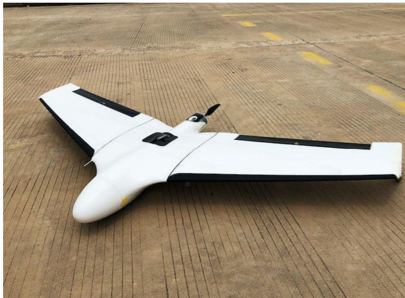
Figure 4.2. An example of fixed-wing drone. Credits: [www.uavgl.com](http://www.uavgl.com)
