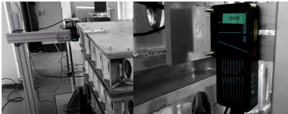
**Figure 3.10:** ODS measuring the sloshing table's motion along the x-axis
