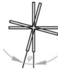
Figure 10. Pure torsional instability.
