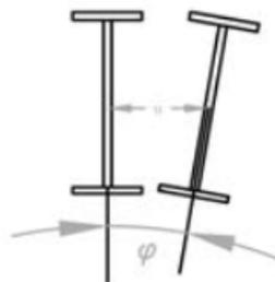
Figure 11. Lateral-torsional instability.
