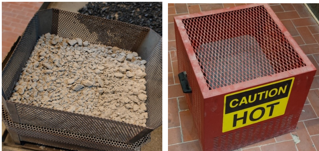
Figure 51 Sample distribution inside the basket and sample cooling
