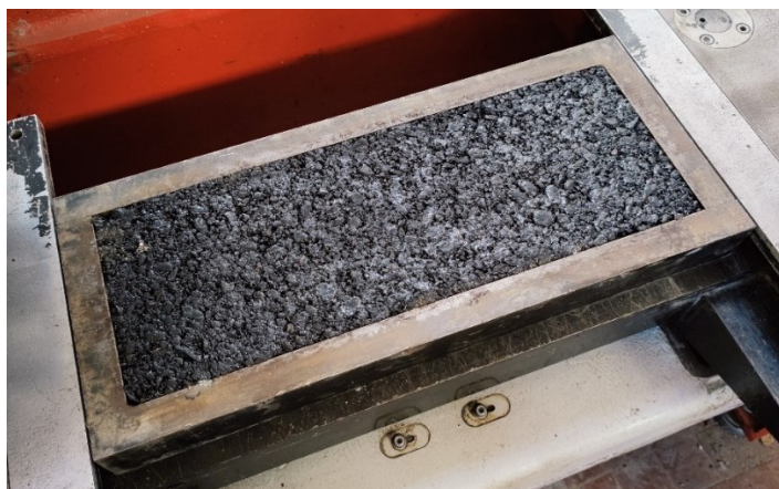
Figure 66 The compacted slab
