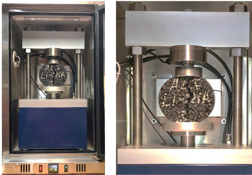
Figure 35 Testing Diametral Specimens to Failure in Accordance with the iRLPD
