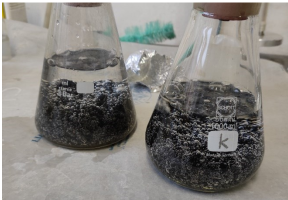
Figure 48 Asphalt particles inside the pycnometer
