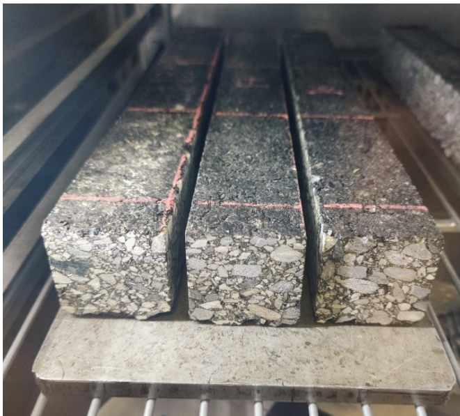
Figure 23 Four point bending beams
