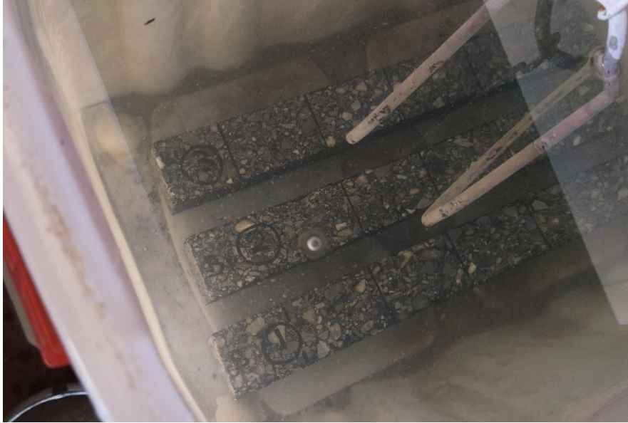
Figure 69 The 4PB beams inside the water path
