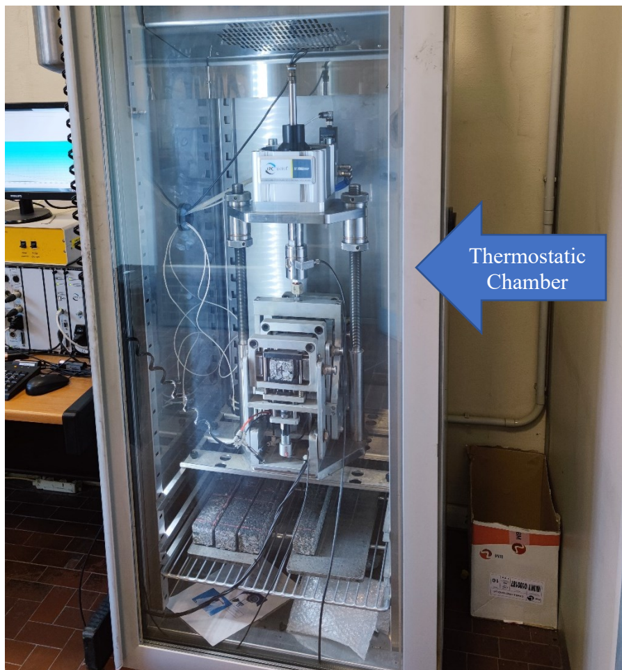
Figure 20 Four point bending machine with thermostatic chamber
