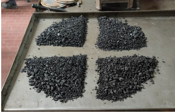
Figure 47 Mixture disaggregation after cooled down
