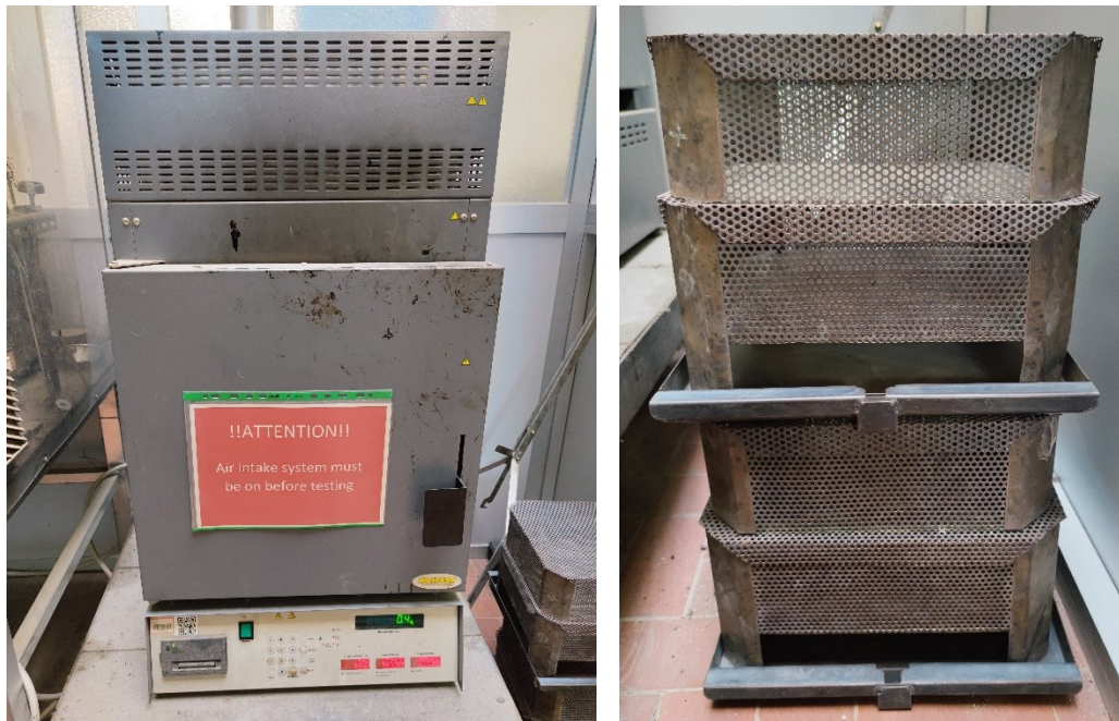
Figure 50 Ignition test furnace and the sample baskets
