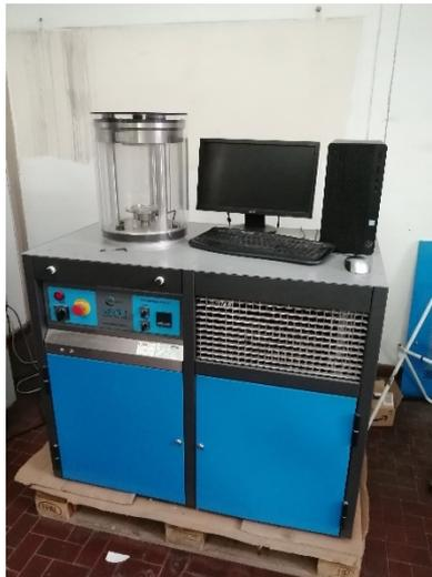
*Figura 3.13 Asphalt Mixture Performance Tester (AMPT)*
