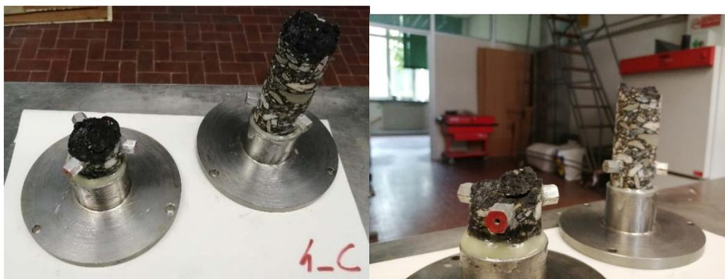
Figura 4.25 Provino 4C testato in stress control a  $T_{RP}=10^{\circ}C$
