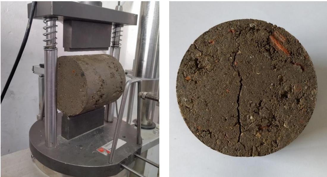
*Figure 10 : (a) ITS test machinery; (b) Crack in the sample after the test*
