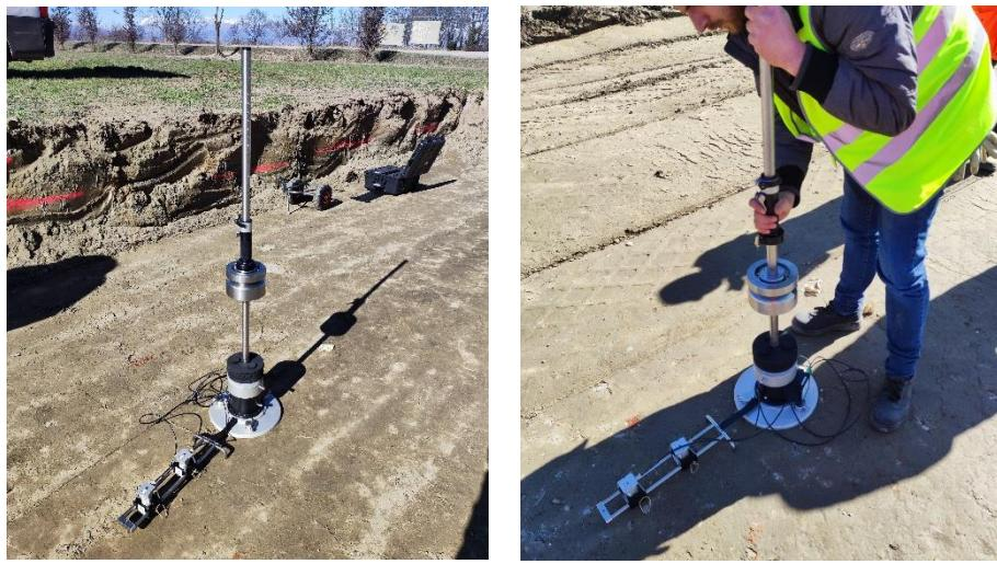
*Figure 25: LWD device with three geophones (a); Test execution on the subgrade (b).*
