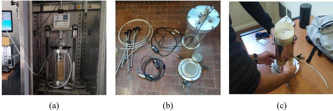
*Figure 6: (a) Nottingham asphalt tester (NAT) during the testing of a sample; (b) Equipment; (c) Sample preparation.*
