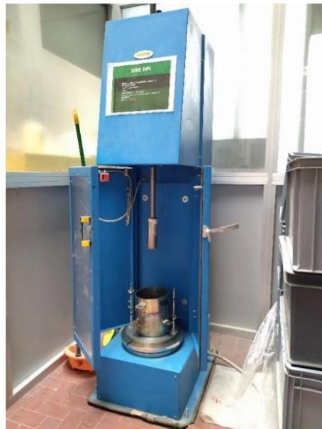
Figure 2: Proctor compaction machinery
