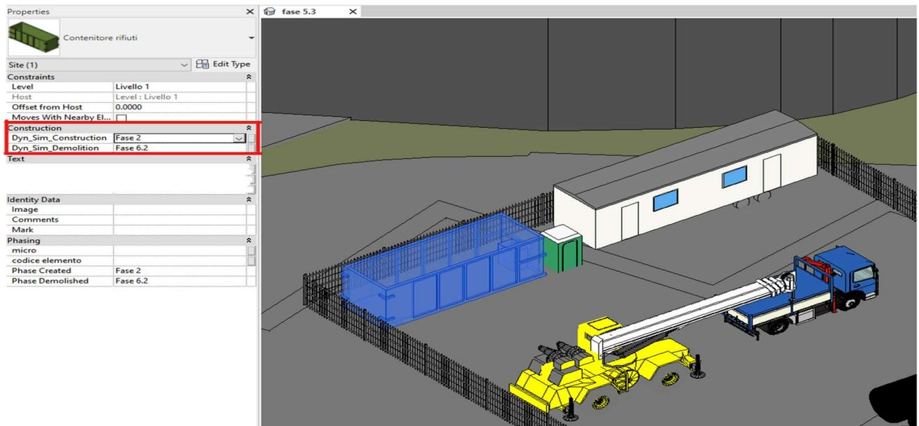
Figure 29 - Dynamo Simulation Parameter appearance on element properties
