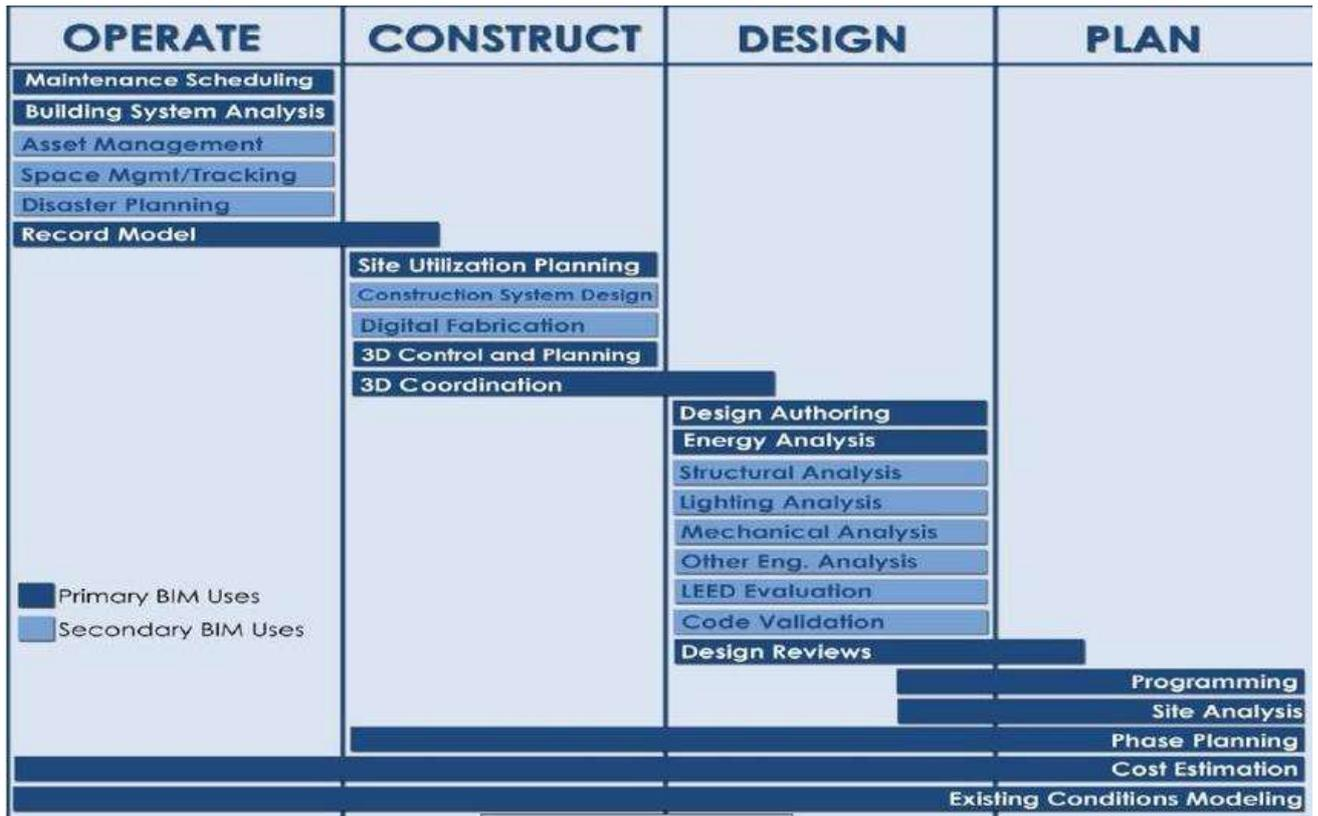
Figure 6 - BIM Uses Throughout a Building Lifecycle [107]
