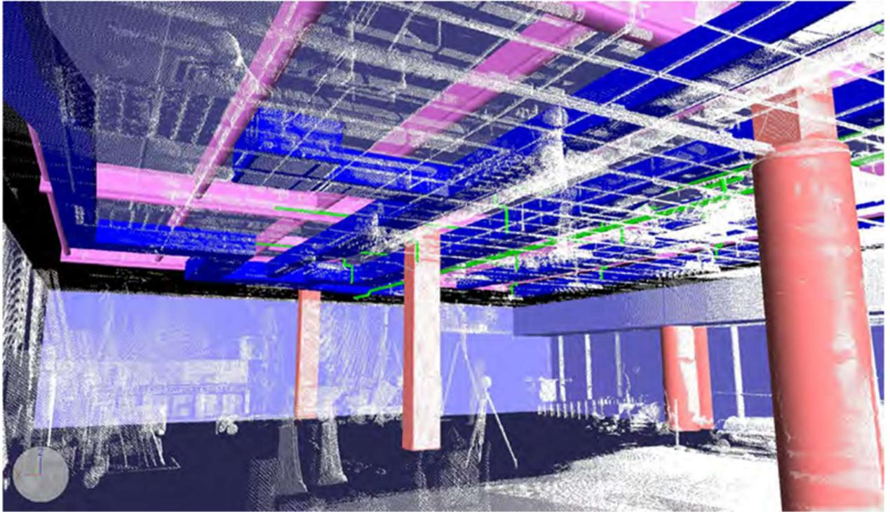
Figure 16 - Laser scan and BIM overlay[148]
