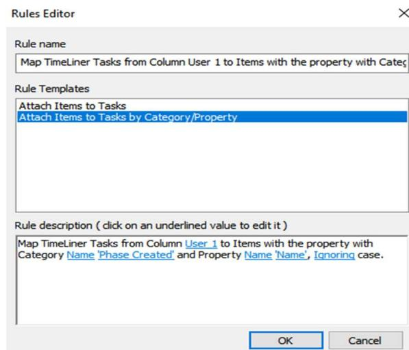
Figure 36 - Navisworks Auto attach using rules editor
