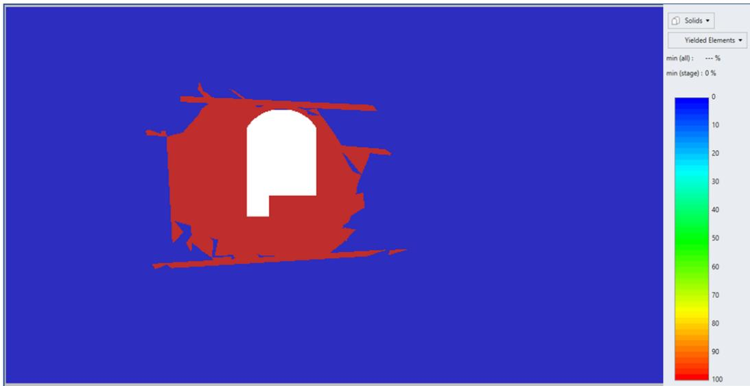
**Figure 6.22:** Auxiliary section Plastic zone in RS3 .
