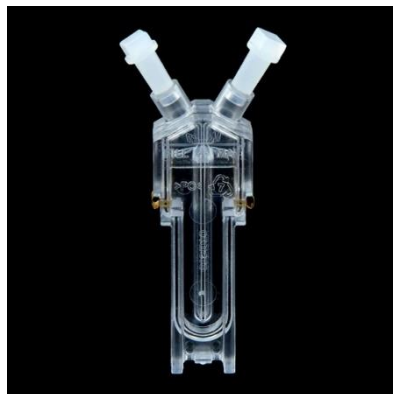
Figure 2.6: Picture of DTS1070 cuvette for Z-potential measurements.
