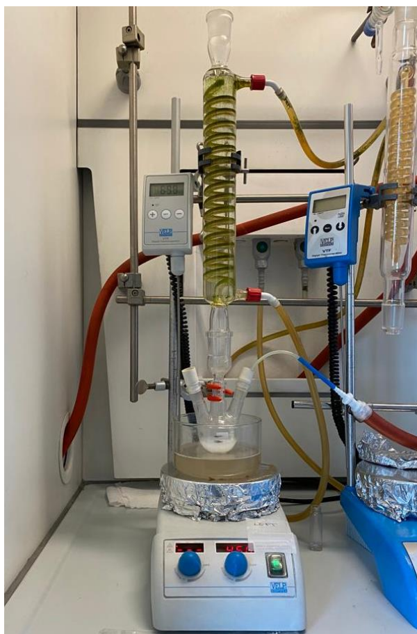
Figure 2.2: Setup for functionalization with amino groups
