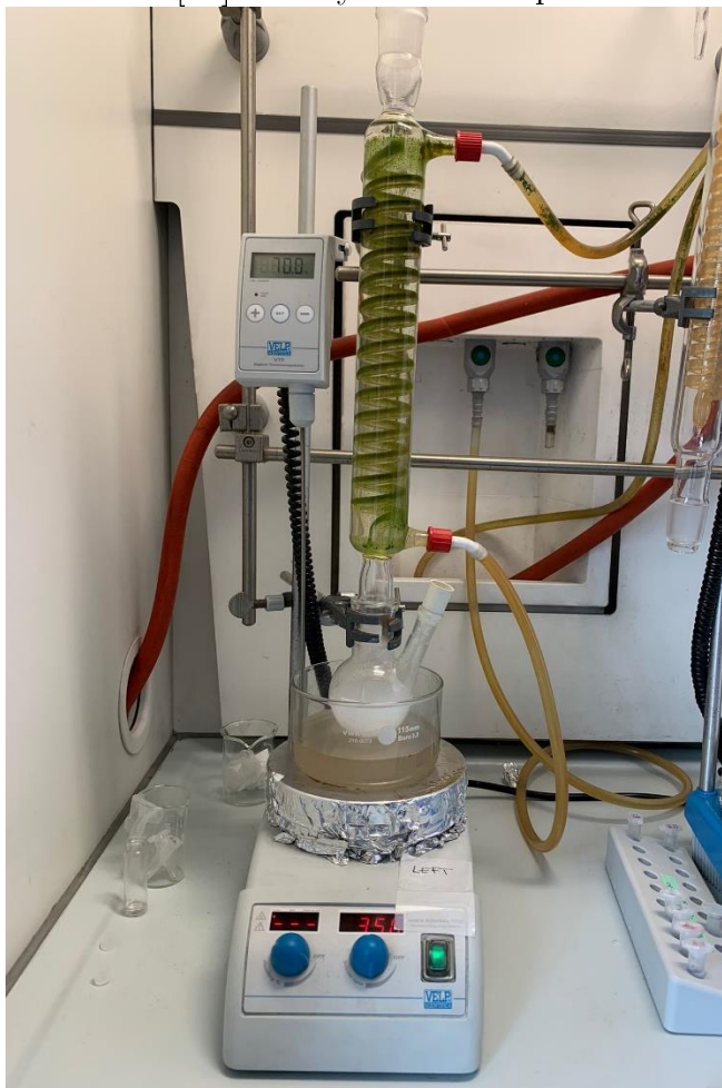
Figure 2.1: Setup for the synthesis of nanocrystals
