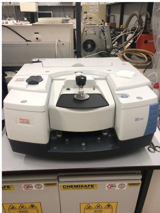
Figura 3.15: Nicolet Thermo Scientific iS50 FTIR Spectrometer.
