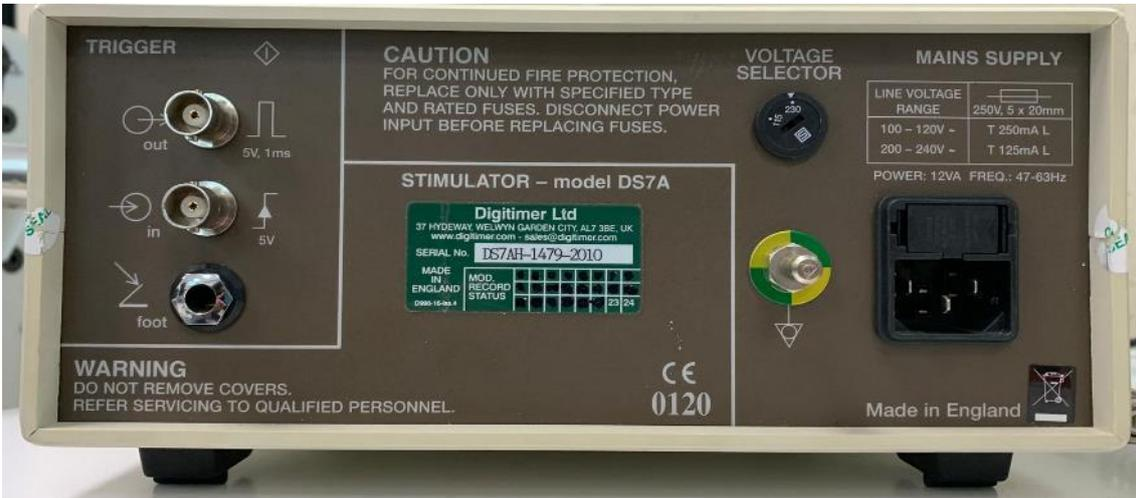
Figura 15. Pannello posteriore Digitimer DSA7H
