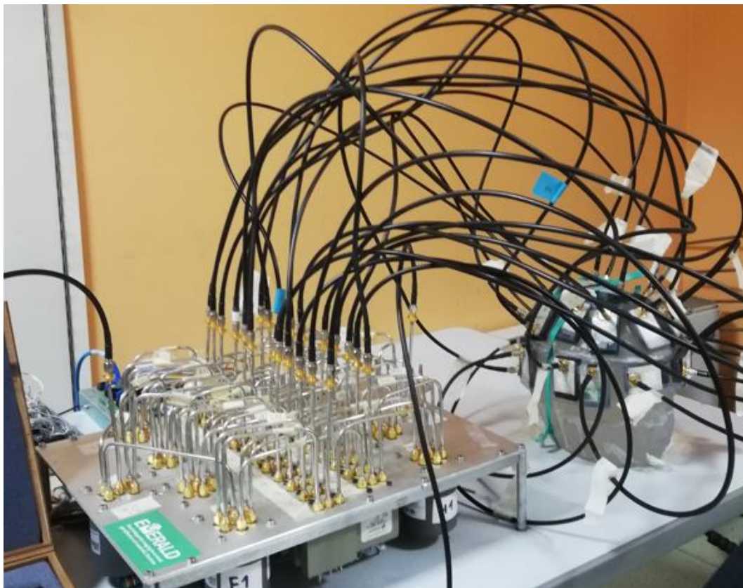
Figure 3.1 A Prototype Microwave System for 3D Brain Stroke Imaging developed at the DET of the Politecnico di Torino: the photo shows the helmet of antennas surrounding the 3D human head phantom and the switching matrix.
