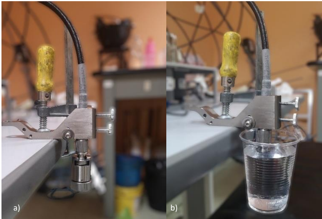
Figure 4.7. Coaxial probe calibration: a) short measurement, b) water measurement.
