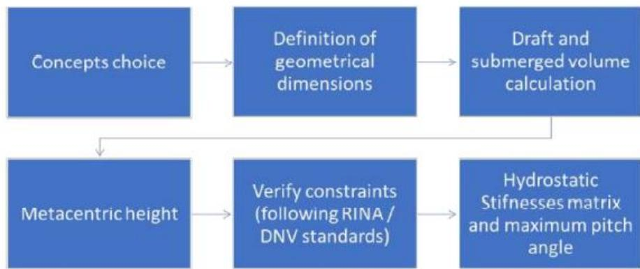
*Figure 4.2 Operating scheme of hydrostatic tool*
