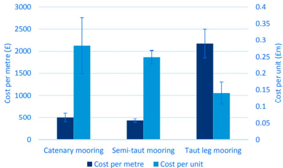
Figure 3.3 Moorings cost per meter and cost per unit [9]
