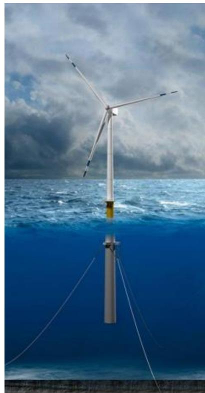
*Figure 2.5 Spar-buoy substructure concept*
