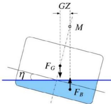
Figure 4.9 Floating structure in heeled condition
