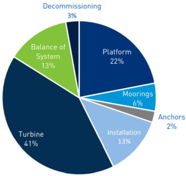
Figure 3.11 CAPEX breakdown for a commercial scale floating wind farm [9]
