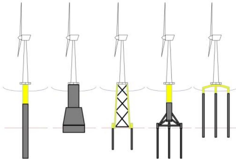
Figure 2.2 Types of bottom fixed concepts. From left to right: monopile, gravity-based, jacket, tripod and tripile [7].
