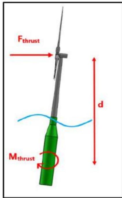
Figure 4.8 Thrust force and moment acting on a FOWT
