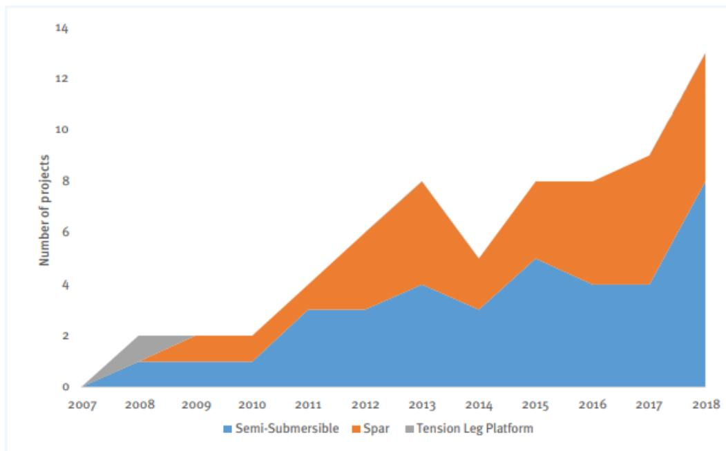
Figure 2.4 Cumulative number of European projects by structure concept type from 2007 to 2018 [8]
