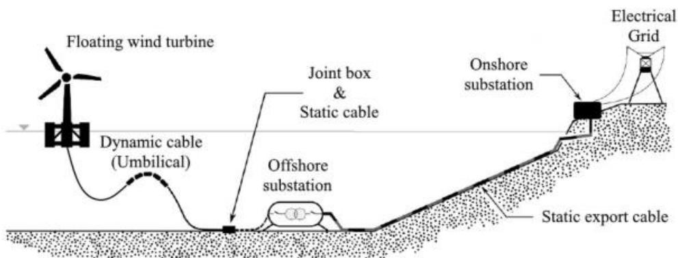
Figure 3.8 Power transmission system of a floating offshore wind [15]
