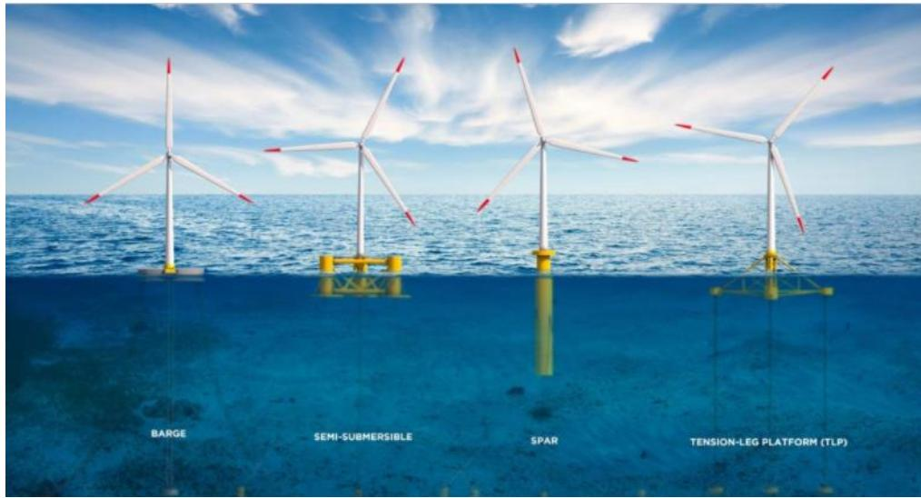
Figure 2.3 Floating structures classification
