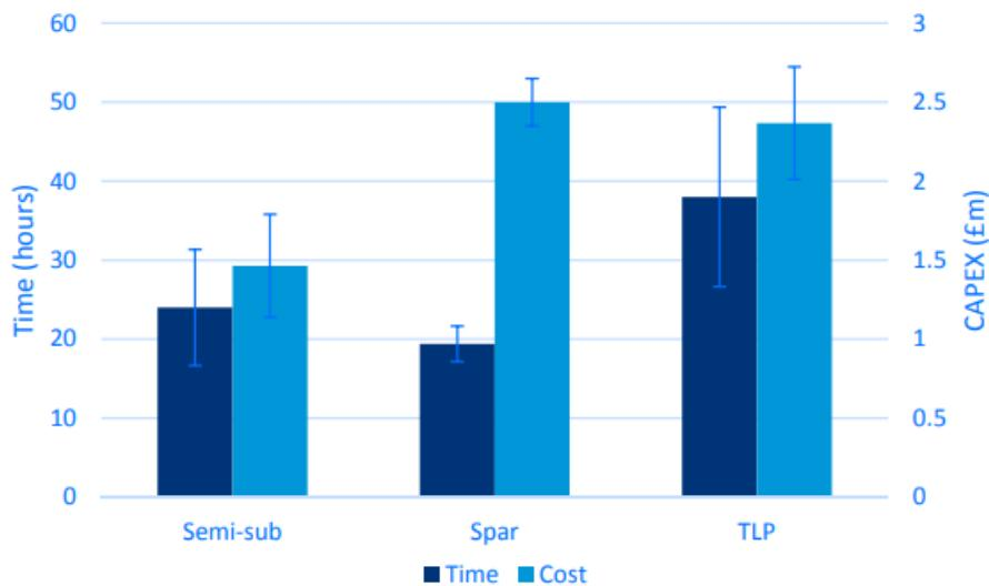
Figure 3.9 Installation time and cost for each type of floating platform [9]
