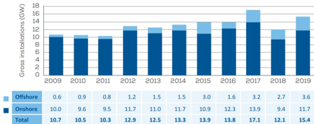
Figure 1.2 New annual onshore and offshore wind capacity installations in Europe [3]
