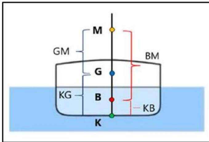
Figure 4.7 Representation of metacentric height
