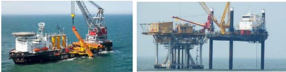
*Figure 3.10 Heavy Lift Vessel (left) and Jack-Up Rig (right).*
