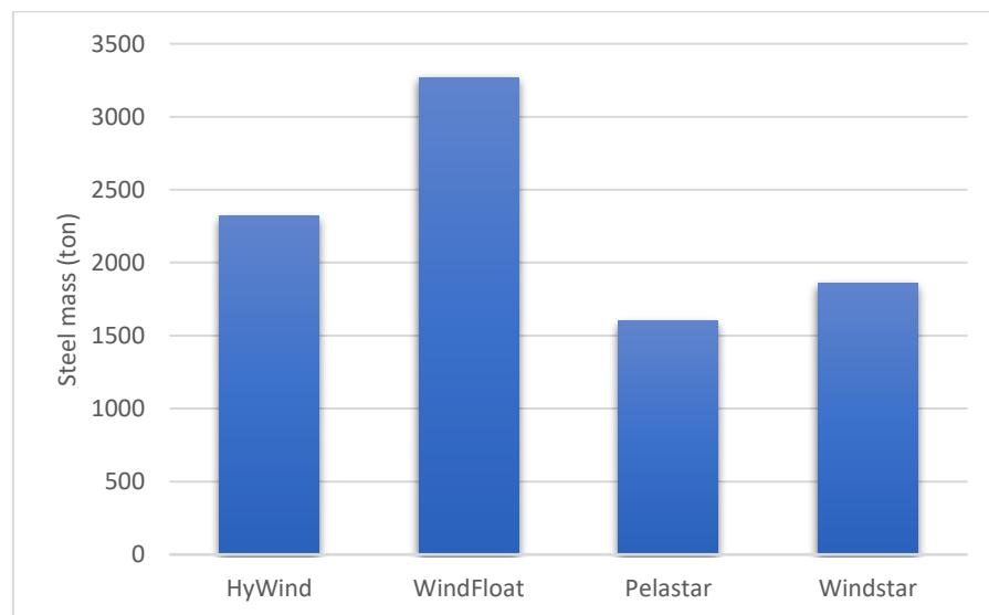
*Figure 5.11 Comparison of the structure deign based on the steel mass*
