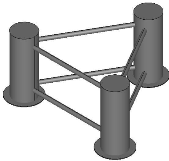
*Figure 4.4 WindFloat concept represantation*
