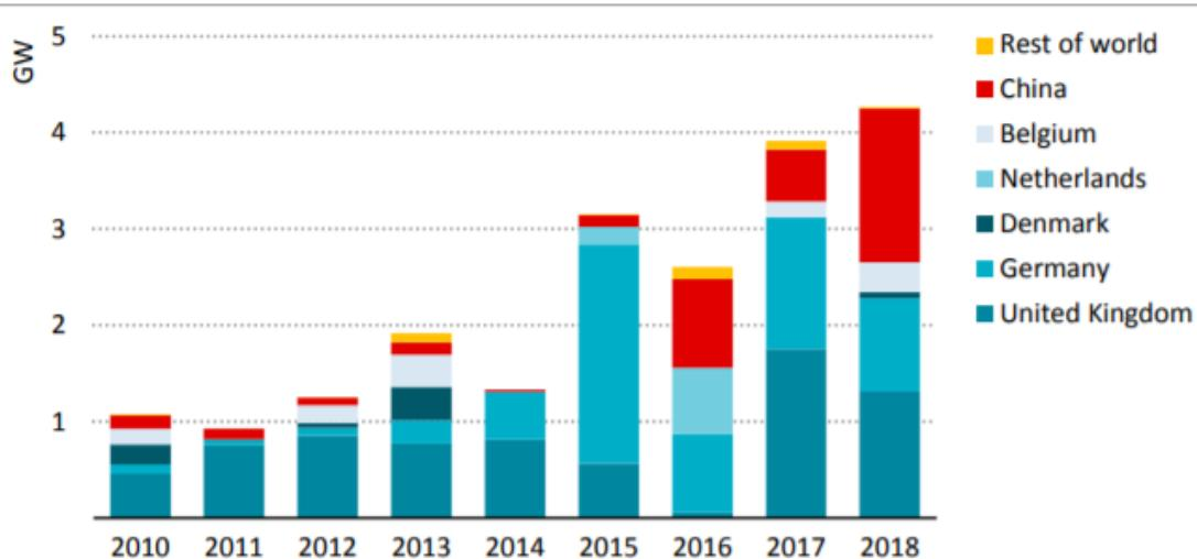
Figure 1.1 Annual increase in offshore wind capacity by region, 2010-2018 [1]
