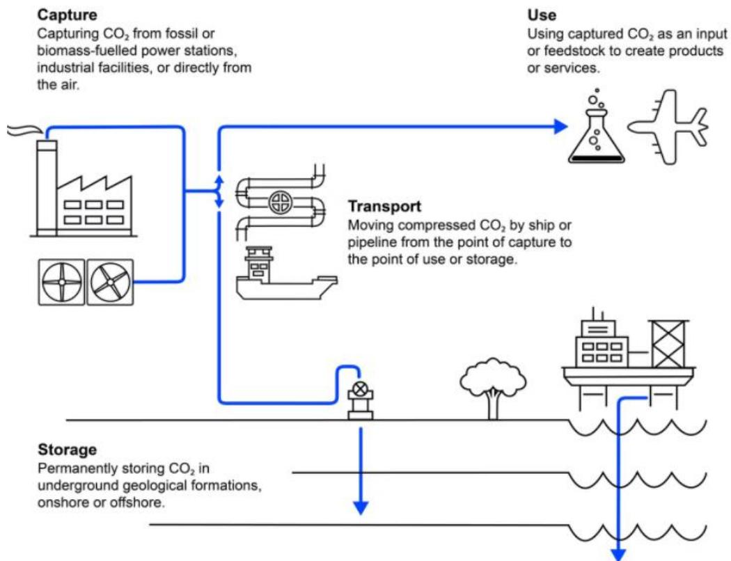
Figure 23 Carbon Capture Utilisation and Storage process diagram (IEA, 2021).
