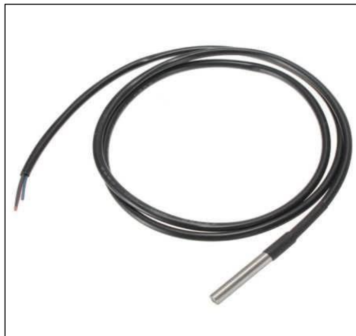
Figure 4-7 Chamber's PT100s for temperature control
