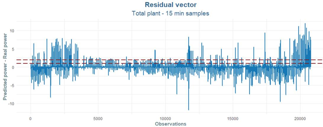
Figure 53: 15-minutes residuals and comparison with limits for the total plant.
