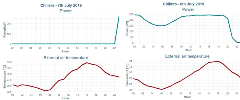
Figure 33: Power curve of the chiller unit during 7th and 8th July 2019.
