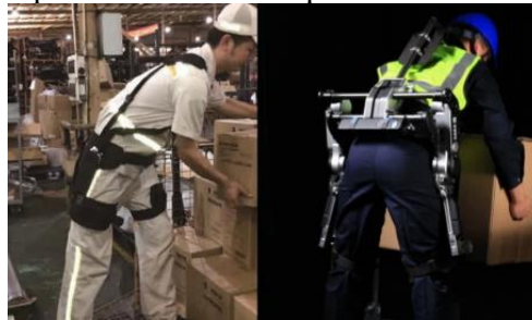
Fig. 19 A passive lower back exoskeleton and an active lower back exoskeleton
