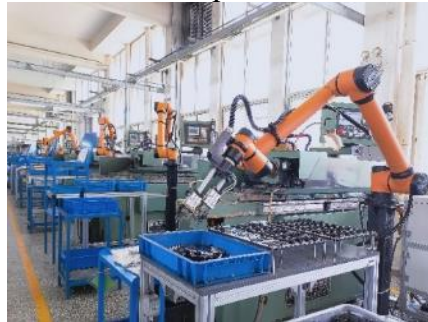
Fig. 10 A collaborative robot is feeding the lathe
