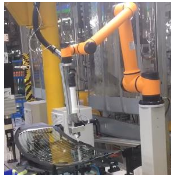
Fig. 12 A collaborative robot is glutting the windshield
