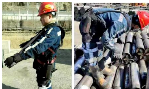
Fig. 22 the exoskeleton used in the mining industry
