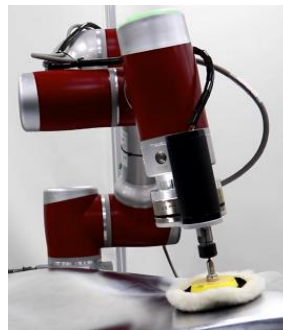
Fig. 13 A collaborative robot is polishing parts, JAKA
