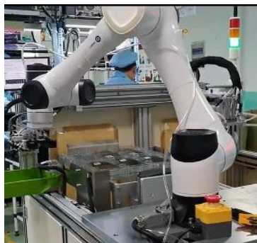
Fig. 9 A collaborative robot is placing a chip on a conveyor, DOBOT
