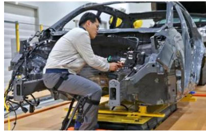
Fig. 21 lower limb exoskeleton chair, Hyundai
