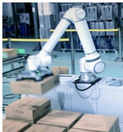
Fig. 11 A collaborative robot is stacking boxes, ELIBOT
