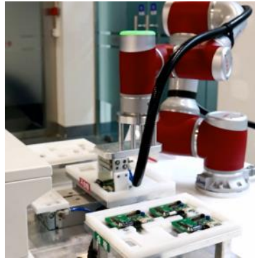
Fig. 14 A collaborative robot is doing a quality check with an X-ray detector
