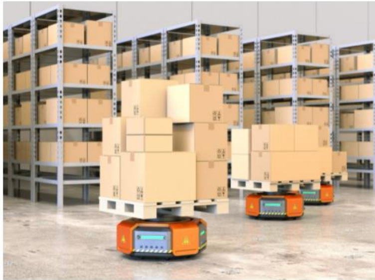
Figure 1.7 Example of automated robotic loader (Robotic Technician Training,2017).
