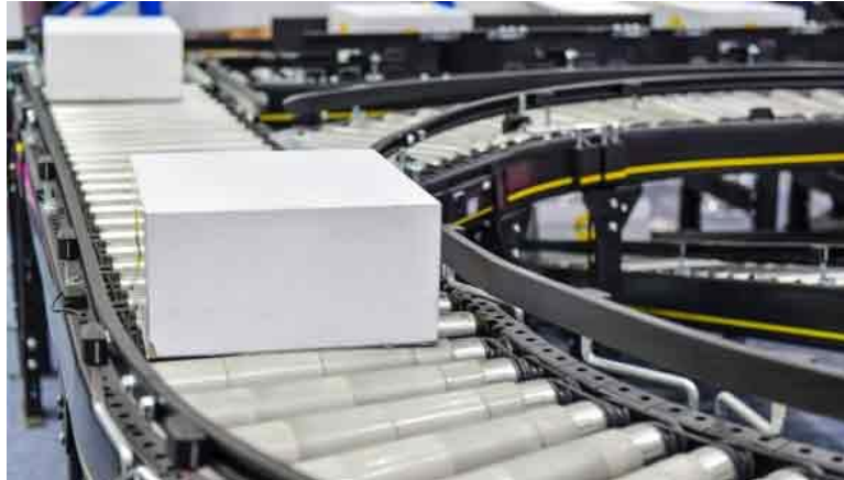
Figure 1.9 Example of fixed automation: conveyors (Engineering Review, 2017)
