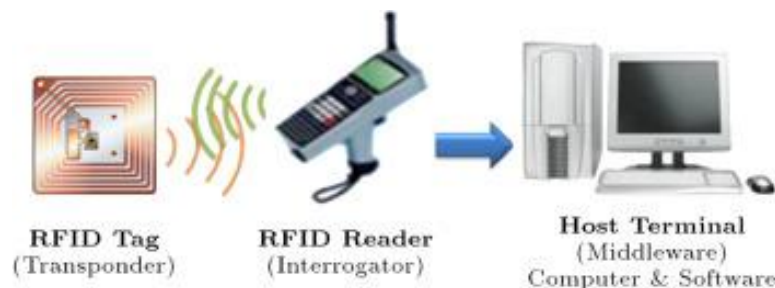
Figure 3.2 RFID system components (Javad, 2012)
