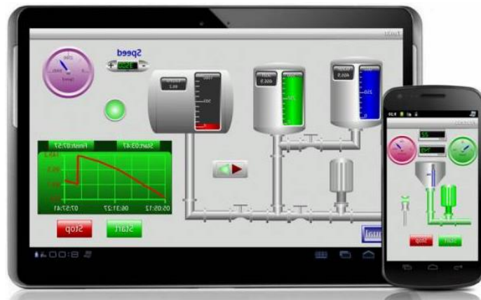
Figure 1.15 SCADA software interface for smartphone and tablet (automationworld.com [14])
