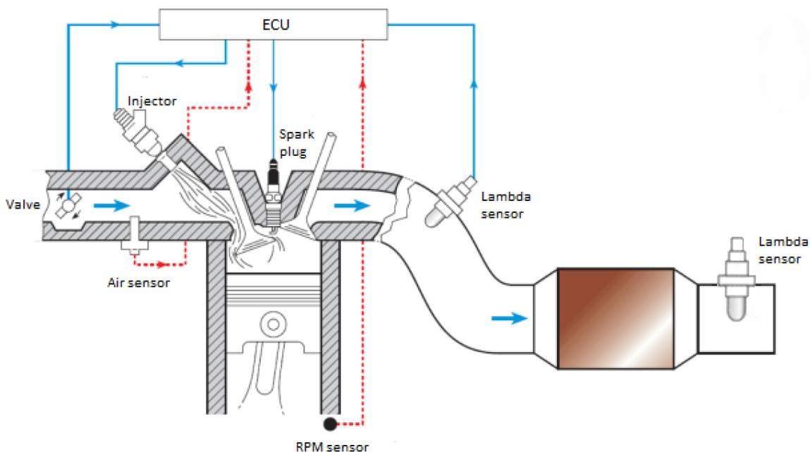
Figure 9: Closed loop control system for air / fuel ratio
