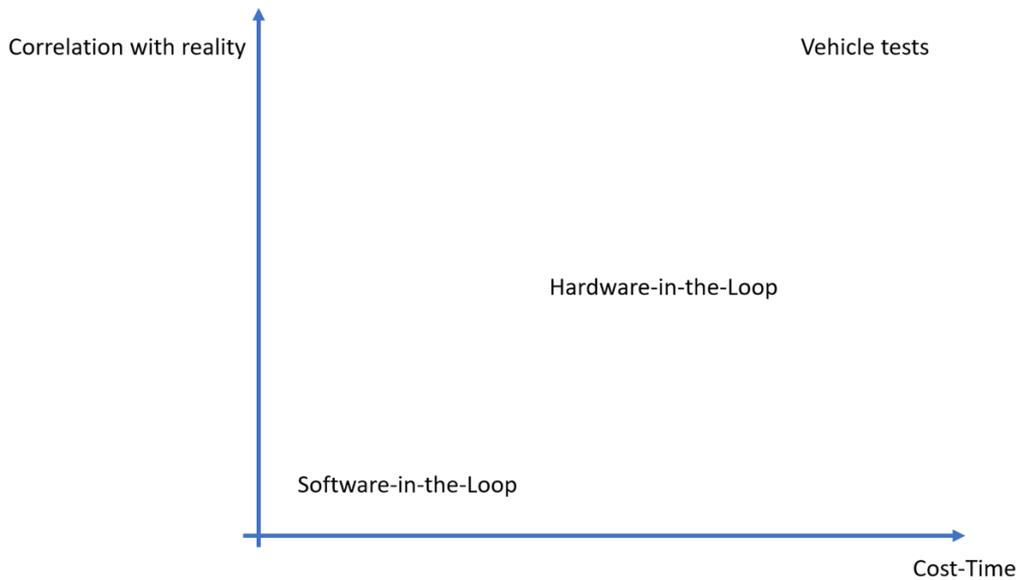
Figure 3: Scheme for correlation with reality of the different approaches
