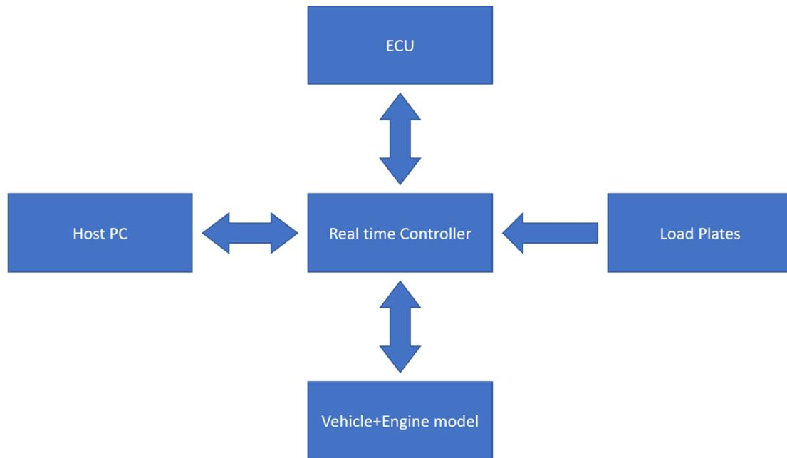
*Figure 6: Hardware-in-the-Loop scheme*
