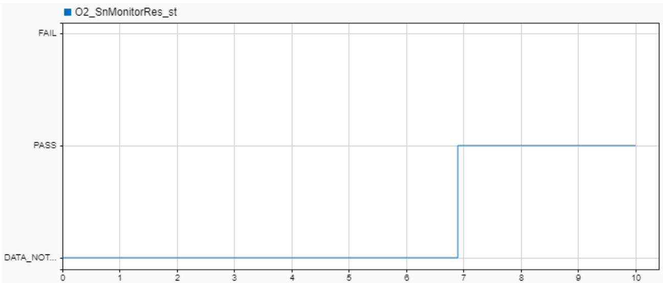
Figure 32: Result of test in SiL for the Oxygen Sensor Monitor
