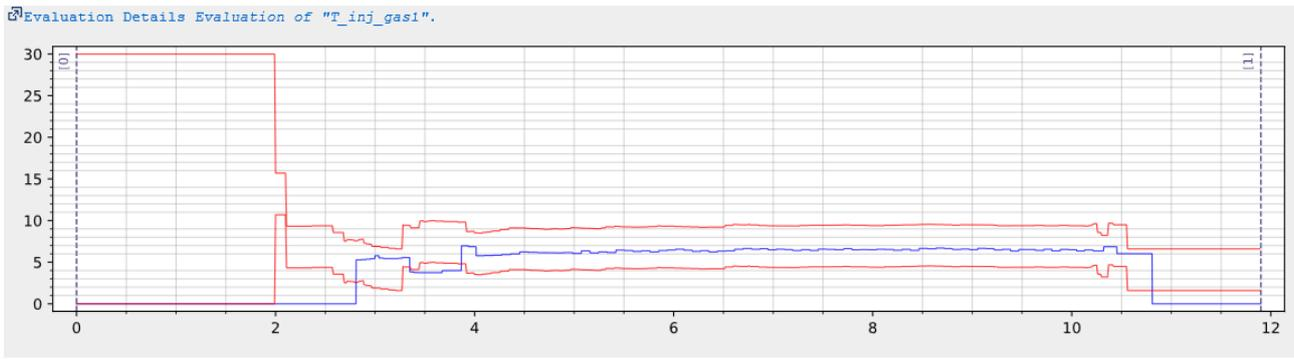
*Figure 27: Result for the dynamic test in HiL*
