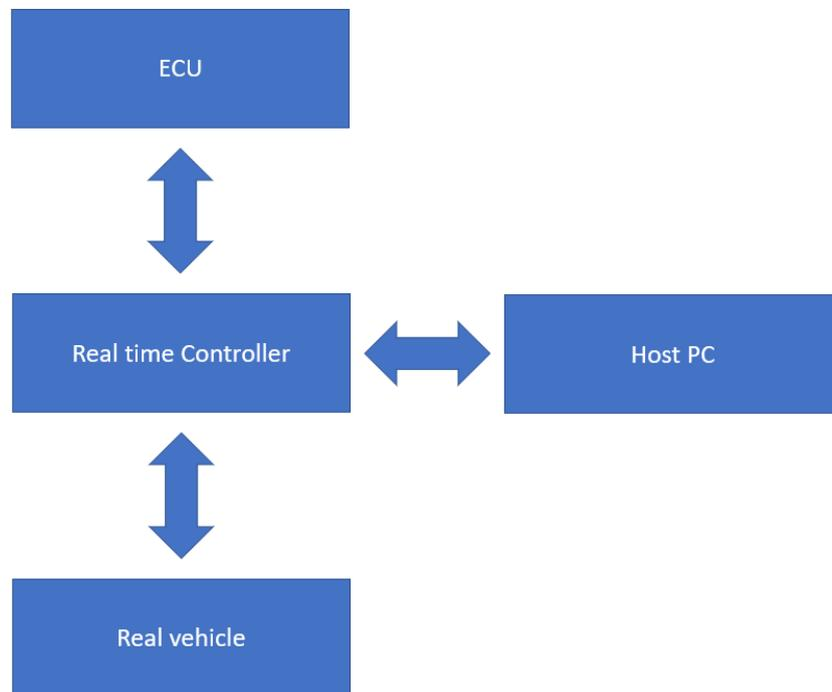
*Figure 8: Vehicle test scheme*
