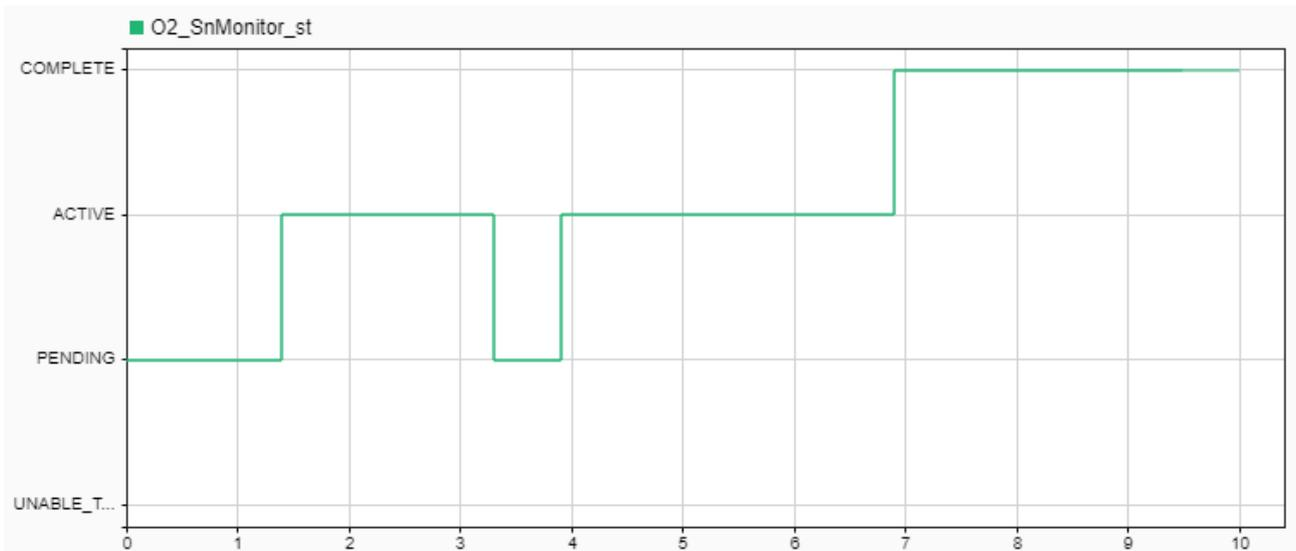
Figure 31: Status of test in SiL for the Oxygen Sensor Monitor
