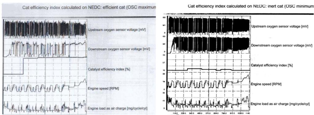
Figure 12: Catalyst efficiency monitored by oxygen sensors
