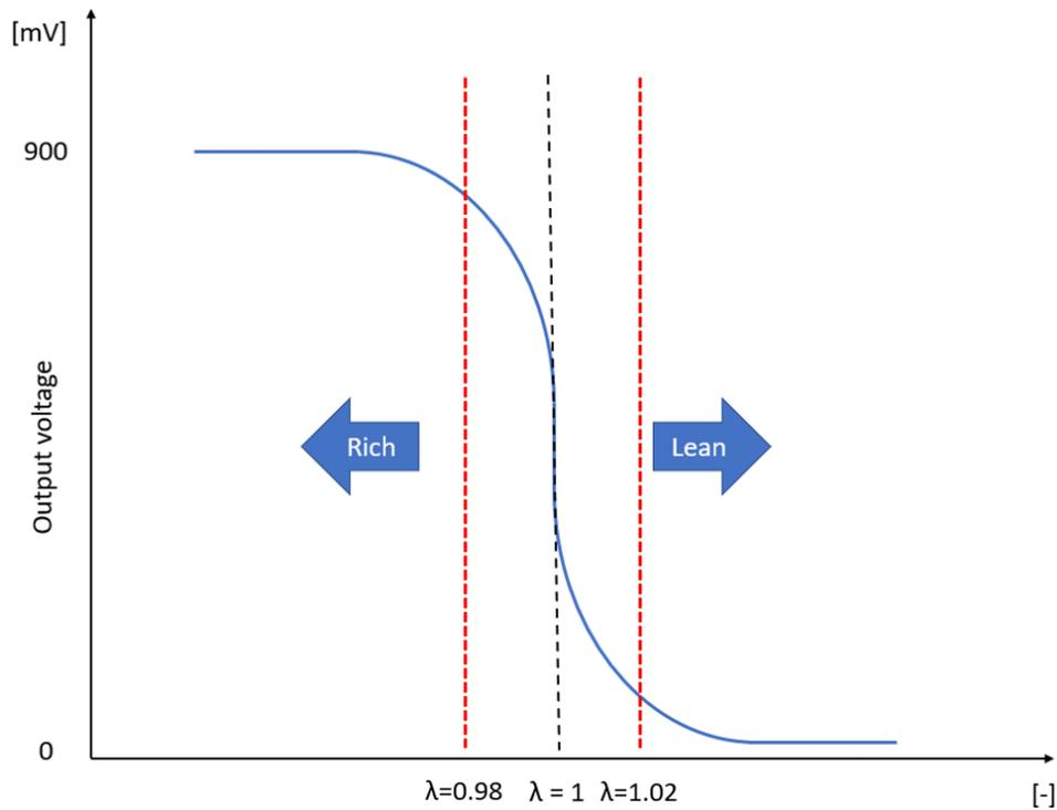
Figure 11: Typical output voltage of a lambda sensor
