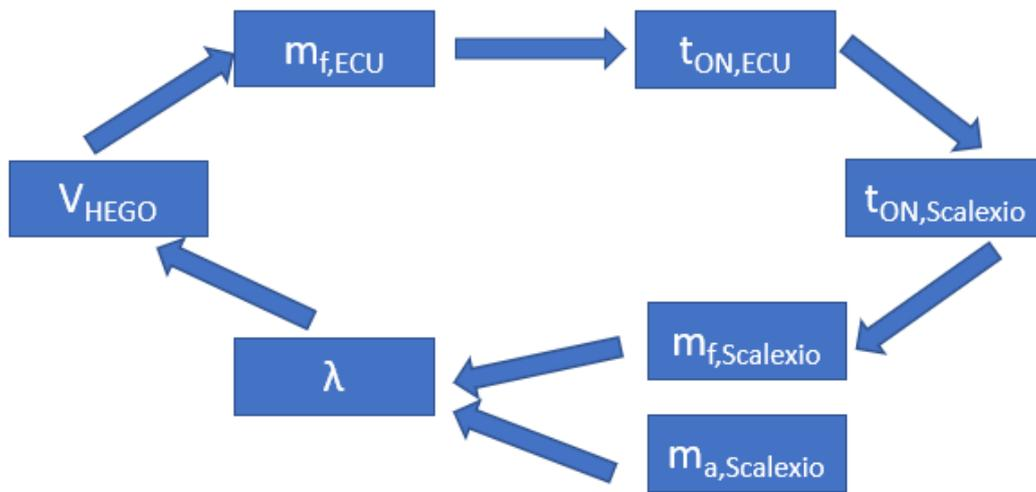
Figure 10: Scheme of closed loop control system for air /fuel ratio
