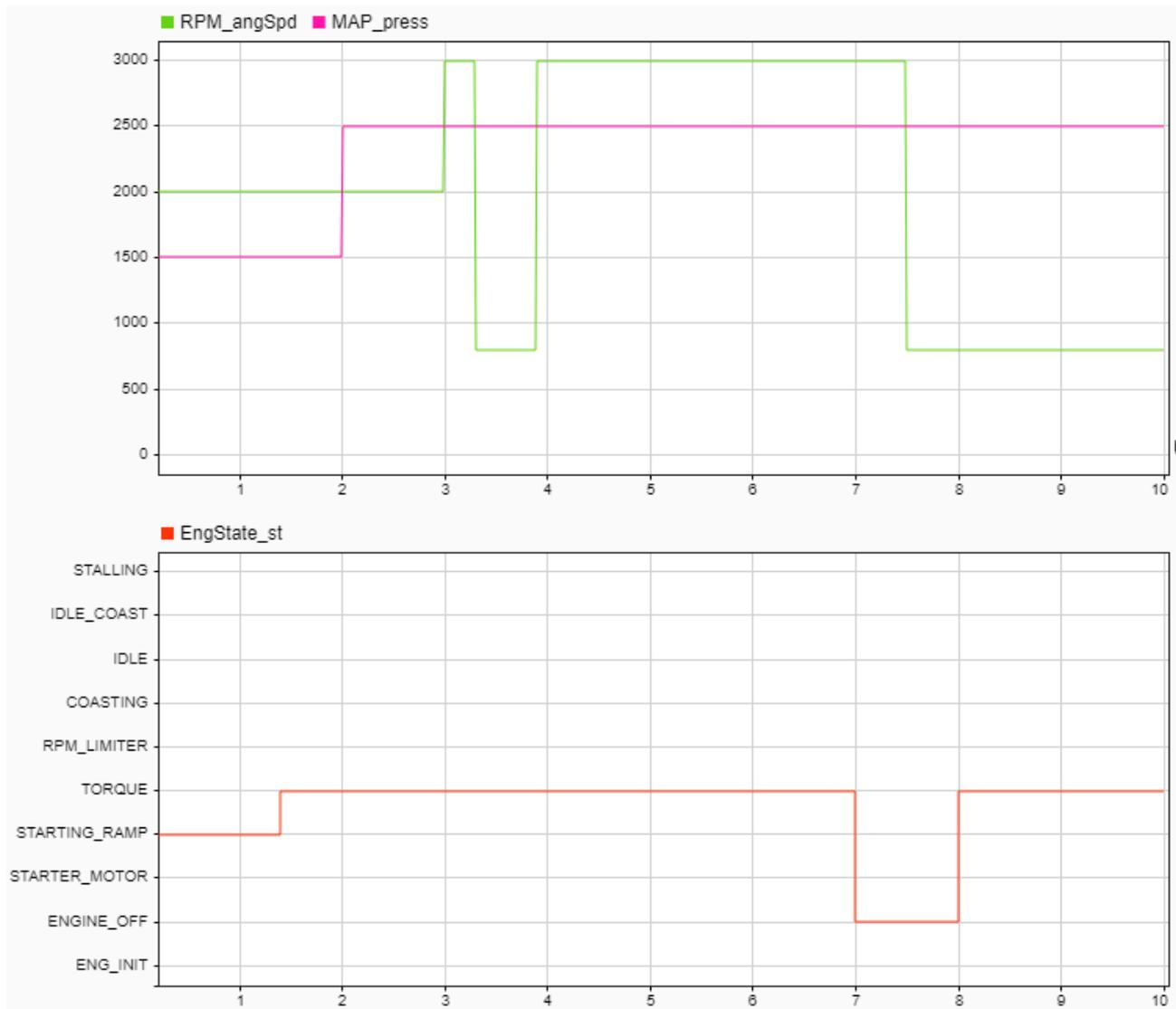
Figure 30: Points of operation for the test in SiL
