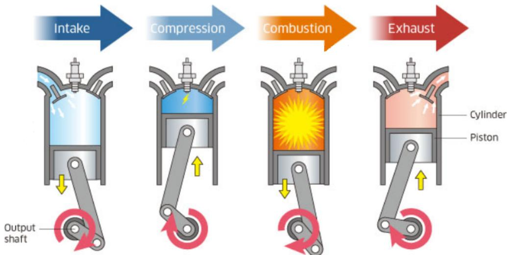
Figure 19: Phases of a ICE with 4 strokes
