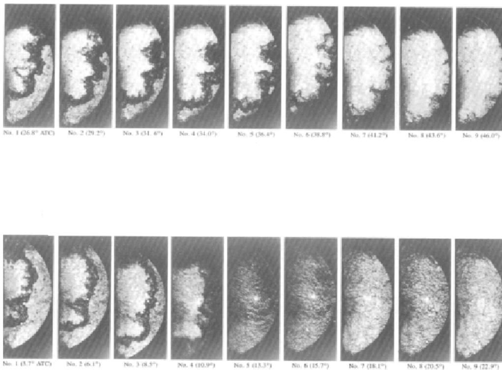
Figure 20: Photographic sets of the combustion's evolution
