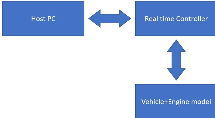
Figure 4: Software-in-the-Loop scheme
