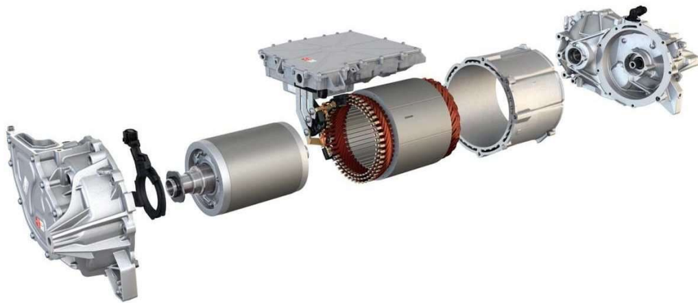
Figure 7.5 - Automotive Electric Motor Exploded View
