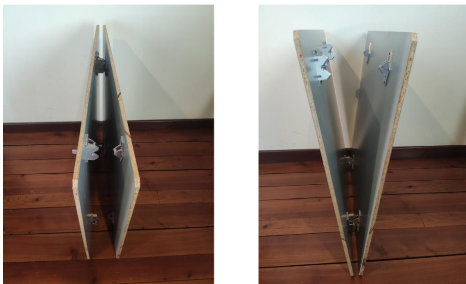
Figure 119 Coupler test 1:3 scale module – maximum misalignment angle
