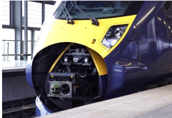
Figure 100 High-speed train with exposed coupler system
