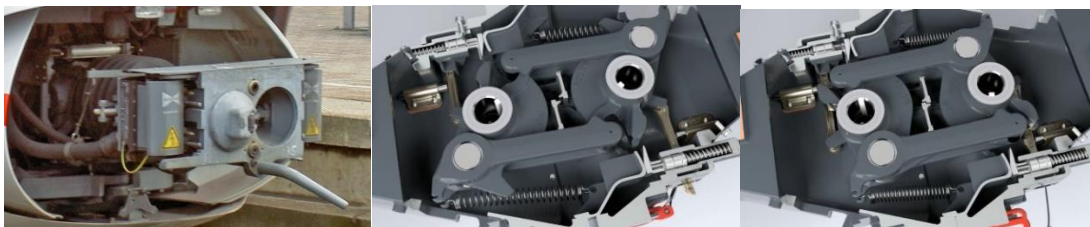
Figure 102 Scharfenberg coupler open and closed position
