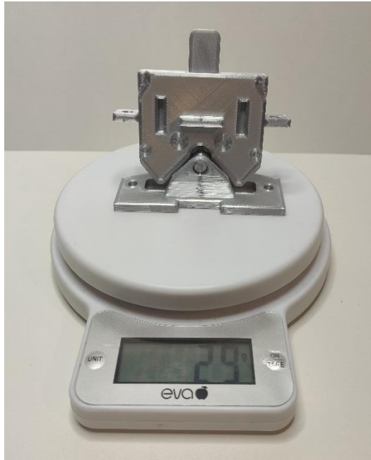
Figure 114 Experiment closing force coupler claws
