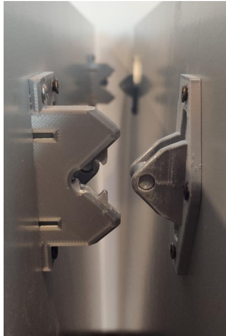
Figure 118 Coupler test 1:3 scale module - engaging phase
