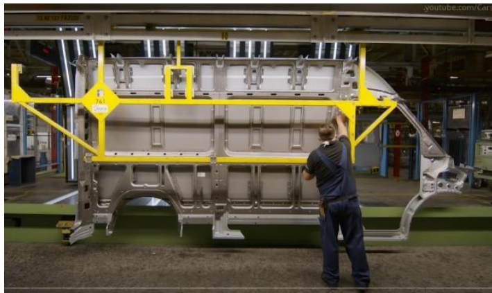
Figure 73 Side panel structure of a Mercedes-Benz Sprinter
