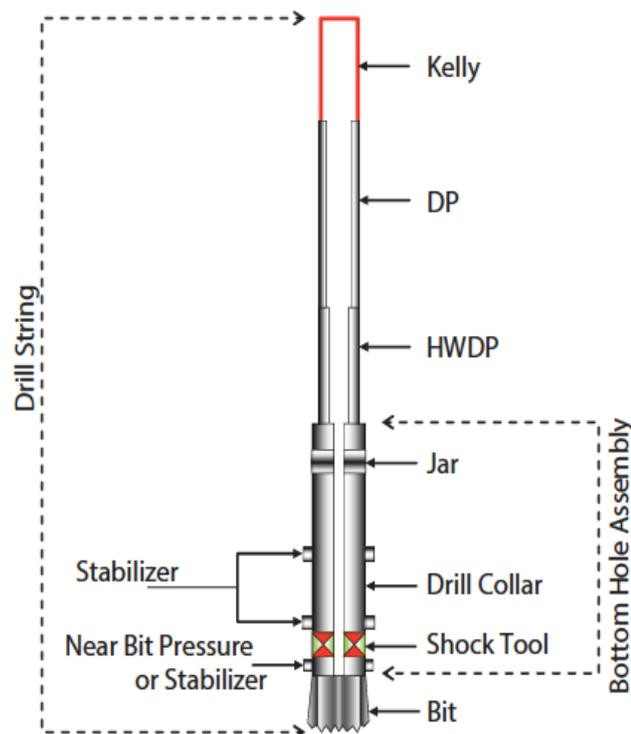
Figure 1.1 Drill string components
