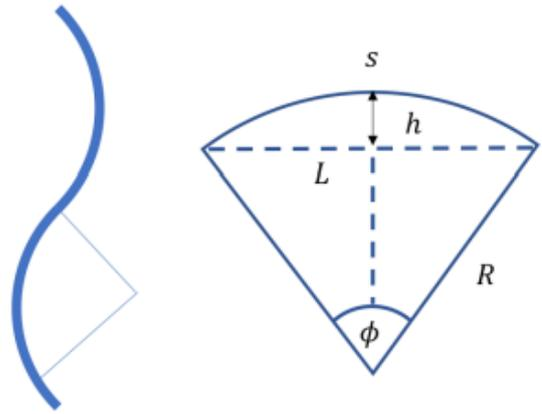
**Figure 4.6 Demonstrates drill string deformed shape as result of lateral vibration (Larsen 2014)**
