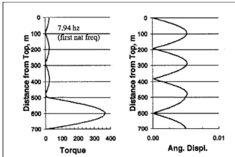
**Figure 4.4 Torsional resonance**
