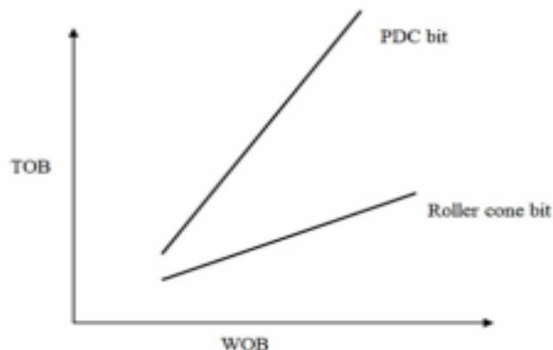
**Figure 5.1 Difference between roller cone and PDC bits**
