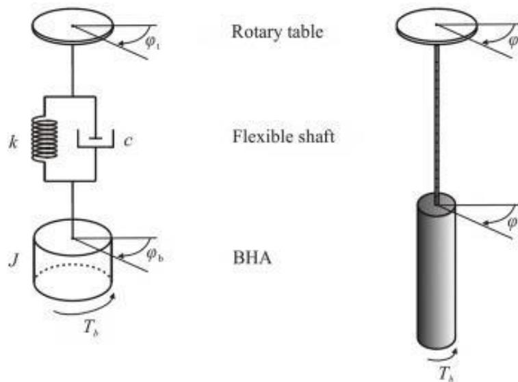
**Figure 6.3 Continuous equivalent model provided by using FEM**
