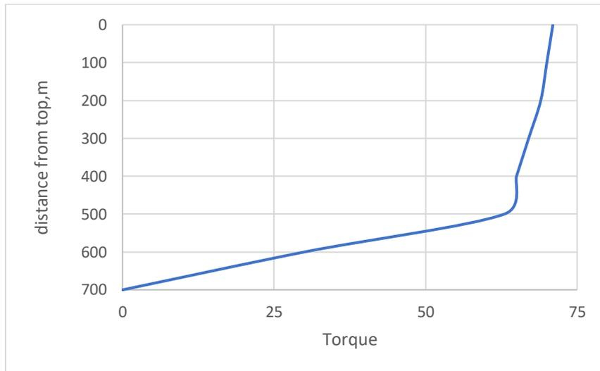
**Figure 4.3 Drill string torque profile during stick/slip**
