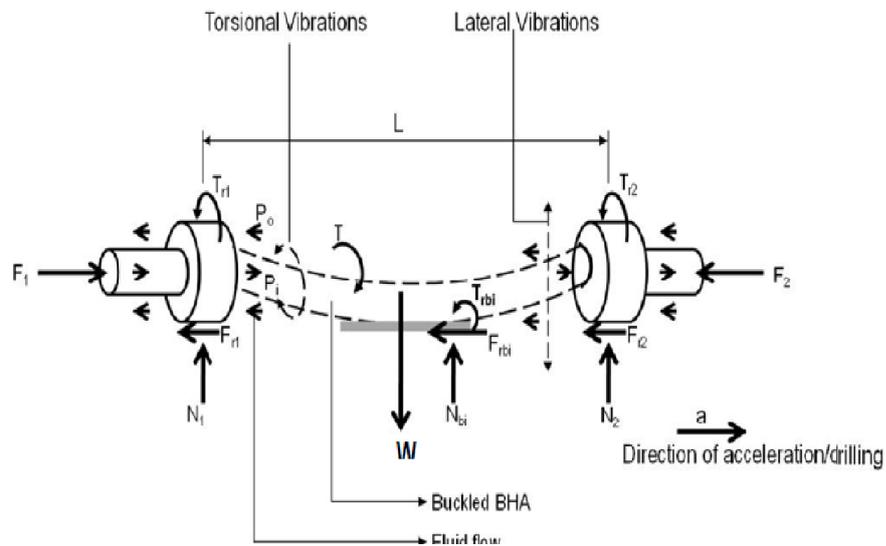
**Figure 6.2 Analytical model representation by horizontal stick**
