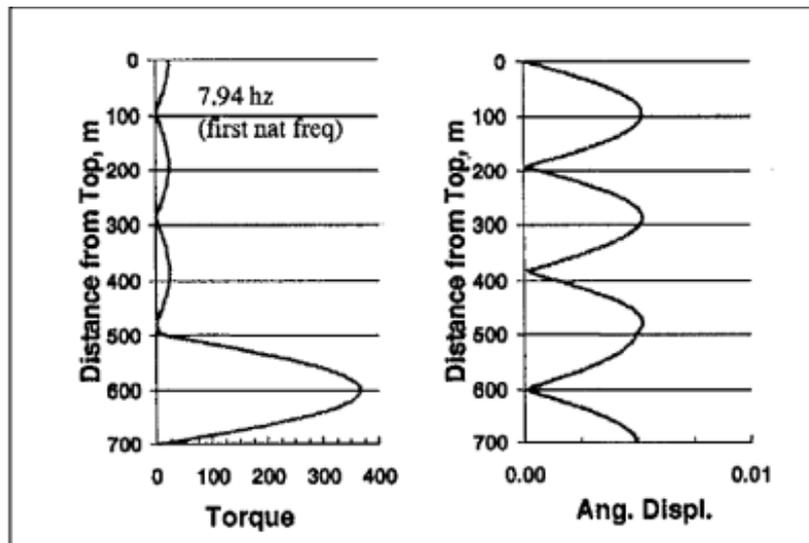
**Figure 4.4 Torsional resonance**
