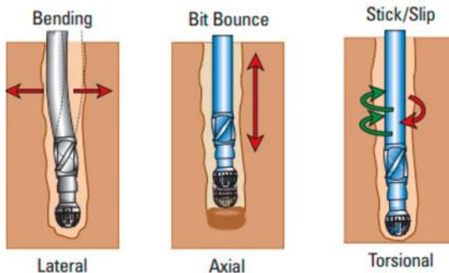
**Figure 8.1 Representation of vibration types**
