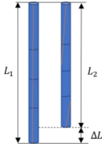
**Figure 4.7 Twist of pipe which causes shortening (red line presents fiber along the pipe)**
