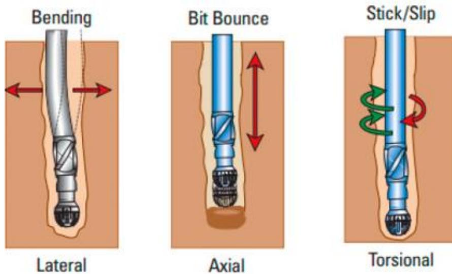
**Figure 8.1 Representation of vibration types**
