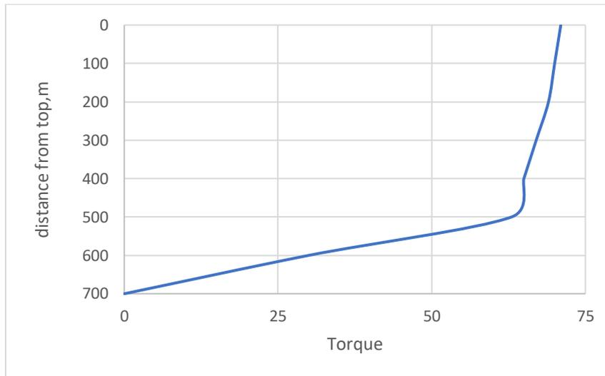
**Figure 4.3 Drill string torque profile during stick/slip**
