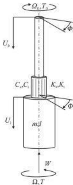
**Figure 6.1 Drill string with lumped mass representing**
