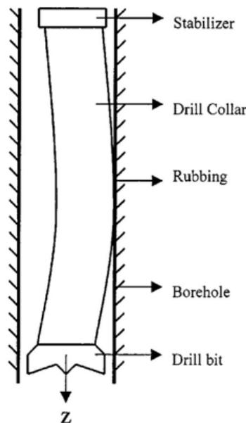
**Figure 4.1 Bending of drilling collar**
