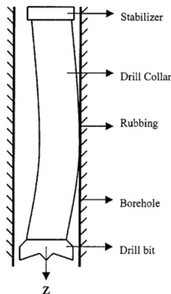
**Figure 4.1 Bending of drilling collar**
